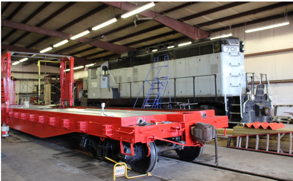
The flatcar in the foreground was being converted into an open-air car. In the background is number 701 a GP 10, ex ICG 8307.
