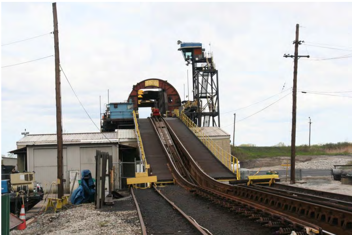
Above and below are two views of “No. 4 Barrel” that dumps the coal from the loaded coal cars onto the conveyor belt to feed the flood loader.
