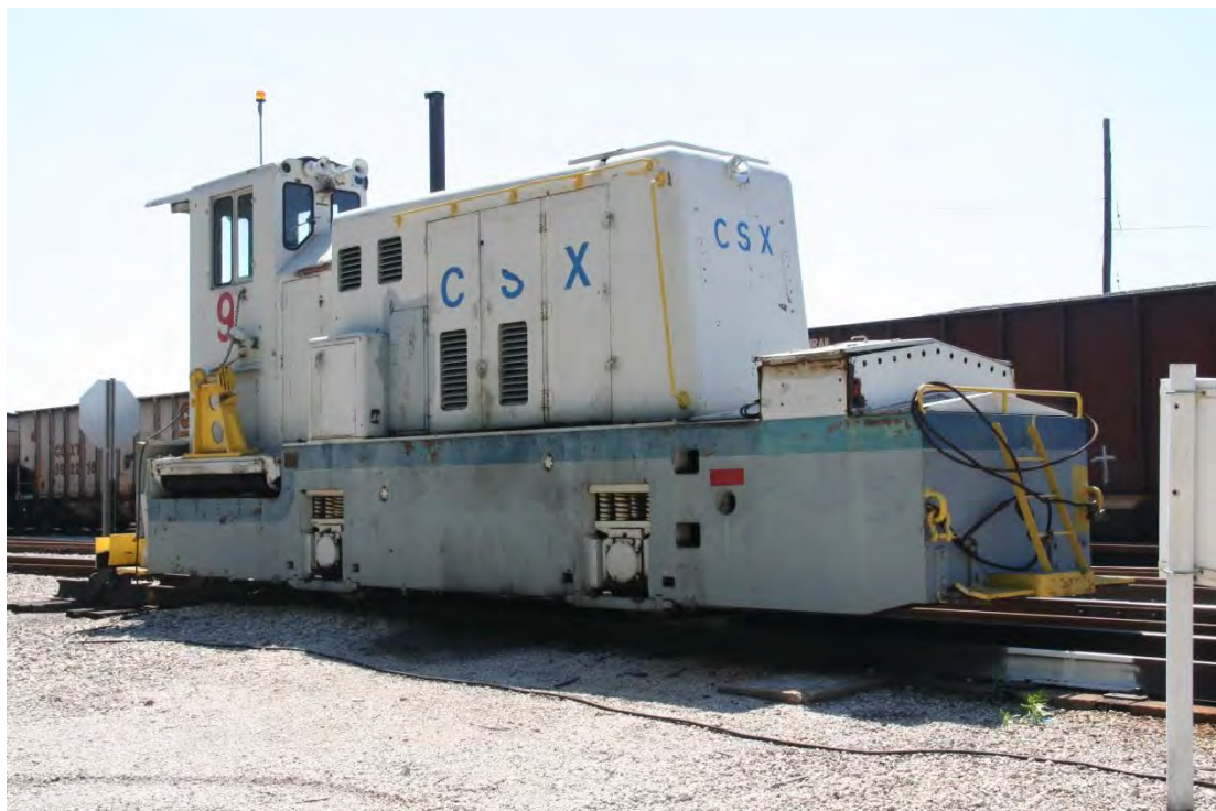
Above and below are views of two of the GE 55-tonners used to move the coal cars to the rotary dumper.
