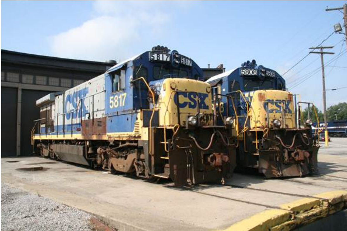
CSXT 5817 and CSXT 5809, both B36-7s, are used as spare part sources to keep TTI's other ex-CSXT locomotives running.
