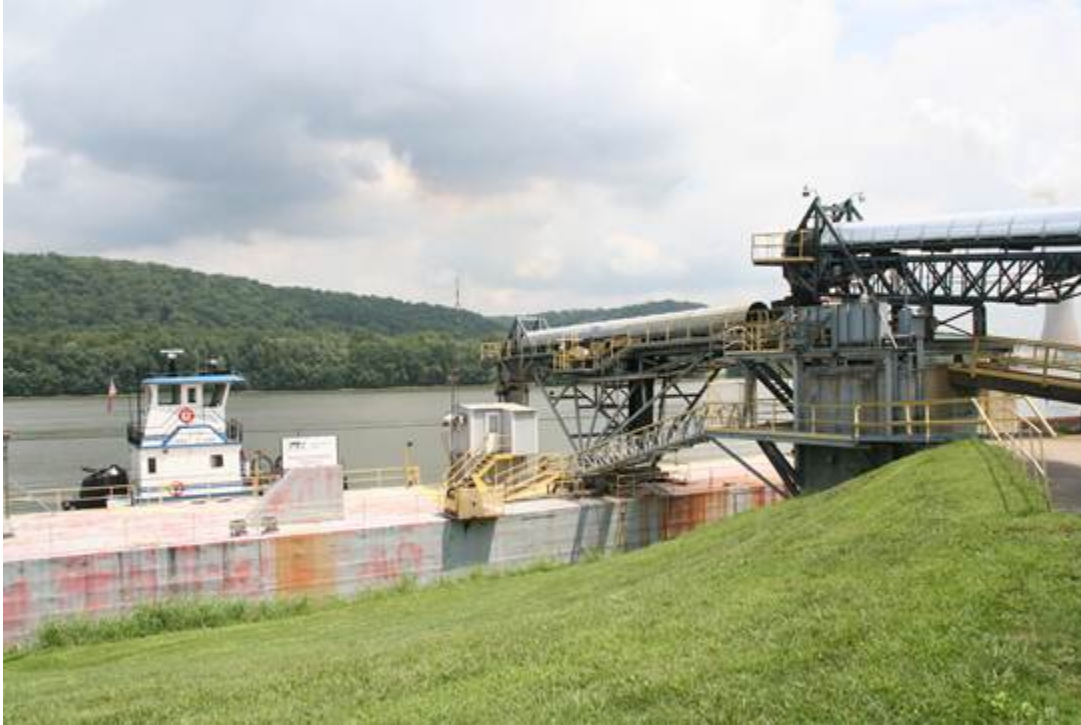
TTInc barge flood loader at Maysville. The facility delivers coal to power plants along the north shore of the Ohio River, which do not have rail access. A cooling tower of such a plant can be seen right center under the conveyor belt.
