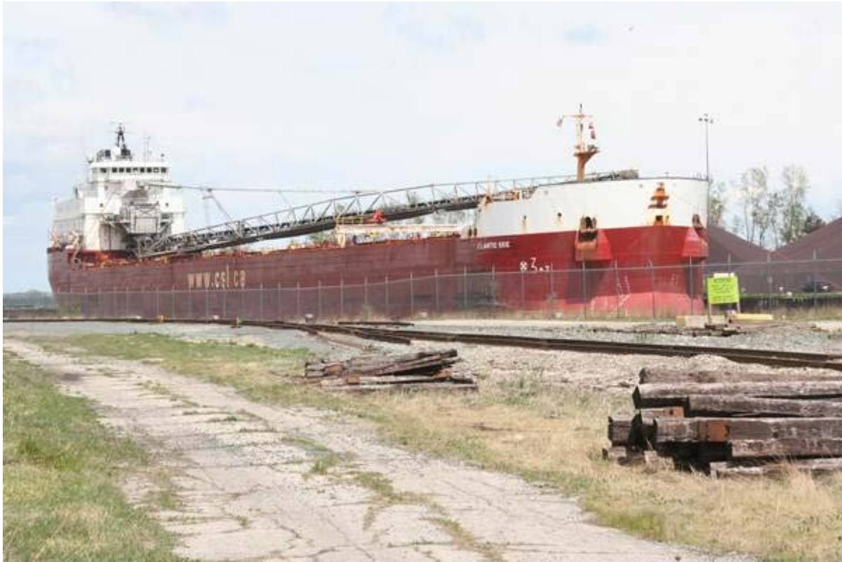
Atlantic Erie at Slip No. 1 off-loading taconite via her off-loading equipment
