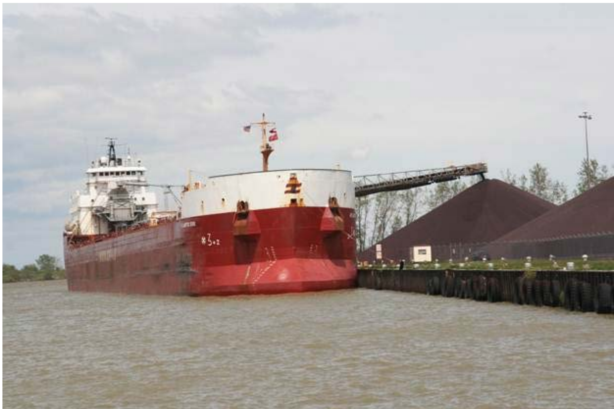
Atlantic Erie at Slip No. 1 off-loading taconite via her off-loading equipment
