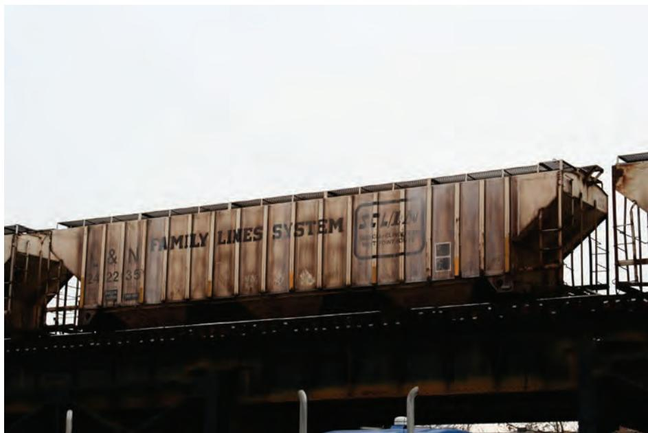
L&N 242235 was built for the L&N by Pullman Standard. She is seen here in July 2013 coming down into Queensgate Yard from the C&O Bridge approach. She is 60 feet long, 10 feet 8 inches wide, and 15 feet 1 inch tall. Internally she provides 4,750 cubic feet of cargo space within to carry 202,300 pounds of product.
