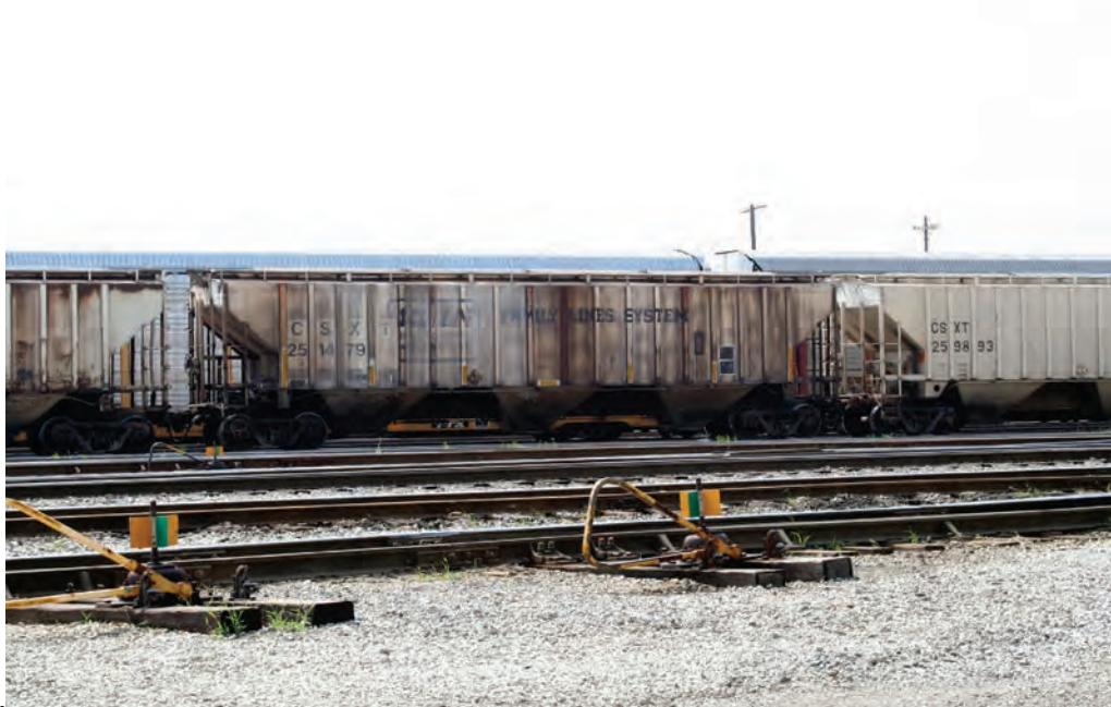
**CSXT 251479**, still in Family Line paint, is the former SCL 242020. Seen here at Columbus, Ohio, in 2011, she is 59 feet 11 inches long, 10 feet 7 inches wide, and 15 feet tall. With a cubic capacity of 4,759 cubic feet, she can carry 201,000 pounds of goods.
