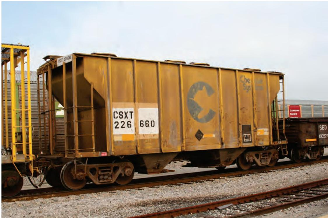
**CSXT 226660**, seen at Indianapolis, Indiana, in 2012, is a former Chessie System B&O car built by Pullman Standard. She has four loading hatches and two gravity flow discharge hatches. She is 38 feet 10 inches long, 10 feet 7 inches wide, and 14 feet 10 inches high. She can carry 206,000 pounds within her 2,700 cubic feet interior.
