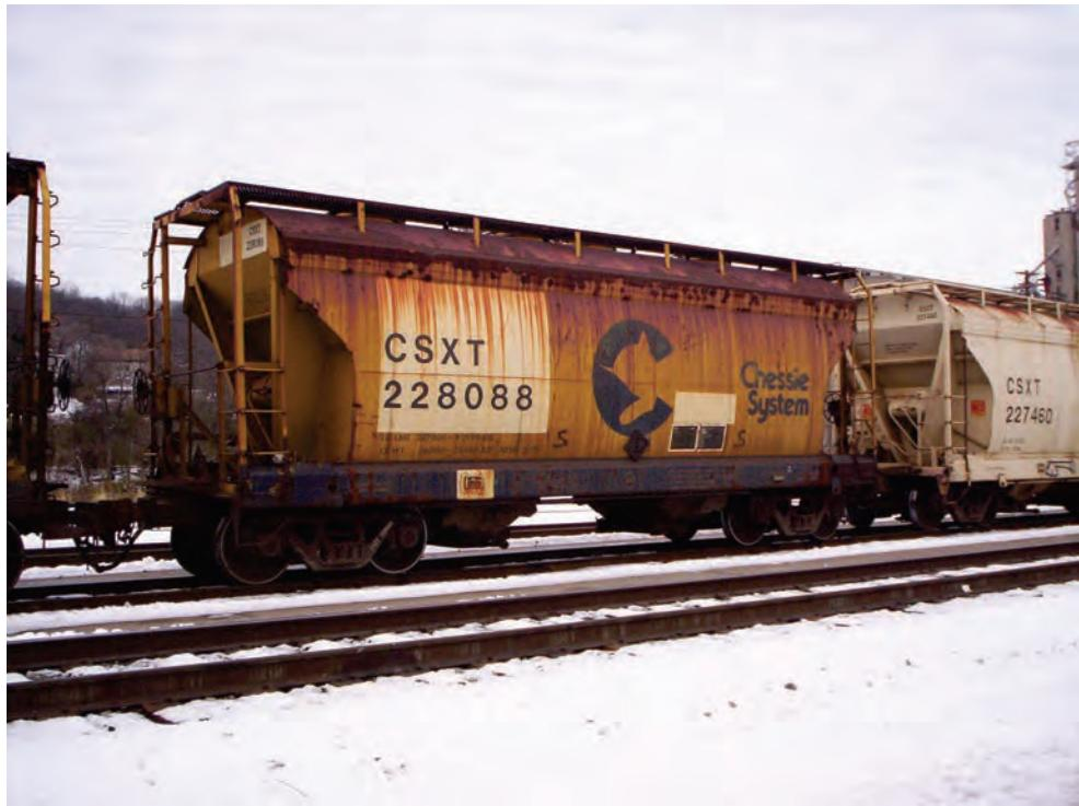
**CSXT 228088 (ex C&O 604704) and CSXT 227748** are former Chesapeake & Ohio Railway Chessie System two door gravity flow hoppers built for Chesapeake & Ohio Railway by American Car & Foundry. They are 41 feet 11 inches long, 10 feet 8 inches wide, and 15 feet 1 inch high. They have a load limit of 207,000 pounds and a cubic capacity of 2,700 square feet. Note the difference between the two cars in the manner in which CSXT painted over their former reporting marks.
