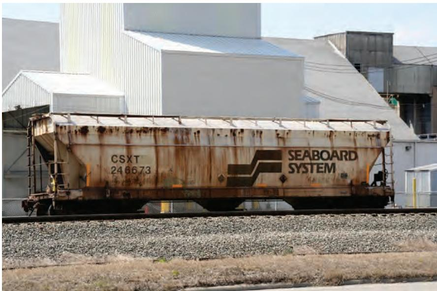
CSXT 246673 was built by ACF as L&N 240536. L&N was owned by Seaboard System and thus its logo is on the side of the car. Note the difference in placement of the Seaboard logo between CSXT 246673 and CSXT 247656. CSXT 244673 is 58 feet 1 inch long, 10 feet 8 inches wide, 15 feet 1 inch high and has an internal capacity of 4,660 cubic feet and a carrying limit of 199,000 pounds.
