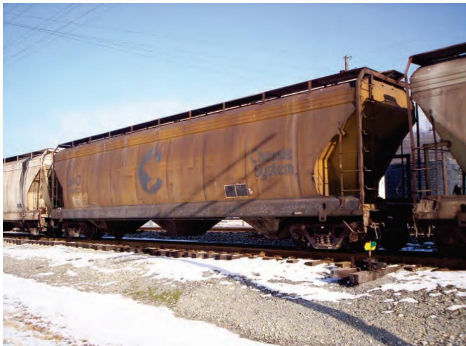
**B&O 606257** was built as a three bay hopper by ACF. Seen here at Toledo, Ohio, in 2011, she is 58 feet 1 inch tall, 10 feet 8 inches wide, and 15 feet 1 inch tall. With an internal capacity of 4,600 square feet, she can carry 198,000 pounds of goods.
