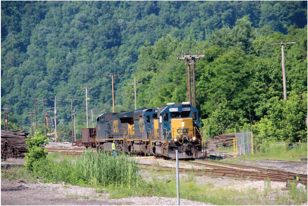
Seen heading out of the Shelby Yard locomotive service area to pick up a unit coal train tied down in the yard are CSXT 8029, a SD40-2; CSXT 4037, an EM SD40-3; and CSXT 646, a GE CW60AC. Note the conductor is on the ground throwing the switch.
