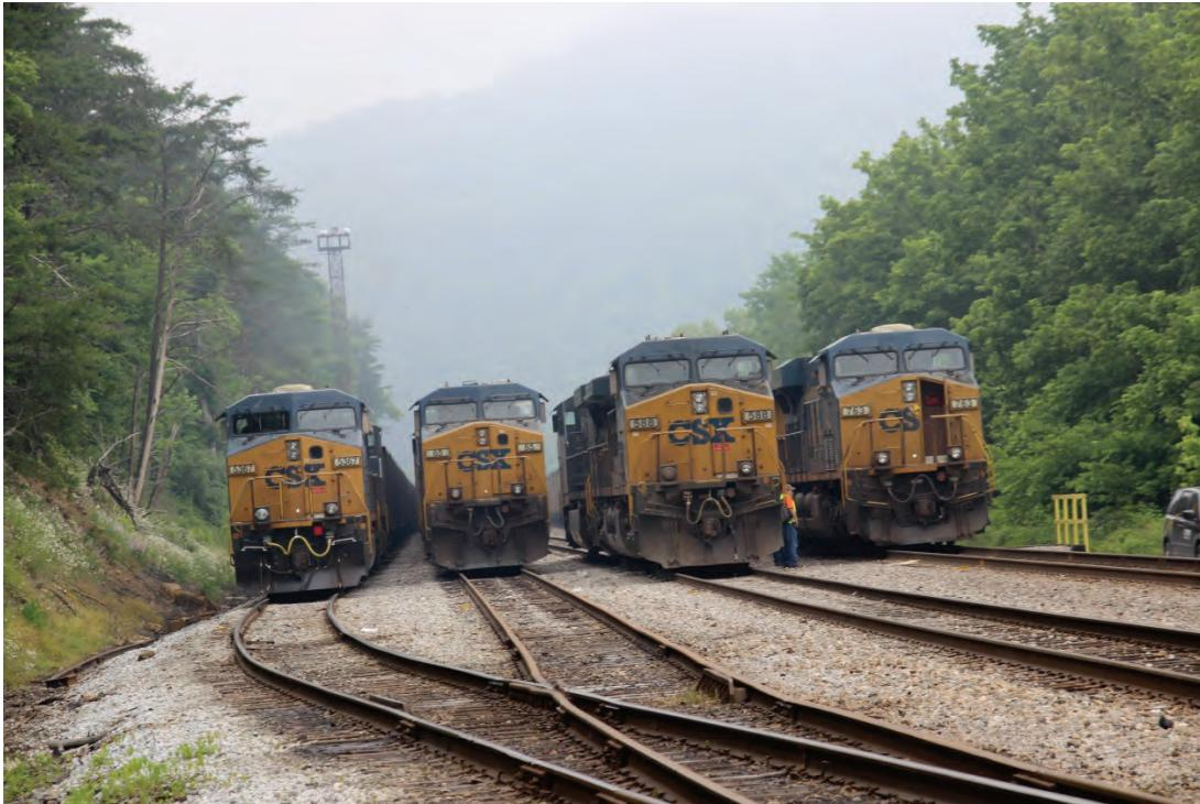
Thursday night at the south end of Shelby Yard CSXT had on display an imposing line up of locomotives. From left to right are CSXT 5367, a GE ES44DC with a unit coal train; CSXT 65, a GE AC4400CW with a unit coal train; CSXT 588, a GE AC4400CW-H in helper service; and CSXT 763, a GE ES44AC-H heading up an ethanol unit train.
