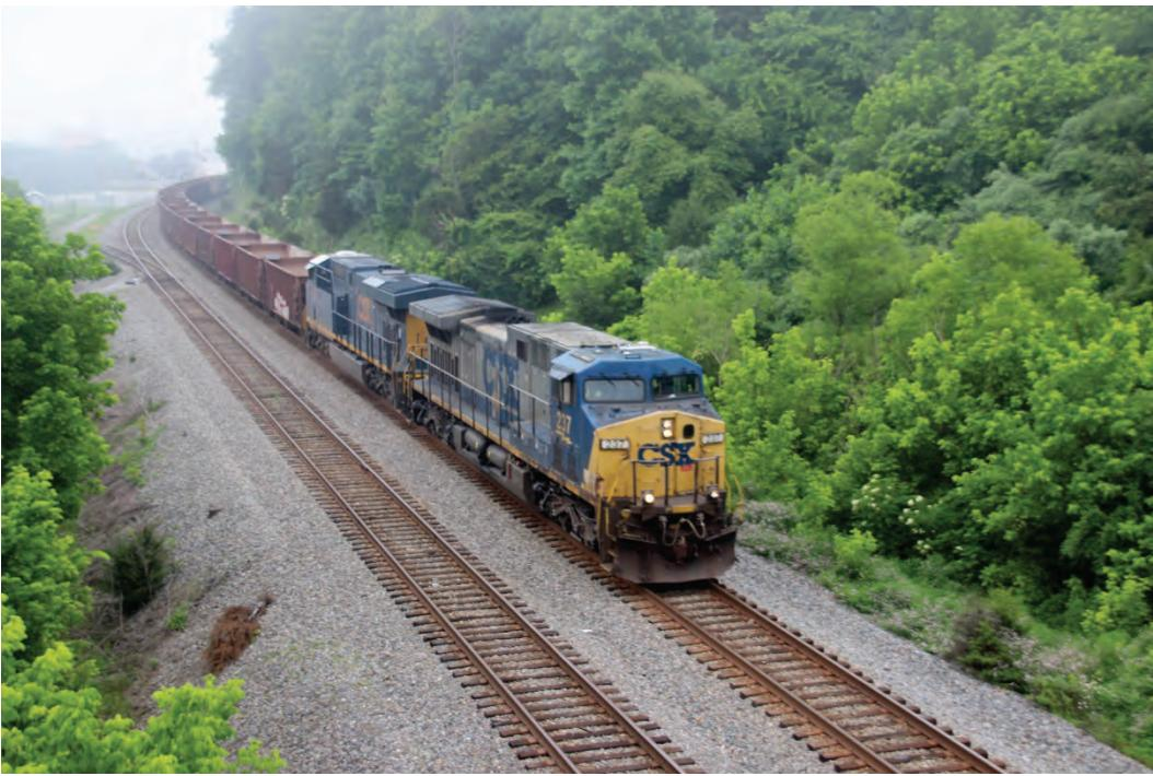
**CSXT 237, a GE CW44AC, and CSXT 3098, a GE ES44AH, lead a unit ballast train north on the main at Coal Run.**
