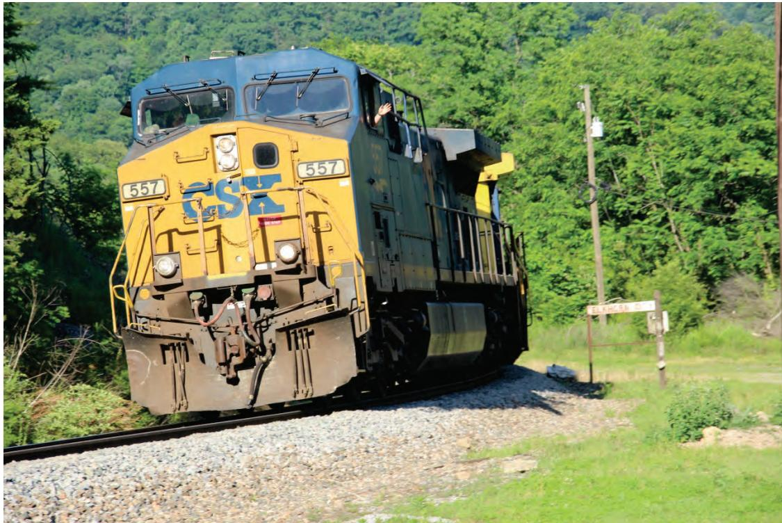
**CSXT 557 and CSXT 526, both GE CW44AC units, are seen at Elkhorn City running light back to Shelby Yard after completing their unit coal train pushing service.**
