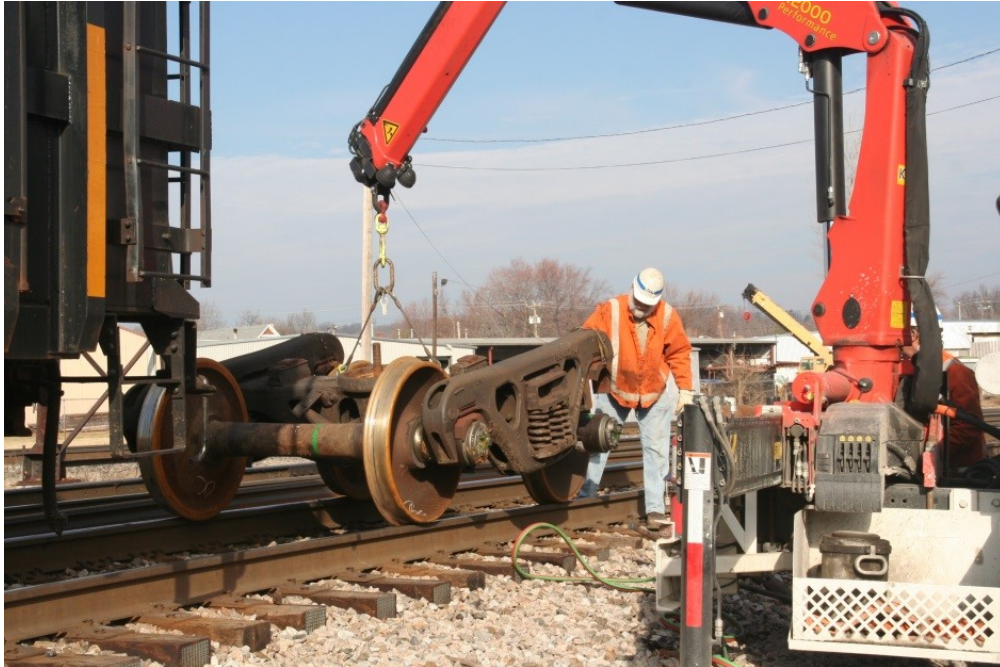
Above: Damaged wheel #4 is removed and a new wheel is mated with the truck.
