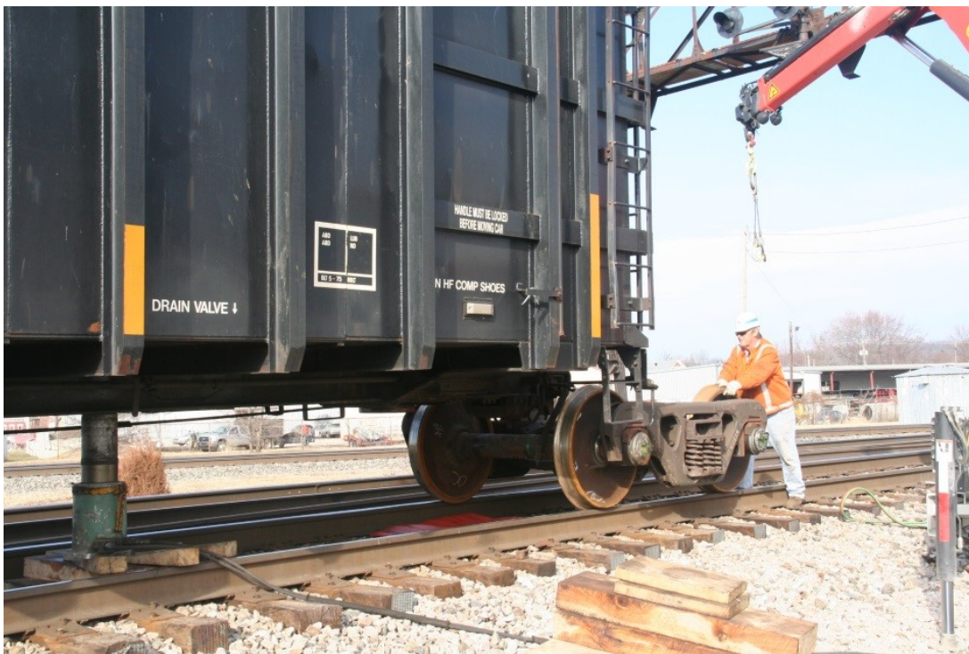
Above: Damaged wheel #4 is removed and a new wheel is mated with the truck.
