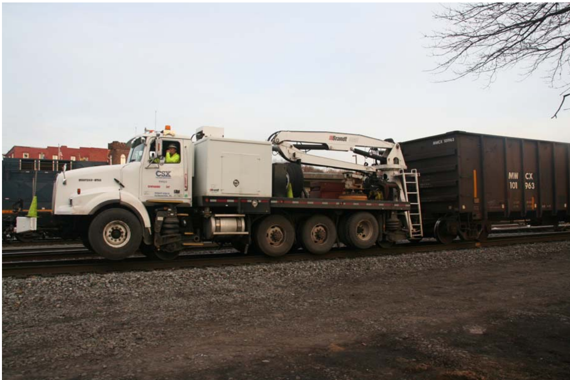
Above and below: CSXT 999011 is a Brandt Truck. It is used by Section Gangs for track repair but can also be used for moving freight cars. Here CSXT 999011 is moving a string of wood chip hoppers at Cumberland, Maryland.
