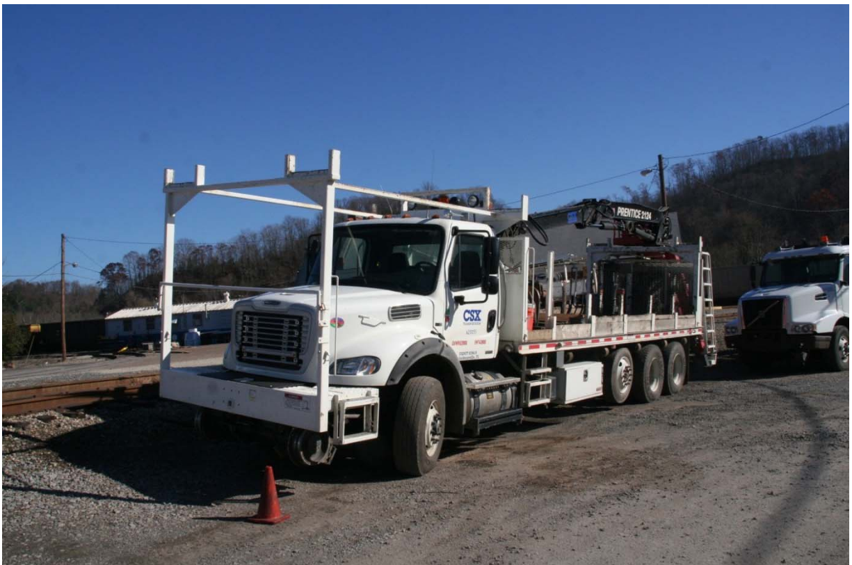
Above and below: CSXT 620055, a grapple truck used by Maintenance-of-Way gangs for lifting and carrying ties or rails. She is seen near Columbus, Ohio.
