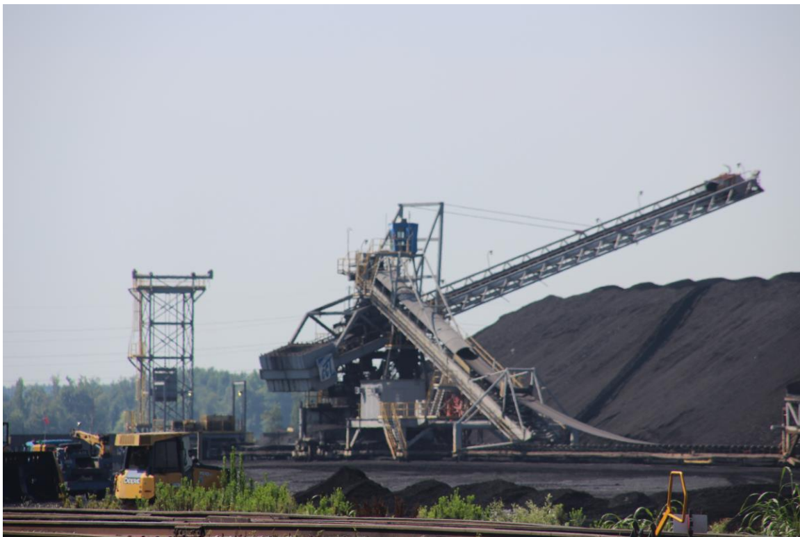
Above and below are views of the conveyor belt used in depositing coal in the blending area.
