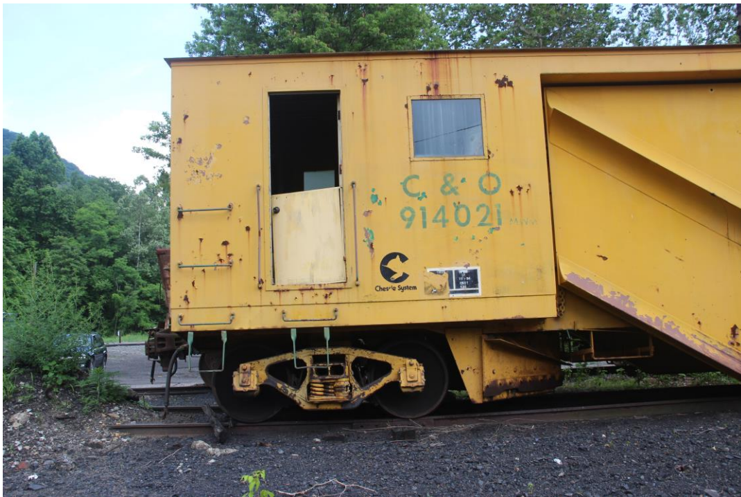
A view of the left side entrance to the mechanical room. The plow’s wing can be seen on the right. Located in front of the rear truck is an auxiliary plow to remove snow from the rail missed by the main plow.
