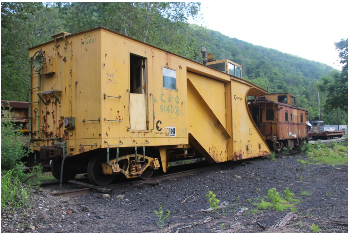
A view from the “B” end down the right side. The plow’s wings are to the front of the mechanical room. The caboose is C&O 903572.
