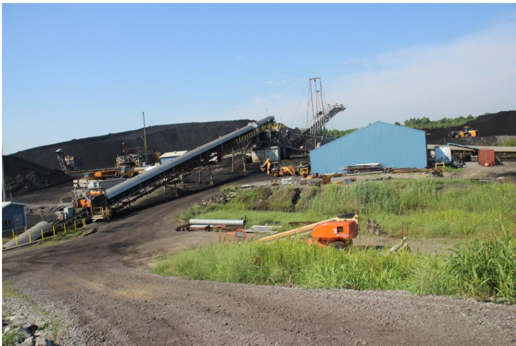
Looking west from the scale house toward one of the storage piles where Wyoming Basin and Western Kentucky coal is blended to provide the correct BTU and ash content required by the purchaser of the coal.
