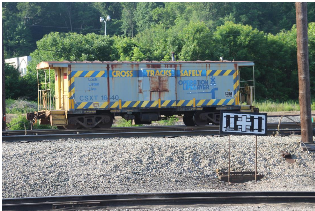
The knowledgeable railfan will not identify CSXT 16440 as a caboose, but as a shoving platform. However, CSXT 16440 is not a shoving platform but instead a spaced car used at South Charleston Yard when moving placard chemical cars. Note the Chessie Safety Ladder sign at the left of the CSXT 16440.
