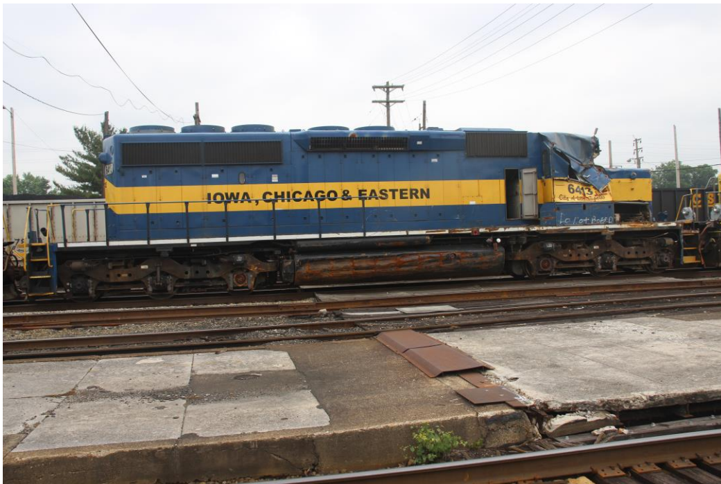
Sitting in back of the CSXT office building was Iowa, Chicago & Eastern Railroad #6413, City of Minneapolis, an EMD SD40-2. She was heavily damaged in a wreck on 26 March 2012 and had recently been bought by CSXT for conversion to a SD40-3.
