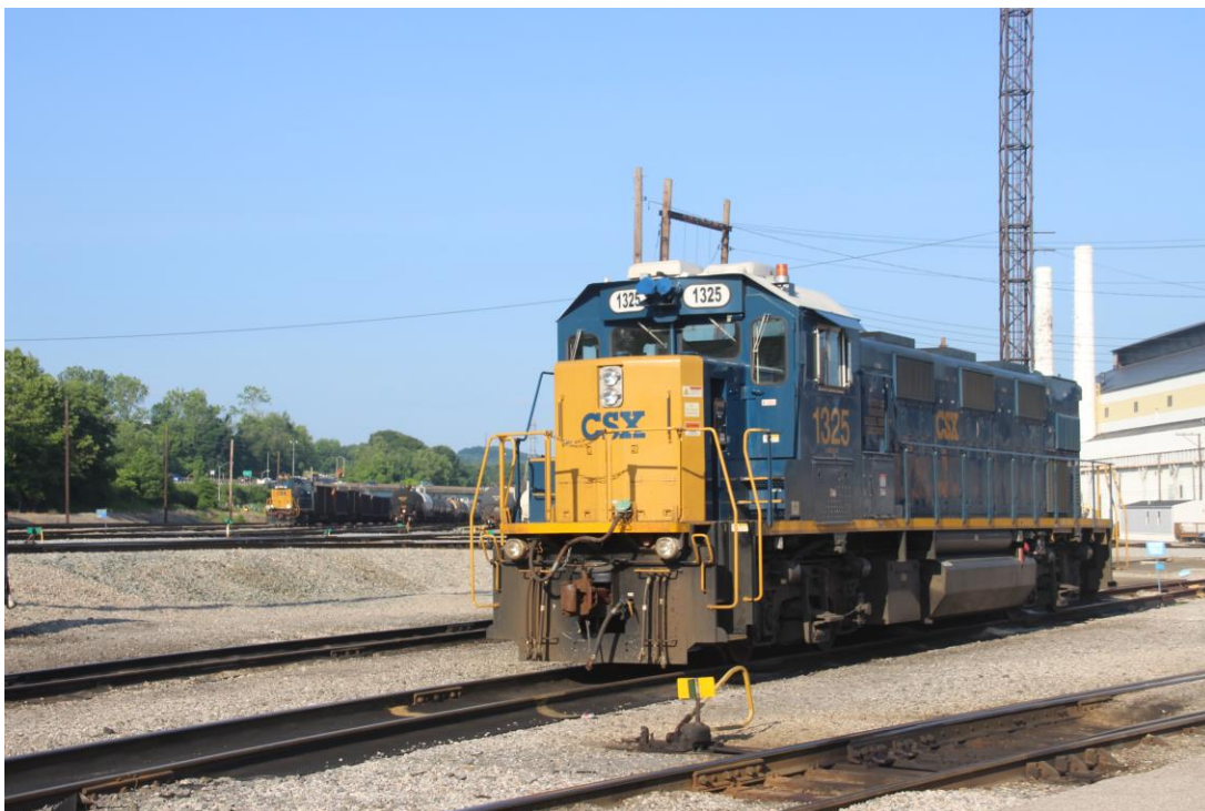
CSXT 1325, a National Railway Equipment 3GS21B-DE, had just been parked by her crew after completing their shift. In the background CSXT 1208, an EMD MP15T, moves a cut of covered hoppers.
