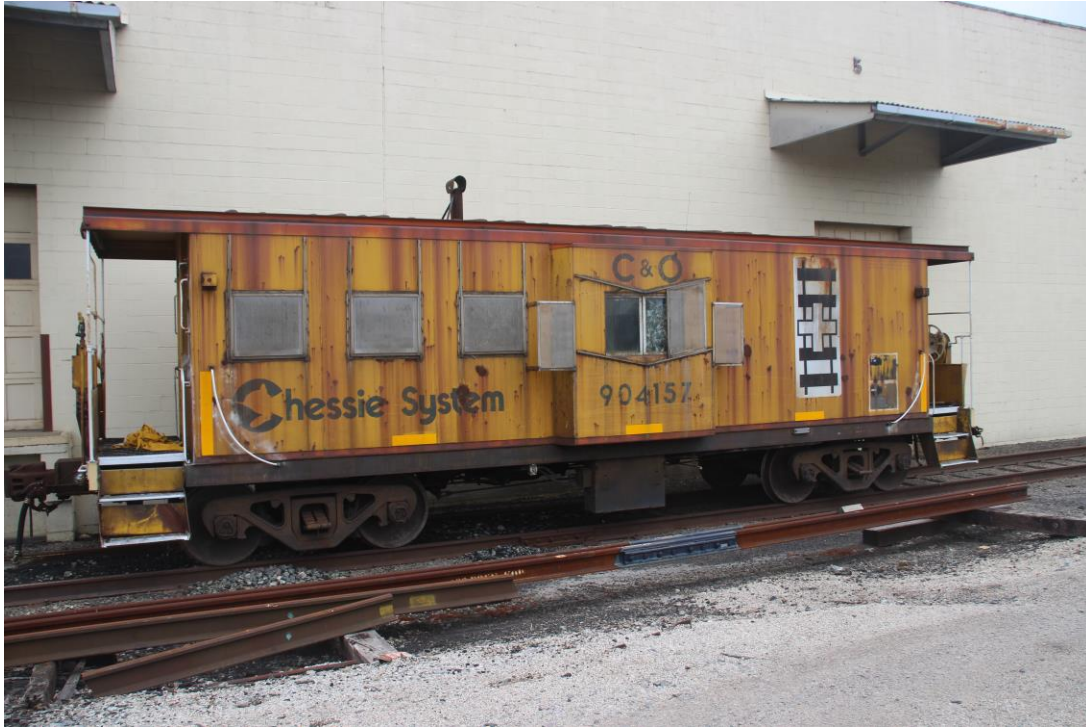
Still in Chessie paint and C&O reporting marks, this CSXT shoving platform, C&O 904157, was found in the CSXT Huntington Yard. Note the correctly painted vertical safety ladder painted on her side, unlike the horizontal safety ladder sign in the South Charleston Yard.
