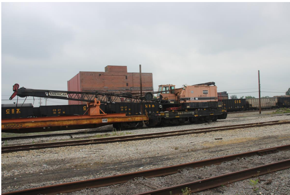
Found sitting in the Huntington Yard was CSXT crane, LRC 500, riding on crane car B&O 950468. The crane's boom rests on CSXT boom support car 960562.
