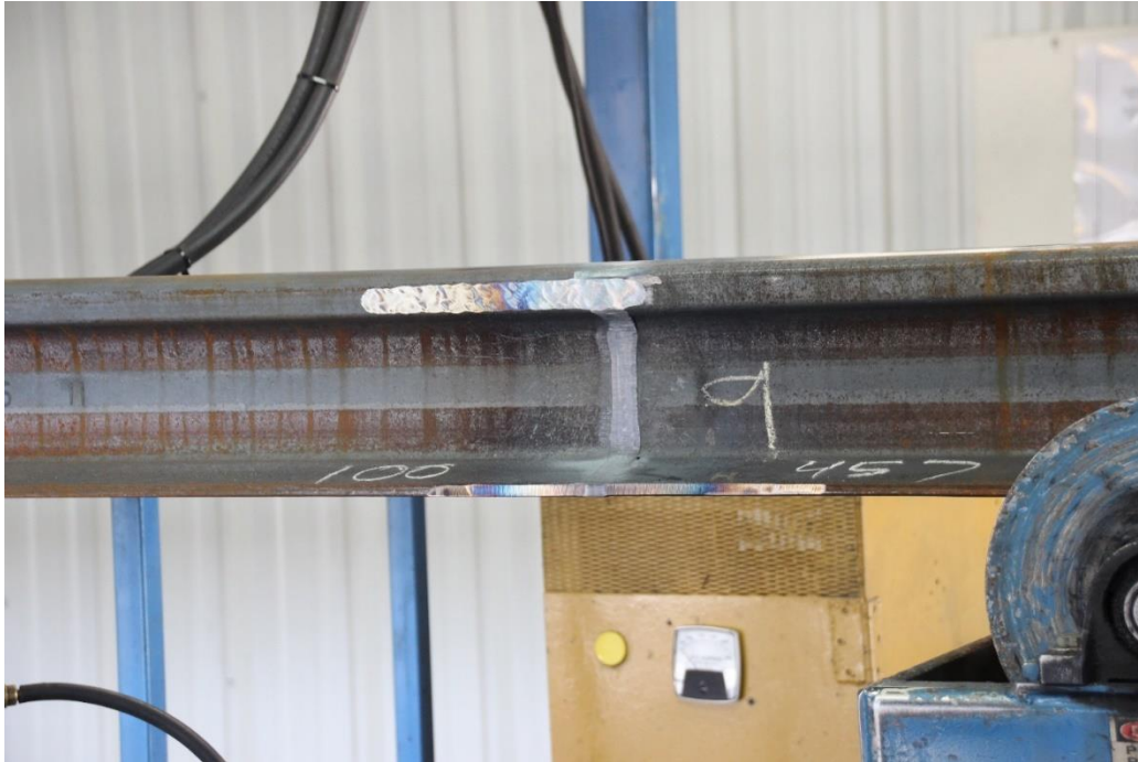
The rail joint after it leaves the hand grinding station
