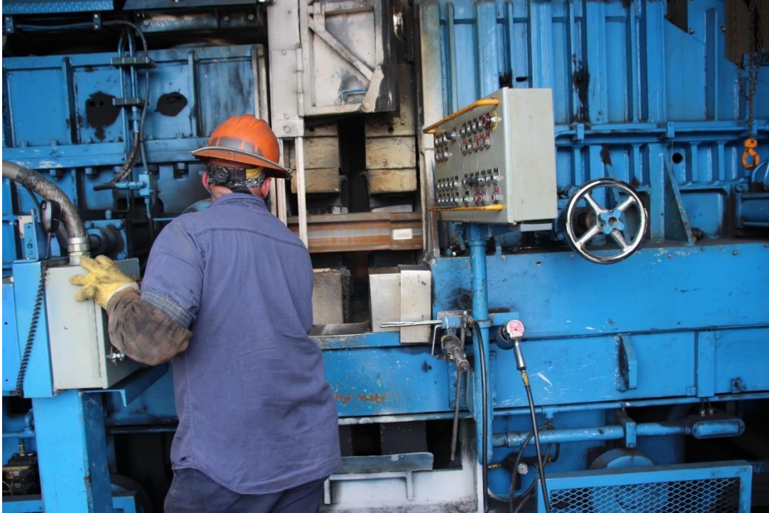
The rail welding machine. Hydraulic rams are being used to aline the two rail butts to each other.
