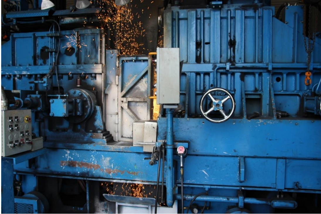
The welding machine welding the two rail butts together. This operation takes 15-seconds.
