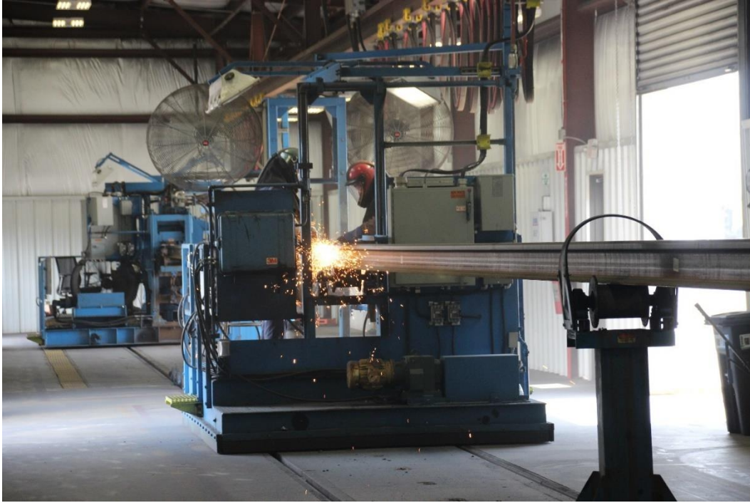
A view from the automatic rail base grinding station toward the hand operated buffering station with the inspection station in the distance
