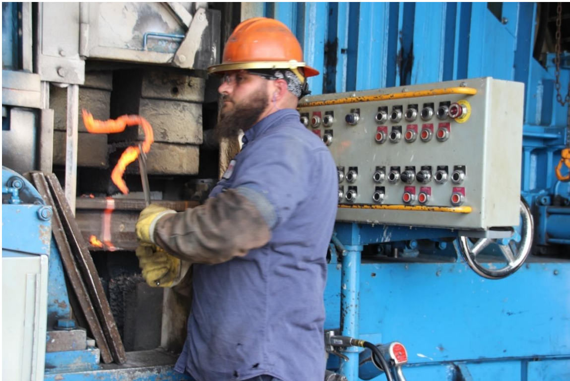
Slag being pulled away from the newly welded rail joint
