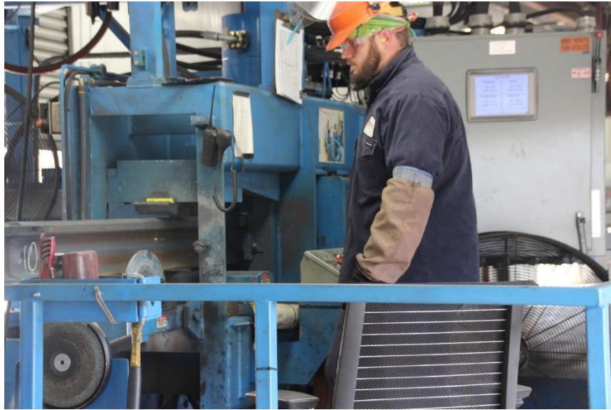
Hydraulic ram pressure being applied at the inspection station to the weld area to insure that the rail does not sag or hog at the welded joint
