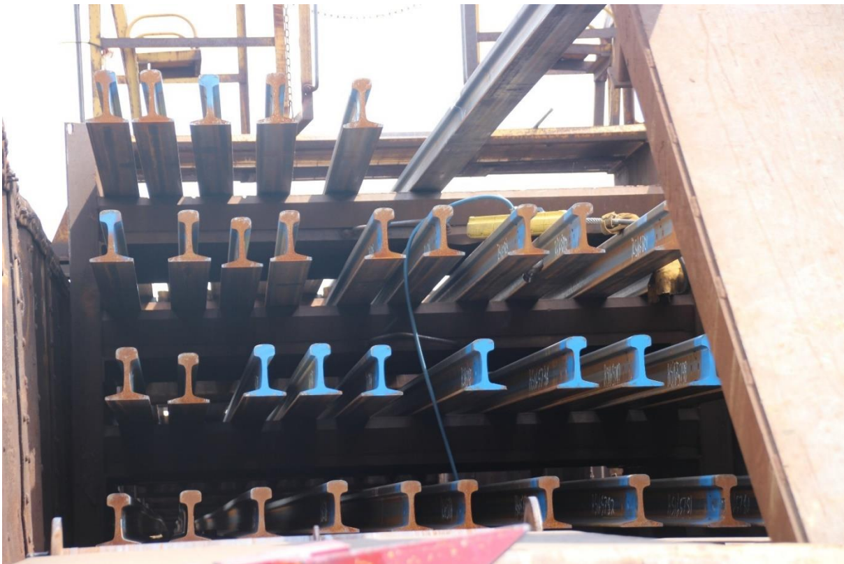
An end view of the newly welded rail on board the rail car. The rail ends are painted blue to indicate that they are Premium Head Hard rails.
