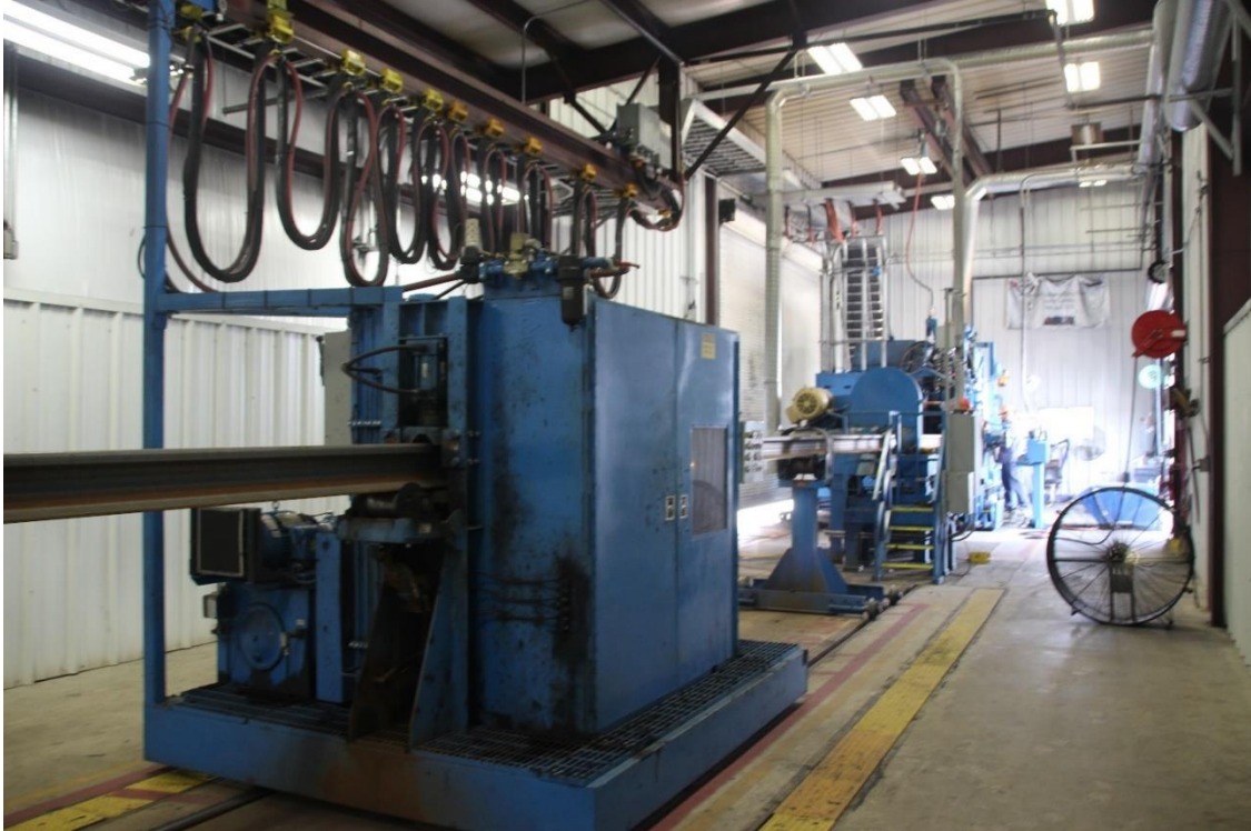
A view from the automatic rail base grinding station toward the welding machine
