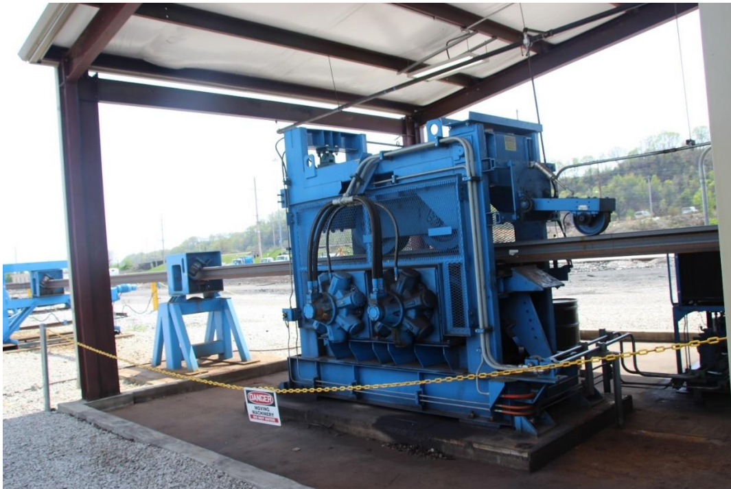
The come-along machine that moves the ribbon rail out of the welding building and onto the ribbon rail holding cars
