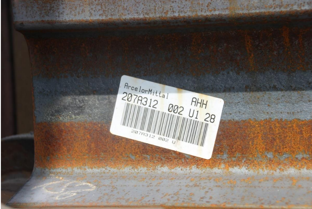
A close-up of one of the scannable bar reading codes on a rail. These bar codes contain inventory information.
