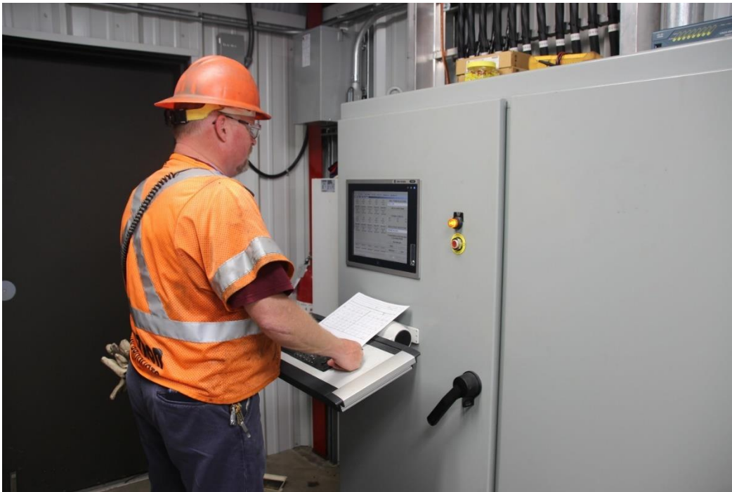
Setting the computer that controls the automatic buffer and manages the production run of the rail through the various stations. No photo was allowed of the automatic buffering station in operation.
