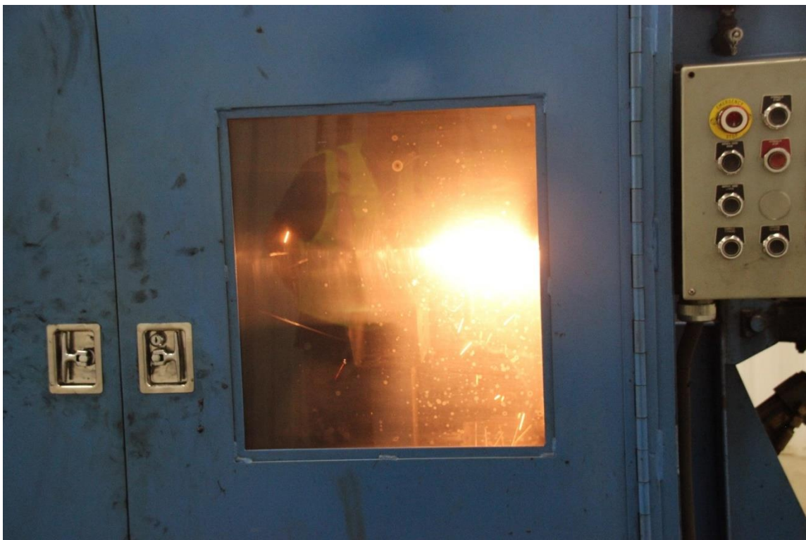
A view into the automatic rail base grinding machine. Sparks fly as excess material is roughly ground off the weld.
