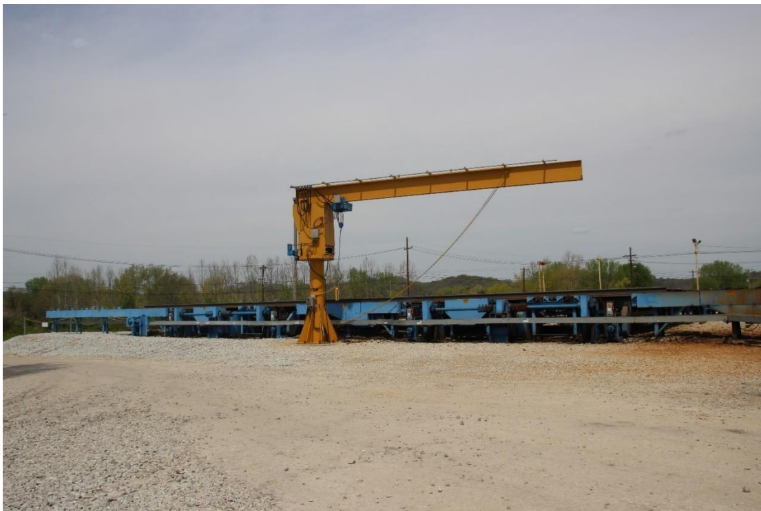
An overall view of the rail holding table. Individual rails are fed off to the right to a conveyor belt to carry them to the automatic buffer wheel building.
