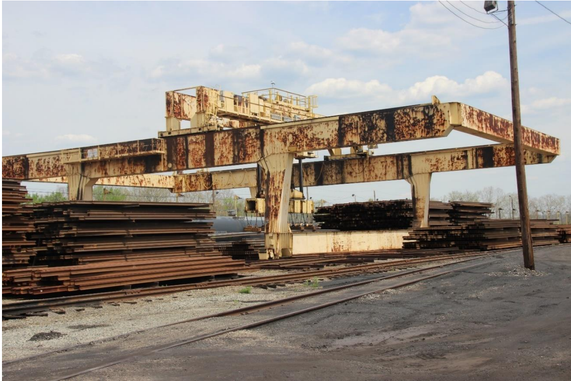
The overhead crane moving into position to pick up new rail for delivery to the rail holding table. In the foreground is a stack of old rail.
