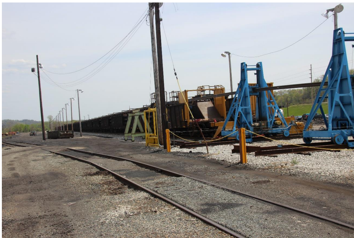
The ribbon rail being automatically loaded onto the ribbon rail car fleet
