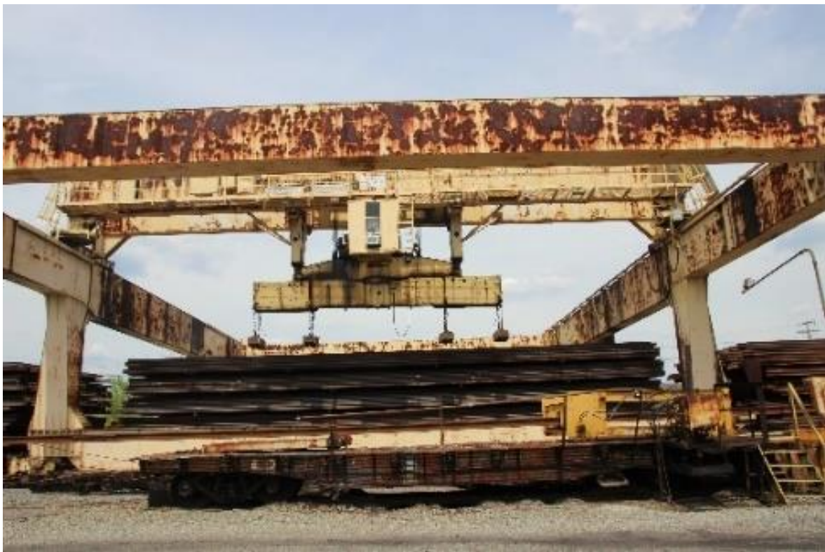
The traveling crane is preparing to pick up nine rails for transport to the loading table.
