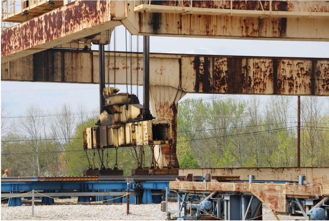
The nine sticks of rail being placed on the rail holding table
