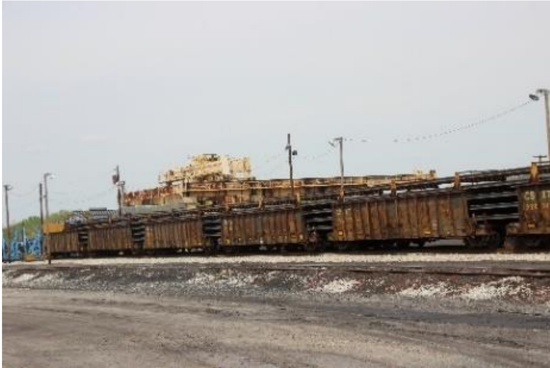
A view of 25% of the rail car train length as seen looking toward the rail welding shop. The rail rides freely in these cars on rollers and is not anchored in place.
