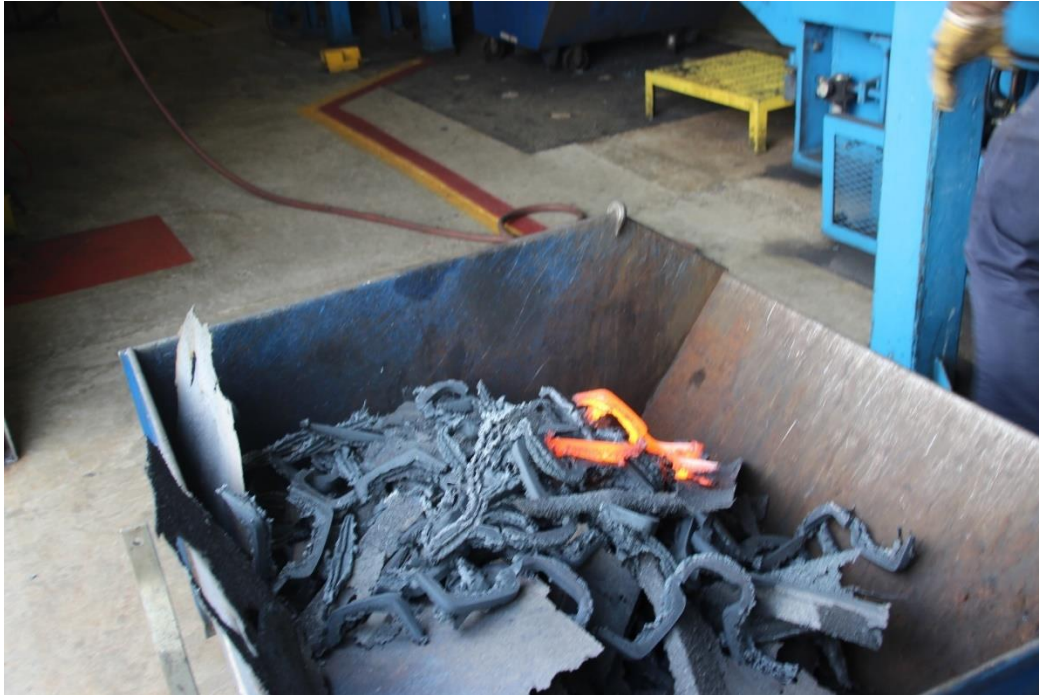
The slag from over 500 welds rests in a scrap collecting basket.
