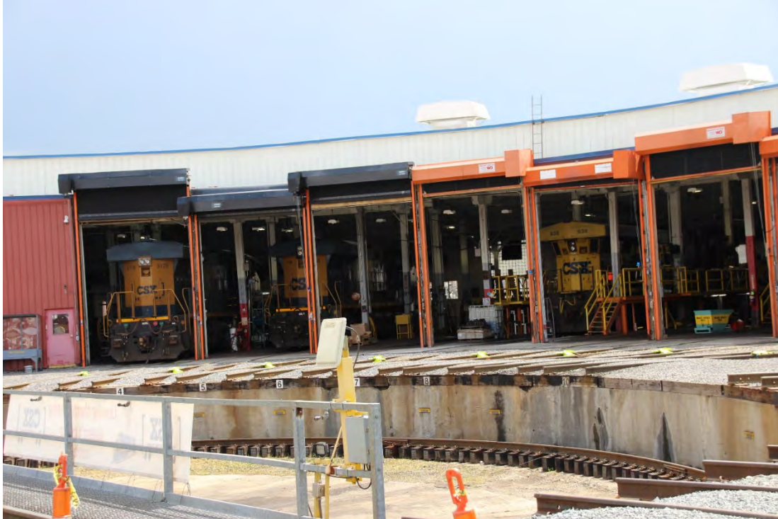
A view into the Cumberland Roundhouse. Three of the bays, #4, #5, and #7 house locomotives. From left to right CSXT 3176, a GE ES44AH; CSXT 788, a GE 44AC-H; and CSXT 688 a GE AC6000CW-H
