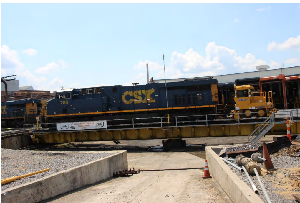
Above and next page. These photos show CSXT 788, a GE ES44AC-H, being pulled onto the turntable by the Trackmobile for turning. Note that even with most of the locomotives weight, on the left side of the turntable, the turntable is not flexing.
