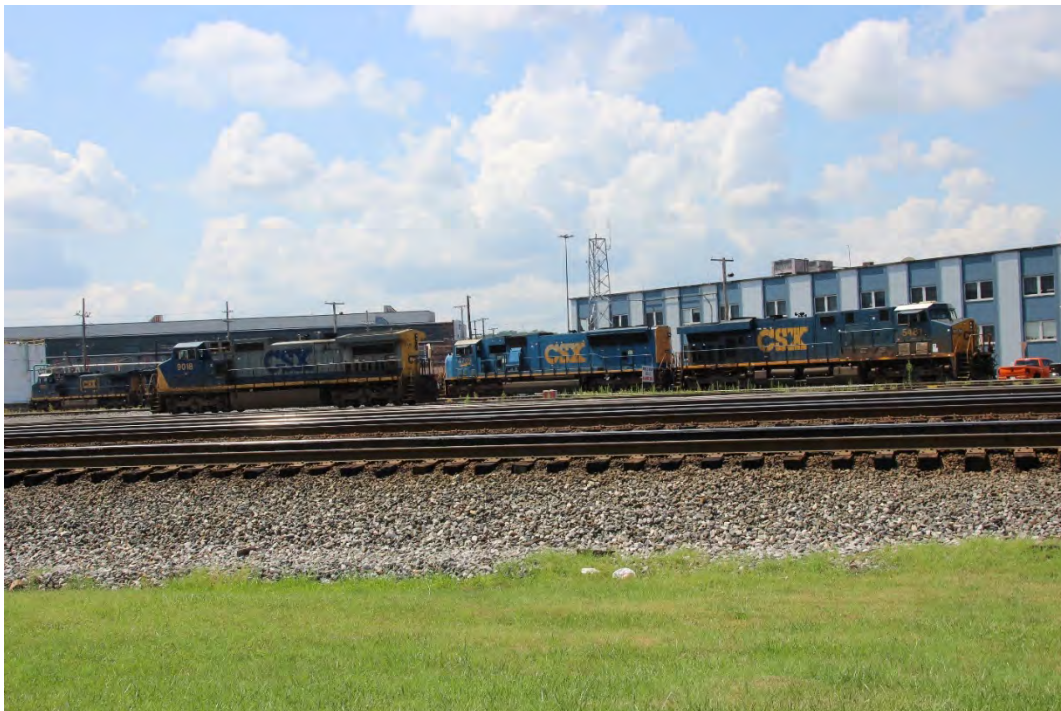
A view of the Cumberland Yard locomotive ready track located just to the east of the locomotive shop. From left to right are CSXT 7656, a GE C40-8W; CSXT 9018, a GE C40-9W; CSXT 4709, a GM SD70MAC ; and CSXT 5481, a GE ES44DC.
