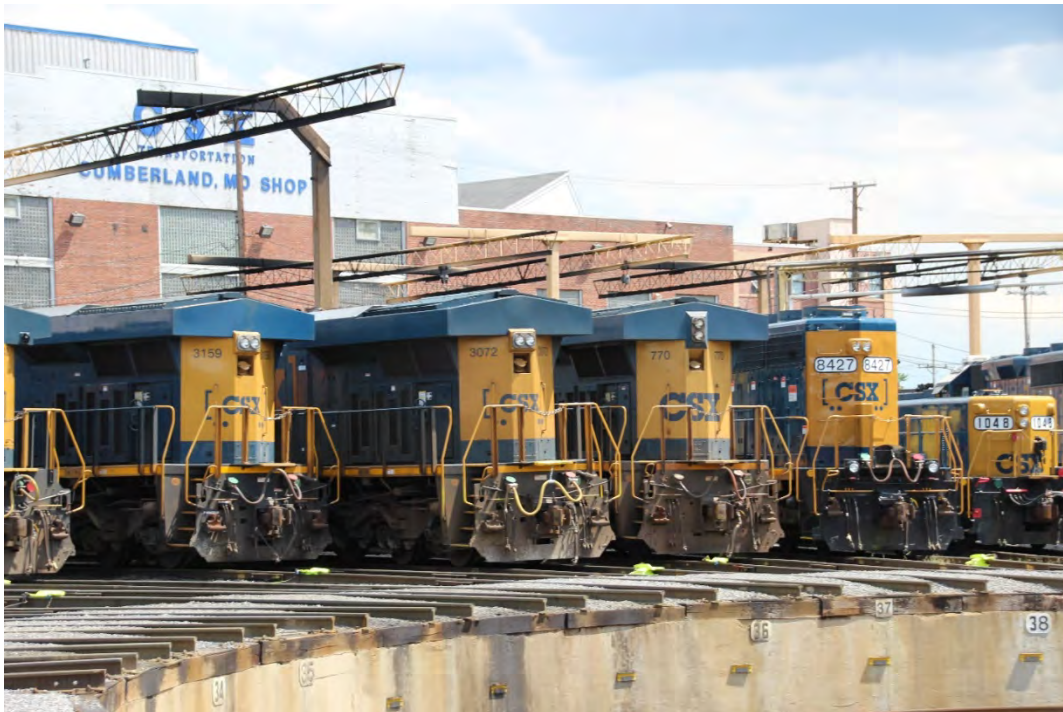
A close up view of the Cumberland Shop service tracks with CSXT 3159, a GE ES44AH; CSXT 3077, a GE ES44AH; CSXT 770, a GE ES44AC-H; CSXT 8427, a GM SD40-2; and CSXT 1045 a slug; waiting serving. Note the track numbers displayed on the upper edge of the turntable wall.
