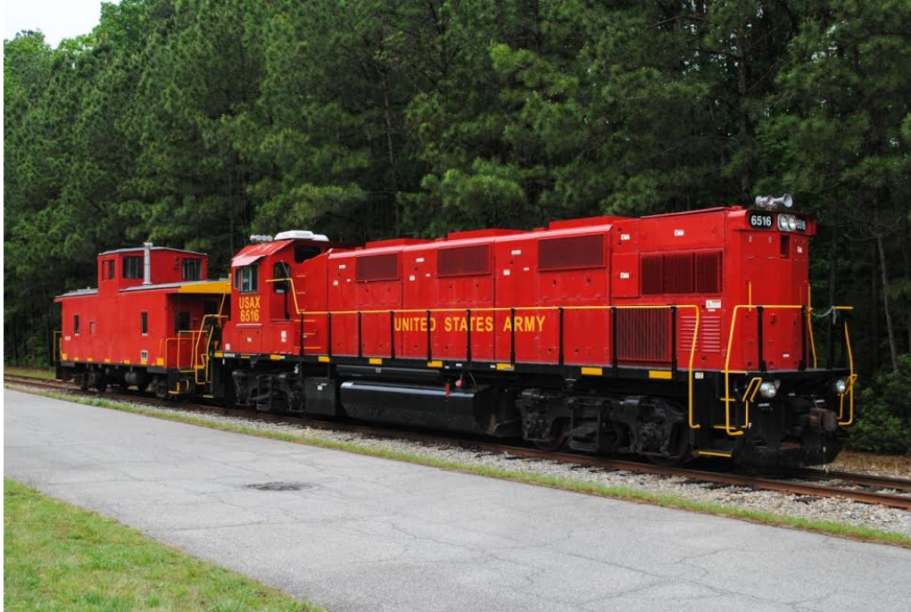
USAX 6516, a NRE3GS2IB with a caboose in tow, is heading for Grove Yard to perform some train make-up training.
