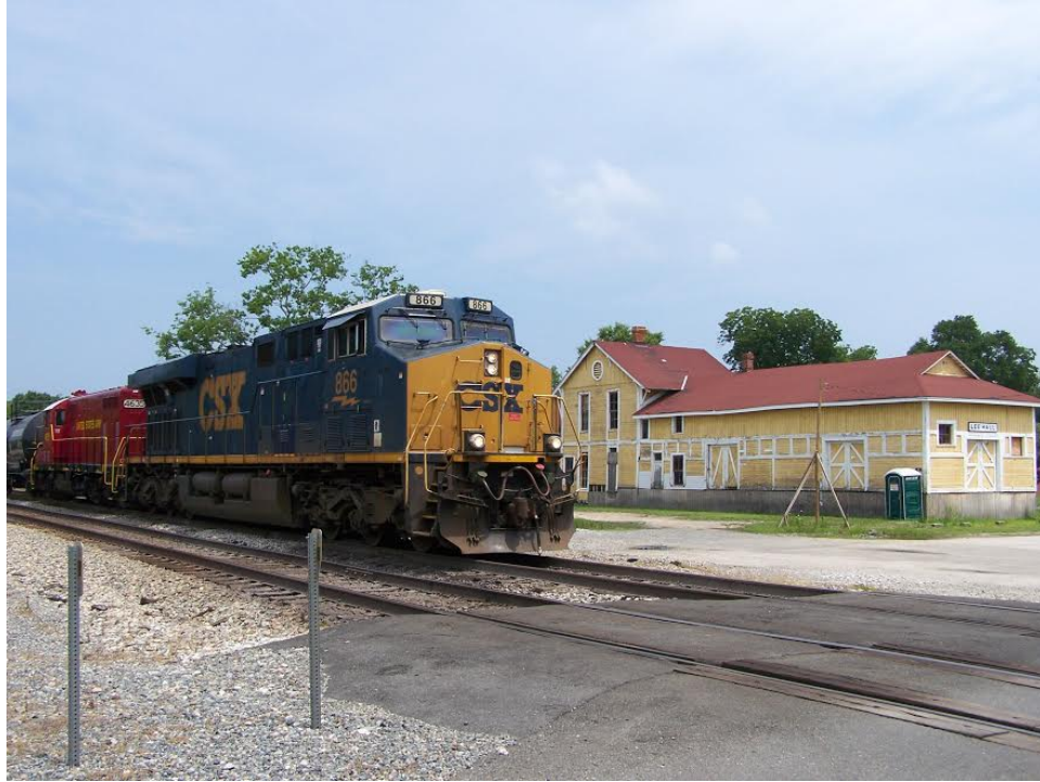
CSXT 866, a GE ES44AH, and U S Army 4636 are seen at Lee Hall Junction Yard. The Lee Hall Depot has just been moved from the south side of the track to the northside |
