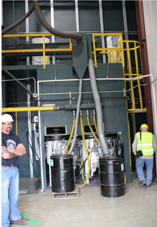
A view of the outside of the paint stripping facility. Used steel filings are carried into the barrel for reuse, while paint, stenciling, and other foreign matter goes into the right barrel for disposal.
