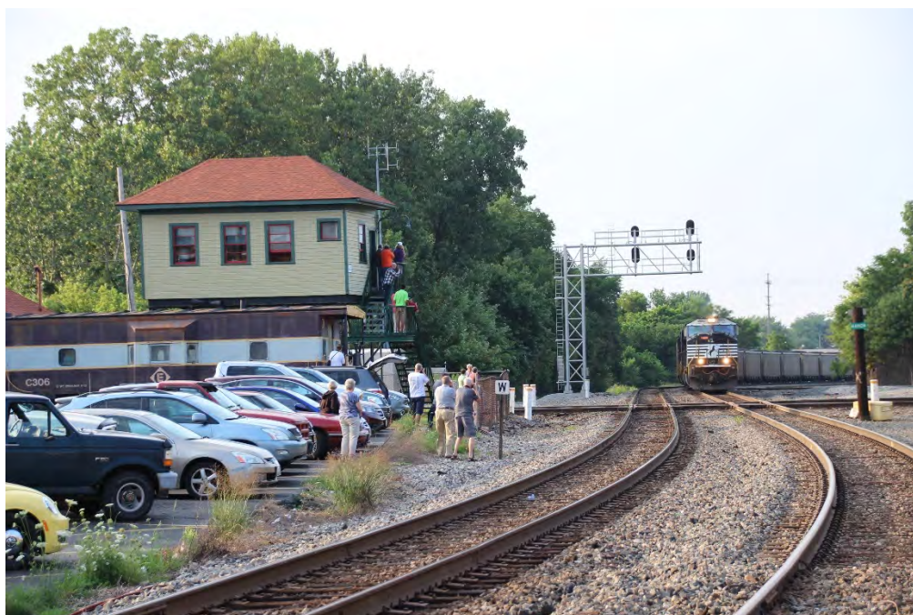
A view up the NS mainline at the CSXT/NS Diamond. AC Tower is to the left. Approaching is an empty NS unit coal train headed by NS 2593, an EMD SD70M; NS 7690, a GE ES44DC; and NS 9693, a GE DASH9-44CW.
