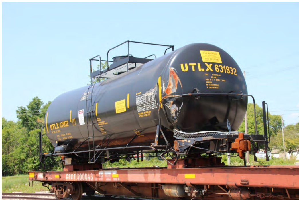
Sitting just outside of the UTLX plant was a string of flatcars with damaged tank cars onboard them. Some 99 percent of the work done at Marion on tank cars is normal FRA/EPA upgrade or maintenance work. Only 1 percent is tank car repair.
