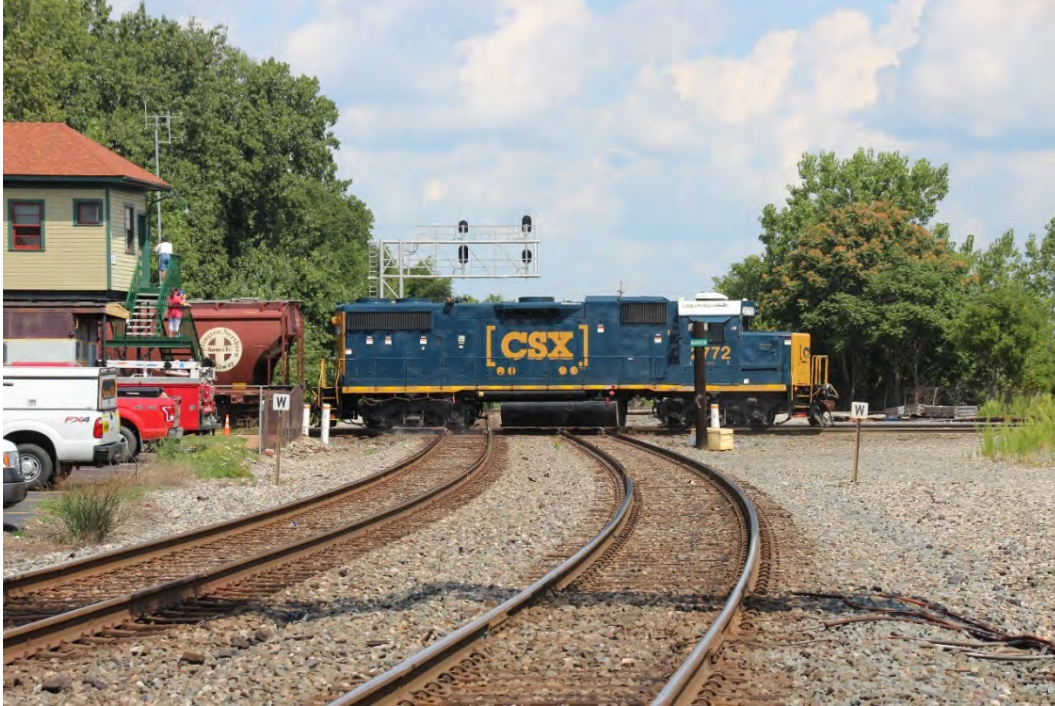
The local CSXT Yard switcher, CSXT 2772, an EMD GP38-2, is seen crossing the CSXT/NS Diamond.
