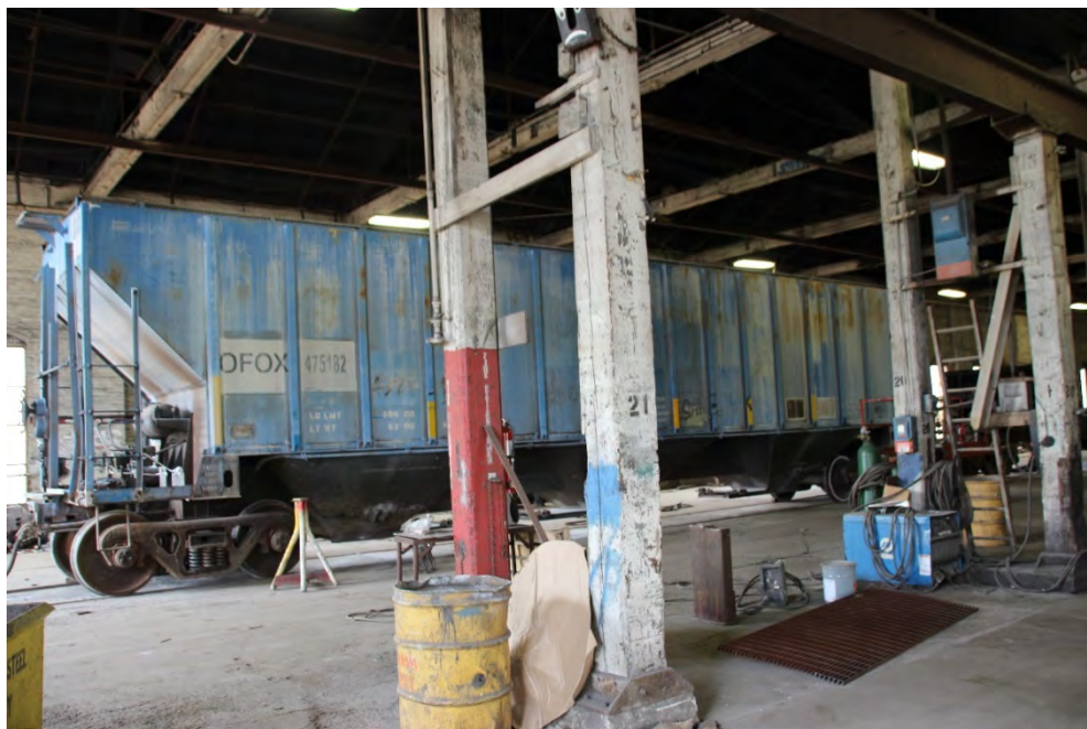
This covered hopper had just been pulled into the shop. Plant employees were preparing to jack the car up to remove its trucks and wheels to do work on the car's discharge doors.
