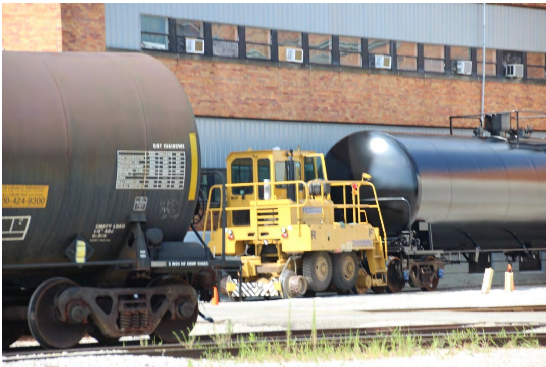
Movement of tank cars within the UTLX buildings at Marion is performed by a Trackmobile seen here moving a newly painted tank car to the stenciling shop.
