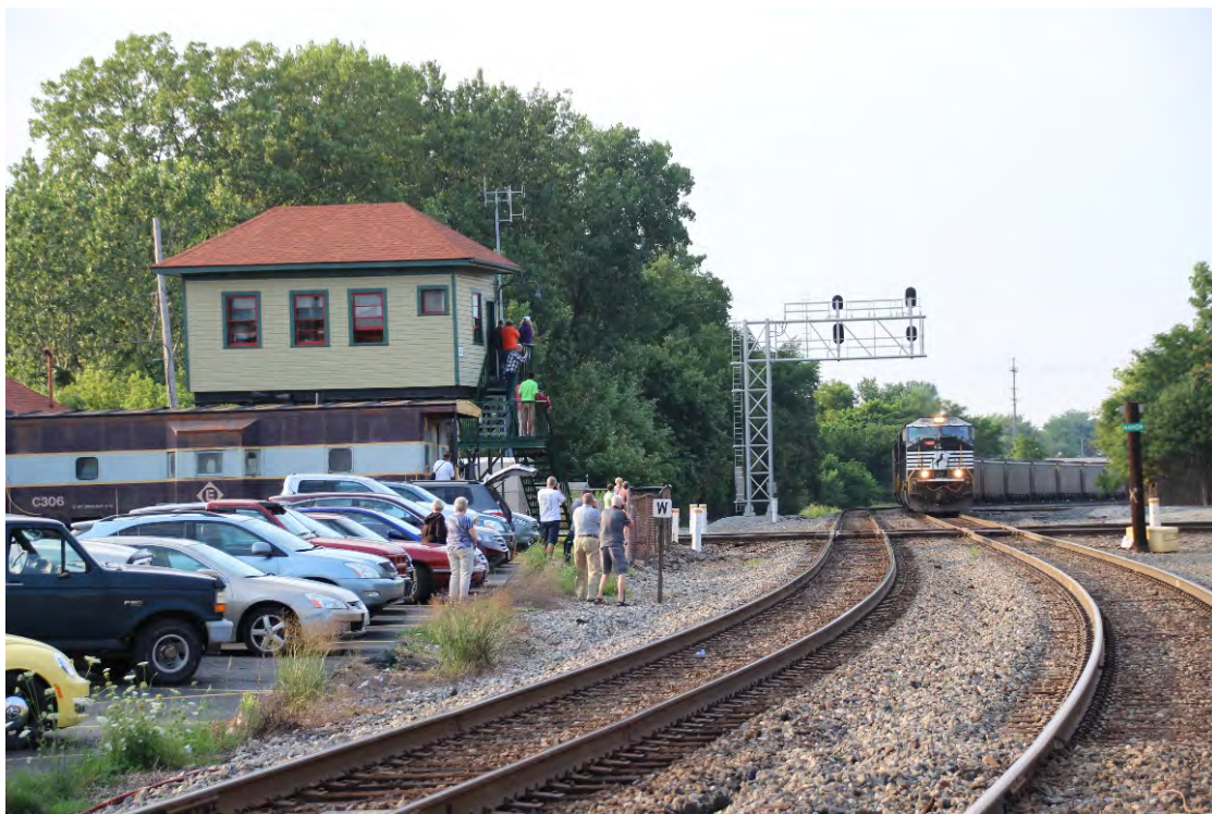
A view up the NS mainline at the CSXT/NS Diamond, AC Tower to the left. Approaching is an empty NS unit coal train headed by NS 2593, an EMD SD70M; NS 7690, a GE ES44DC; and NS 9693, a GE DASH9-44CW.
