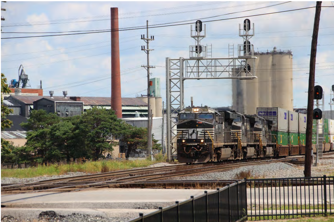
NS 7657, a GE ES44DC, and NS 9004 and NS 9577, both GE DASH9-44CW, lead a stack train over the CSXT/NS Diamond at Fostoria's Iron Triangle Rail Park.
