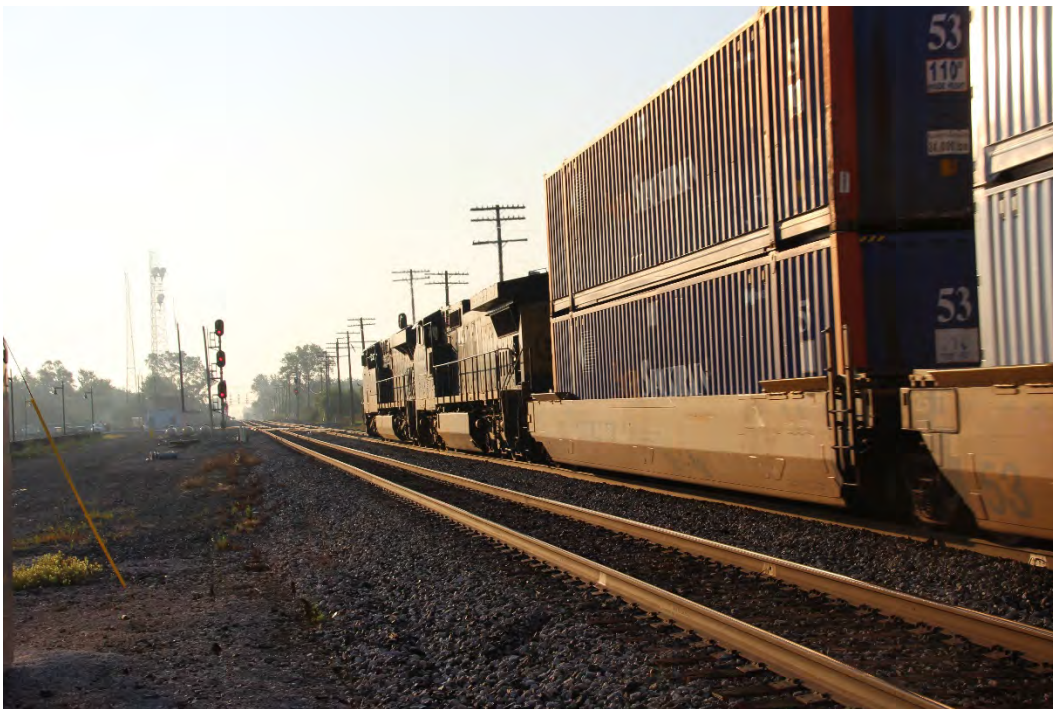
CSXT 866, a GE CW44AC/H, and CSXT 9030, a GE CW40-9, lead a stack train through Fostoria. The diamond is 100 yards in front of the train.
