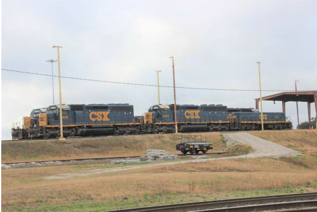
The hump yard switchers rest on the track leading to the hump. A CSXT scale car for calibrating the retarders is seen below the locomotives.
