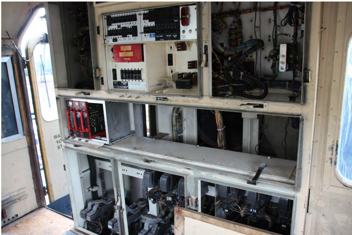
The cab of CSXT 1538 was getting all new wiring and instrumentation.
