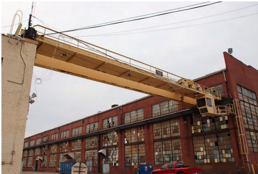
A close-up of the gantry crane that runs between the the Stores Department Building and the Erecting Shop
