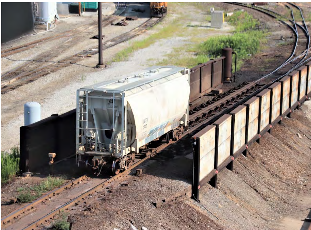
The covered hopper starts its trip down through the retarders.
