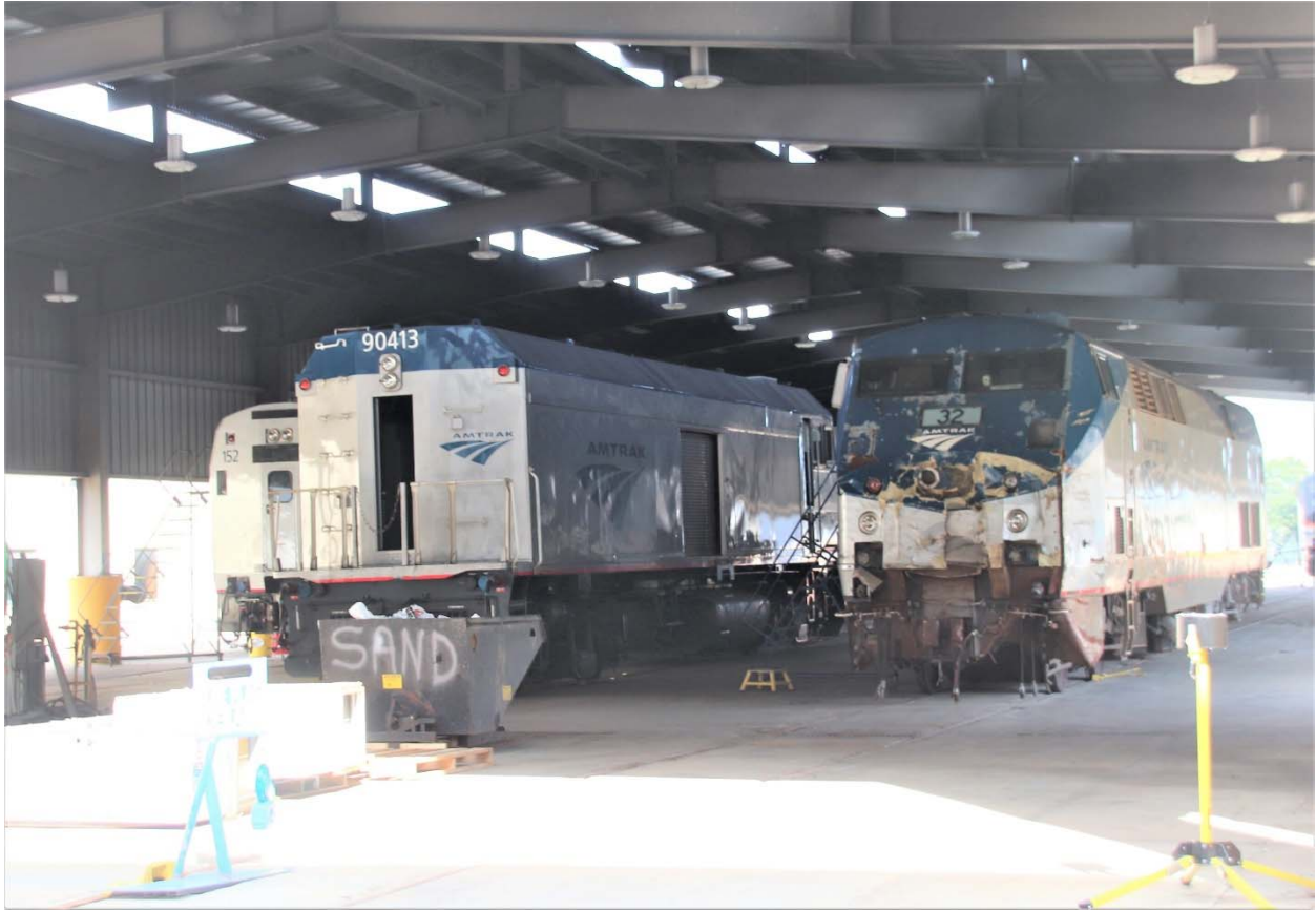
Amtrak 152, 90413, and 32 were all in the shop for repair of damage to their noses.
