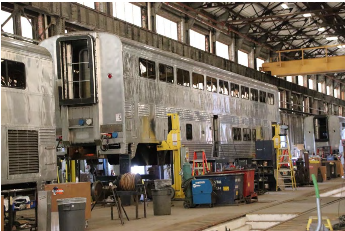
This Amtrak superliner had been gutted down to a metal shell and was to be completely refurbished.
