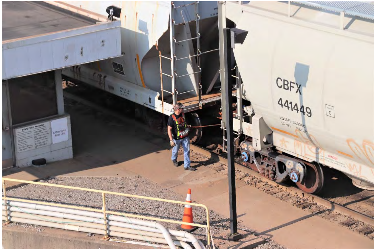
The pin puller has pulled the pin and the hopper is free to roll into the hump yard.
