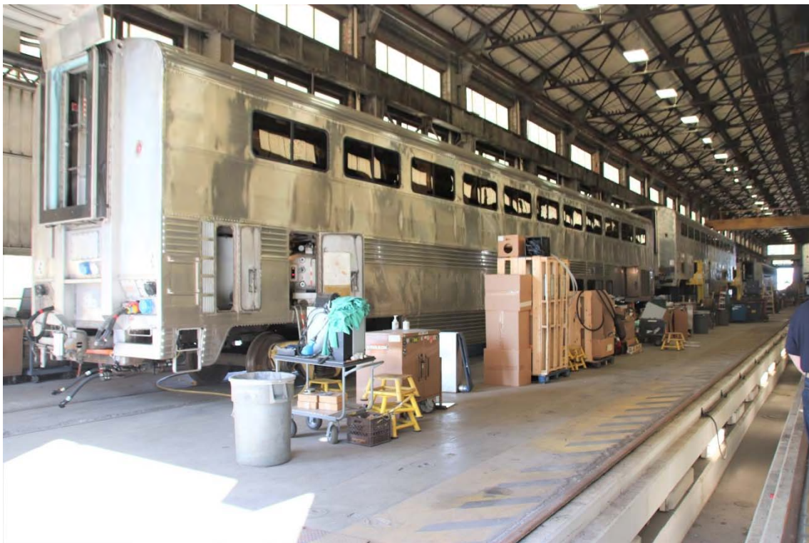
This superliner has been stripped down to bare metal and her insides gutted in preparation for rebuilding.
