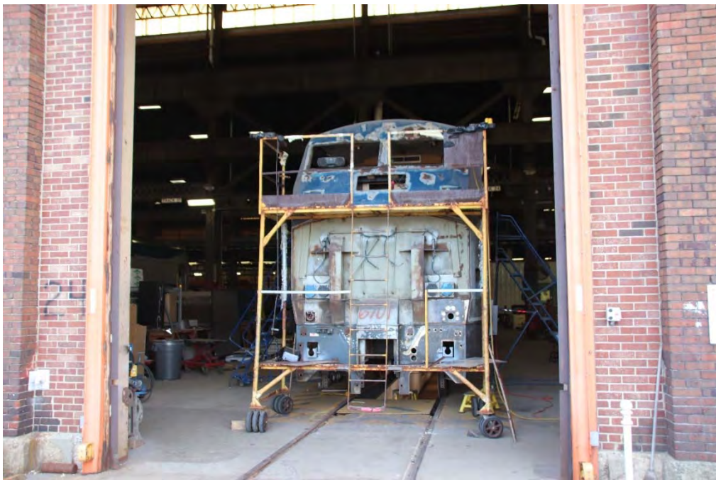
This unknown Amtrak locomotive was in the process of being stripped before her damaged nose could be repaired.
