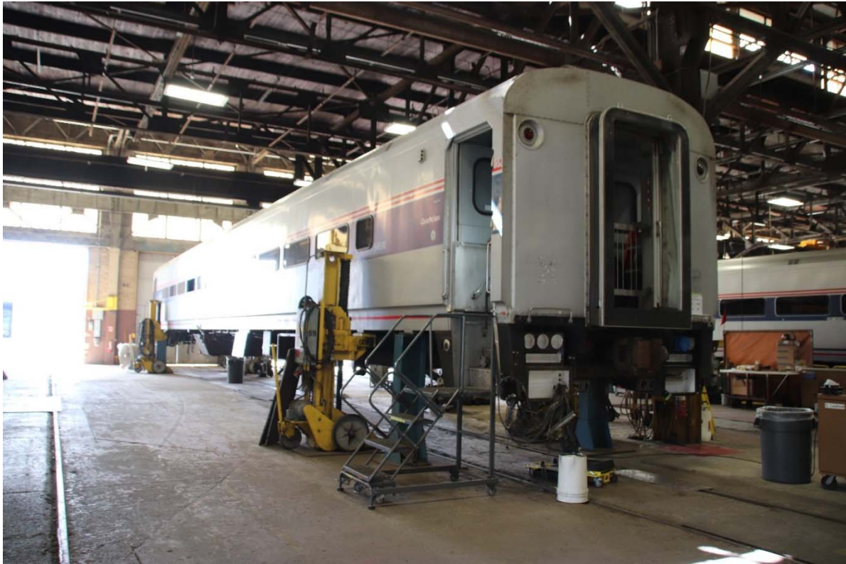
This coach was being outfitted with new trucks and brakes.
