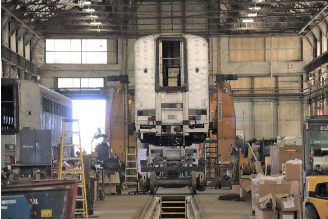
This superliner car had just been jacked up and her trucks were being removed for refurbishing.
