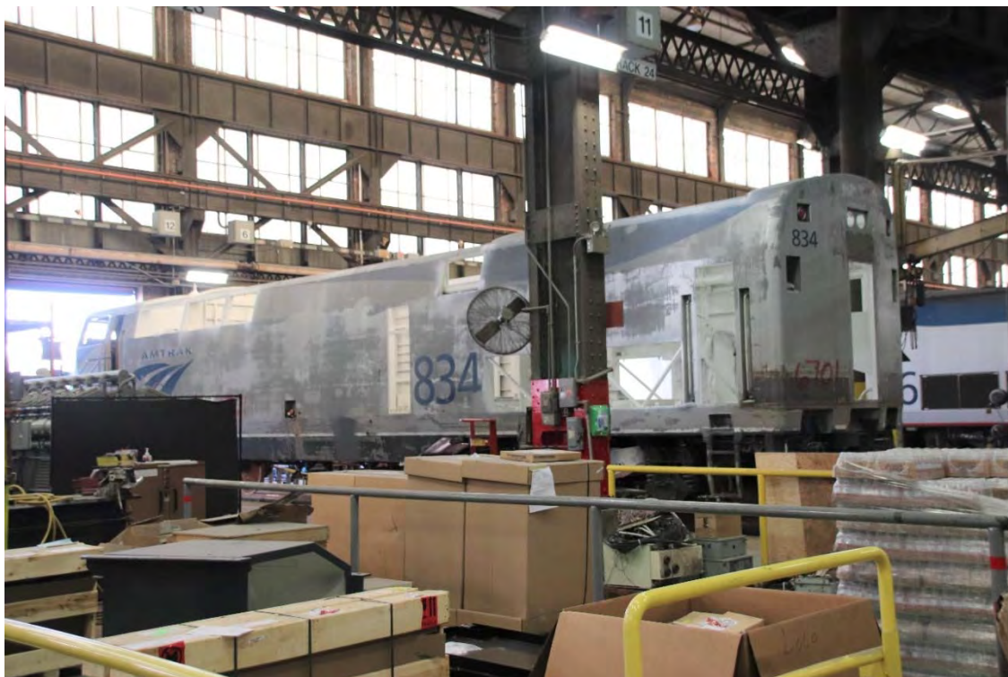
Amtrak 834 had been gutted in preparation for a major overhaul of her mechanical systems.
