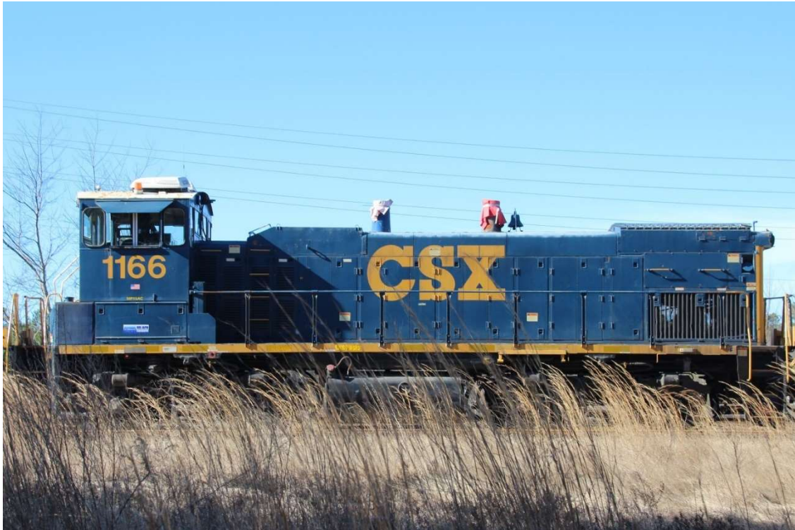
Among the locomotives in storage was CSXT 1166, a MP15AC. Note the covers over her stacks to prevent the injestation of rainwater.
