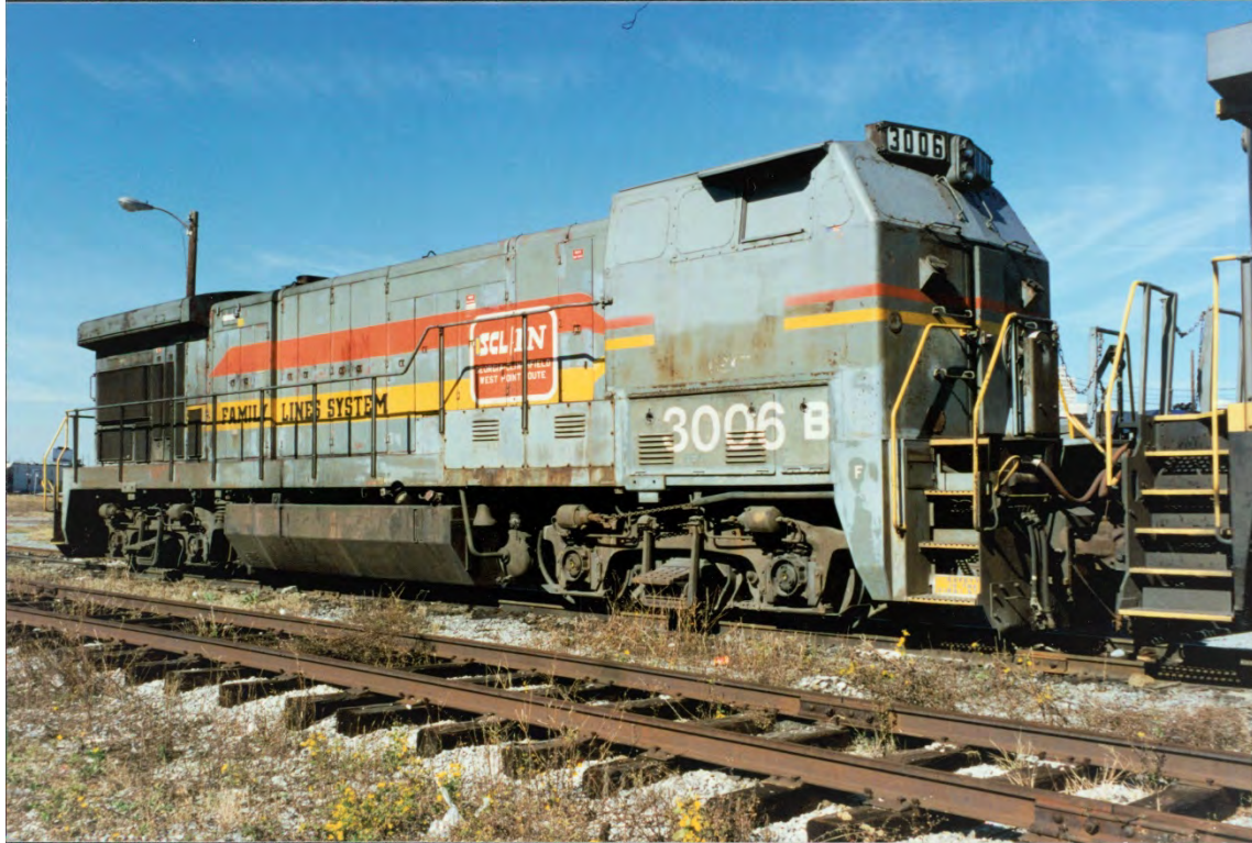
Above and below: It is 1993 and CSXT 3006 has been converted to a “B” unit. Note on the right-hand side the reporting marks are at the frame level and on the left at the cab level. Also, the “B” is smaller than the numbers. (CSXTHS photos)
