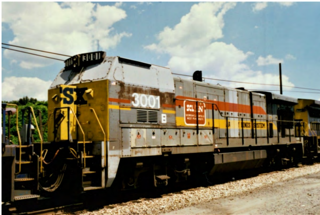
A view of the right side of CSXT 3001B. Here the CSXT ownership lettering is above the cab number. The two grills were to have supported an air conditioning unit that was never installed. (CSXTHS Photo)
