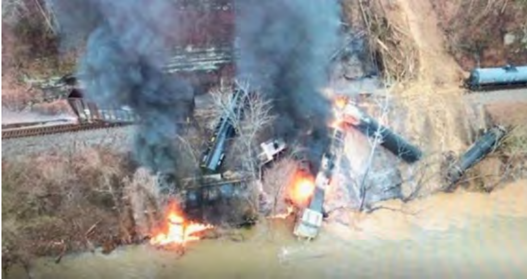
The earth slide that caused the derailment can be seen just to the left of the tank car in the upper right of the photo.
