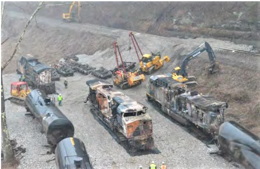
The earth slide that caused the derailment can be seen just to the left of the tank car in the upper right of the photo.
