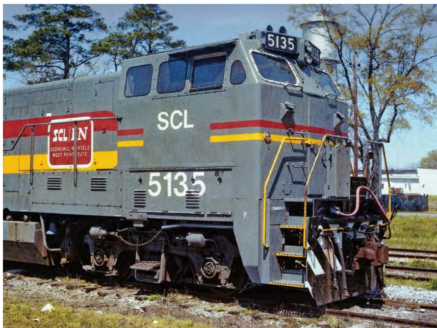
In this view of the cab of SCL 5135, the small windows on her cab front have been plated over but the small triangle windows at the cab's window line are still in place. (Warren Calloway photo)
