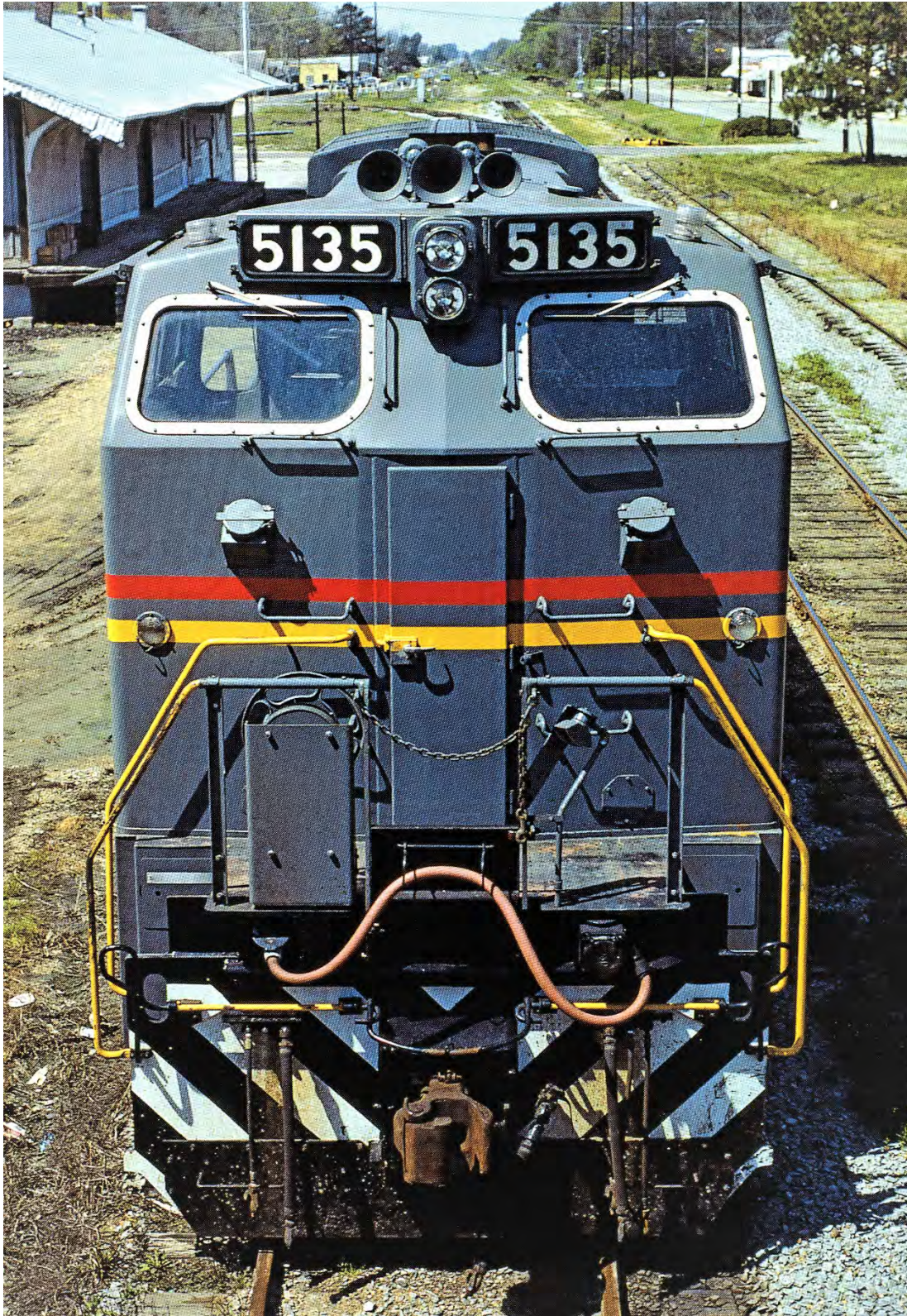
Head on view of SCL 5135 showing the engineer's lack of immediate downward visibility. The location of the plated-over small windows next to the door cannot be seen. (Warren Calloway photo)
