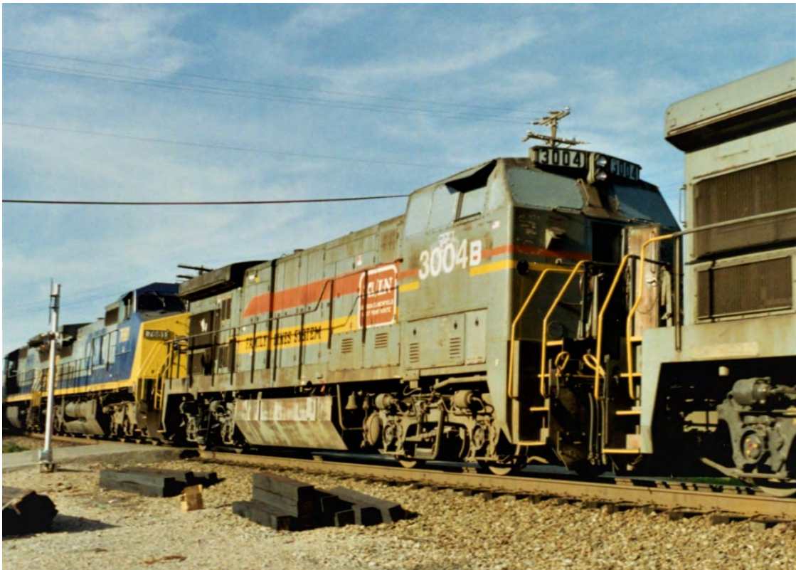
Above and below: Right-and left-hand side views of CSXT 3004B. There appears to be a difference in color. Note the “B” is in line with the reporting number 3004, and on the right side CSXT is stenciled above the road number. (CSXTHS photos)
