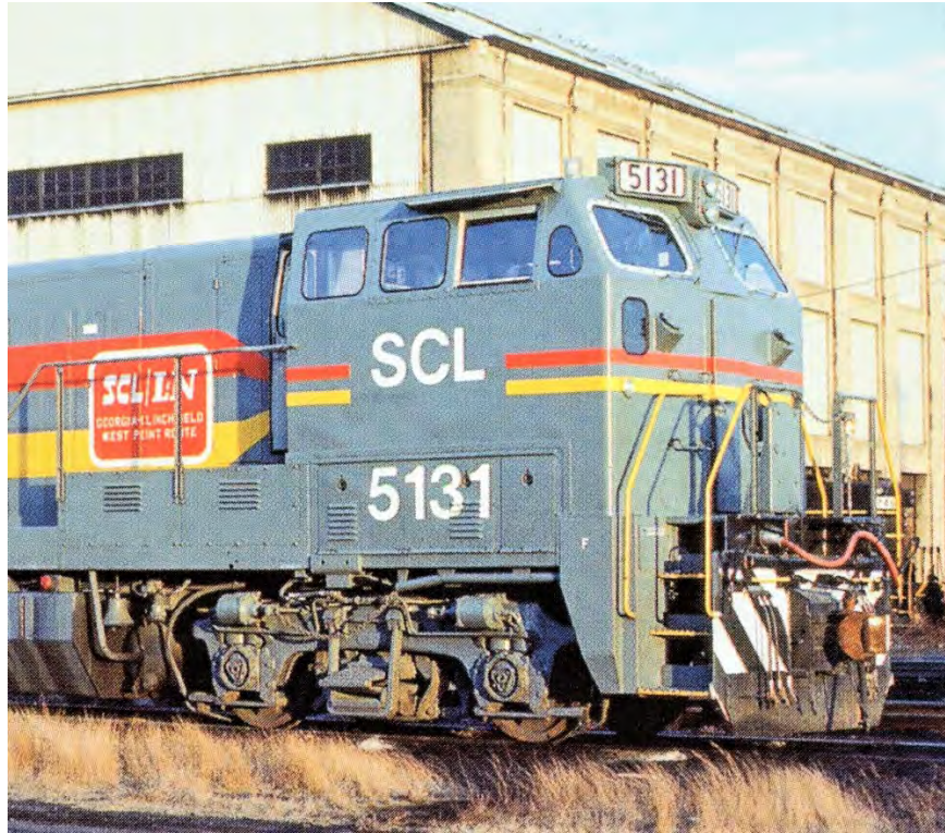
The cab of SCL 5131 as delivered in December 1994. The small triangle windows on the side of the locomotive at the cab's window line and the small windows on the front of the locomotive next to the door were plated over shortly after these locomotives went into service. (Warren Calloway photo)
