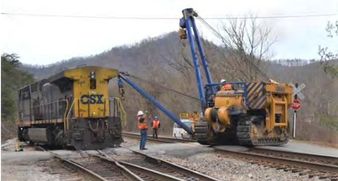
Donahue Brothers have arrived on the scene and are deploying one of their side lift tractors.
