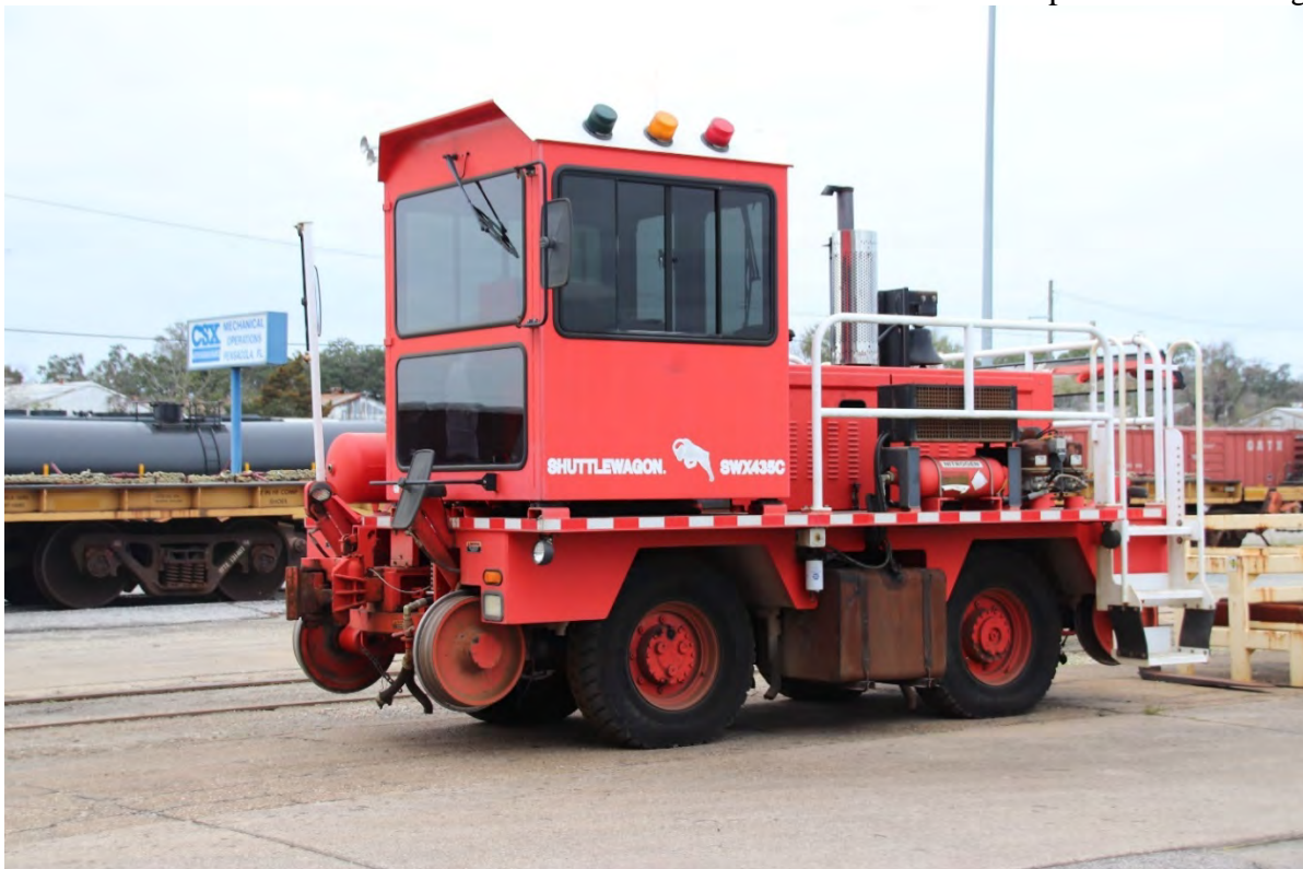
A close-up of the Pensacola Terminal Mechanical Operations' Trackmobile
