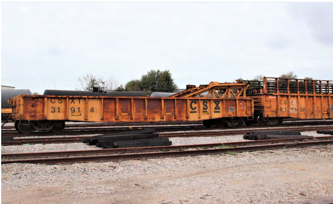
Tie gondolas, CSXT 31914 and CSXT 914508, in their CSXT Maintenance-of-Way orange, are flanked by stacks of new ties sitting on the ground waiting to be inserted under a rehabilitated yard track.
