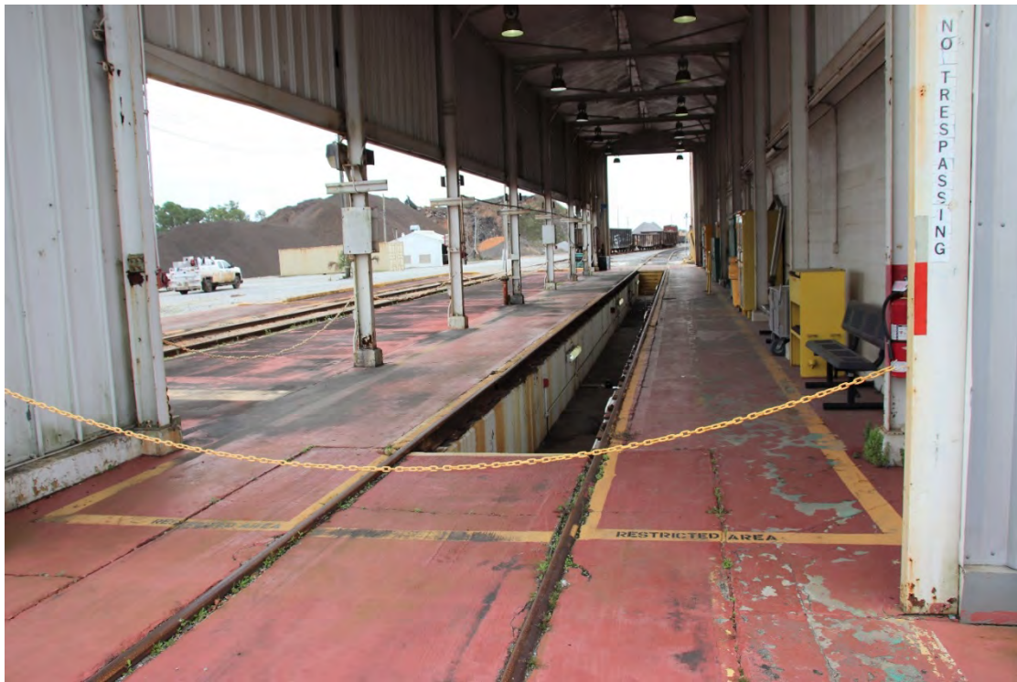
The work pit for inspecting and working on the underframe of cars
