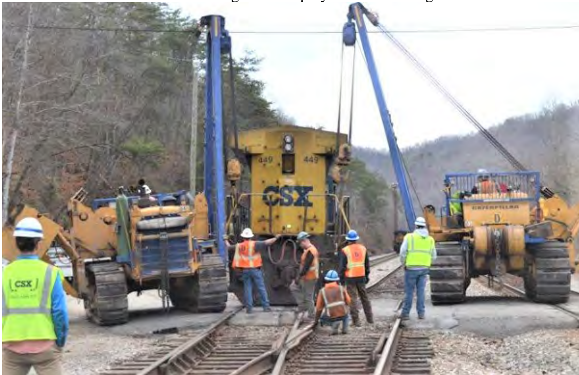
CSXT 449, suspended in the air by the booms of the sidewinders, is being gently nudged to the left to align her wheels with the rails.
