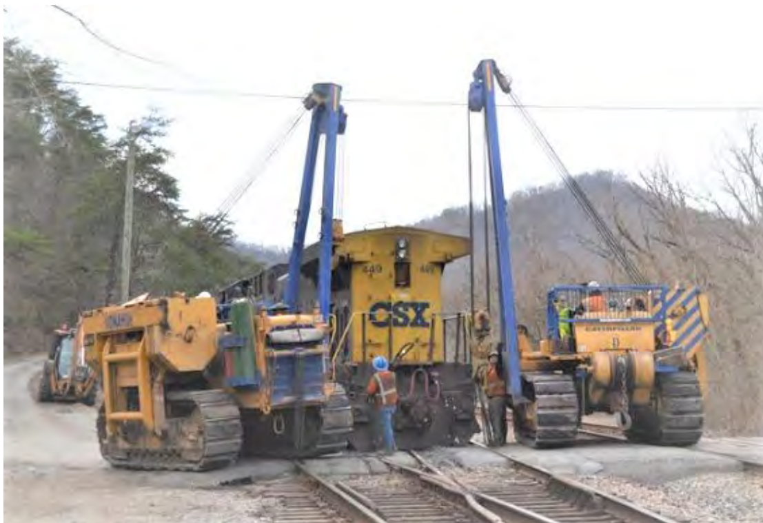
Both of the side lift tractors are hooking their booms to the frame of CSXT 449.
