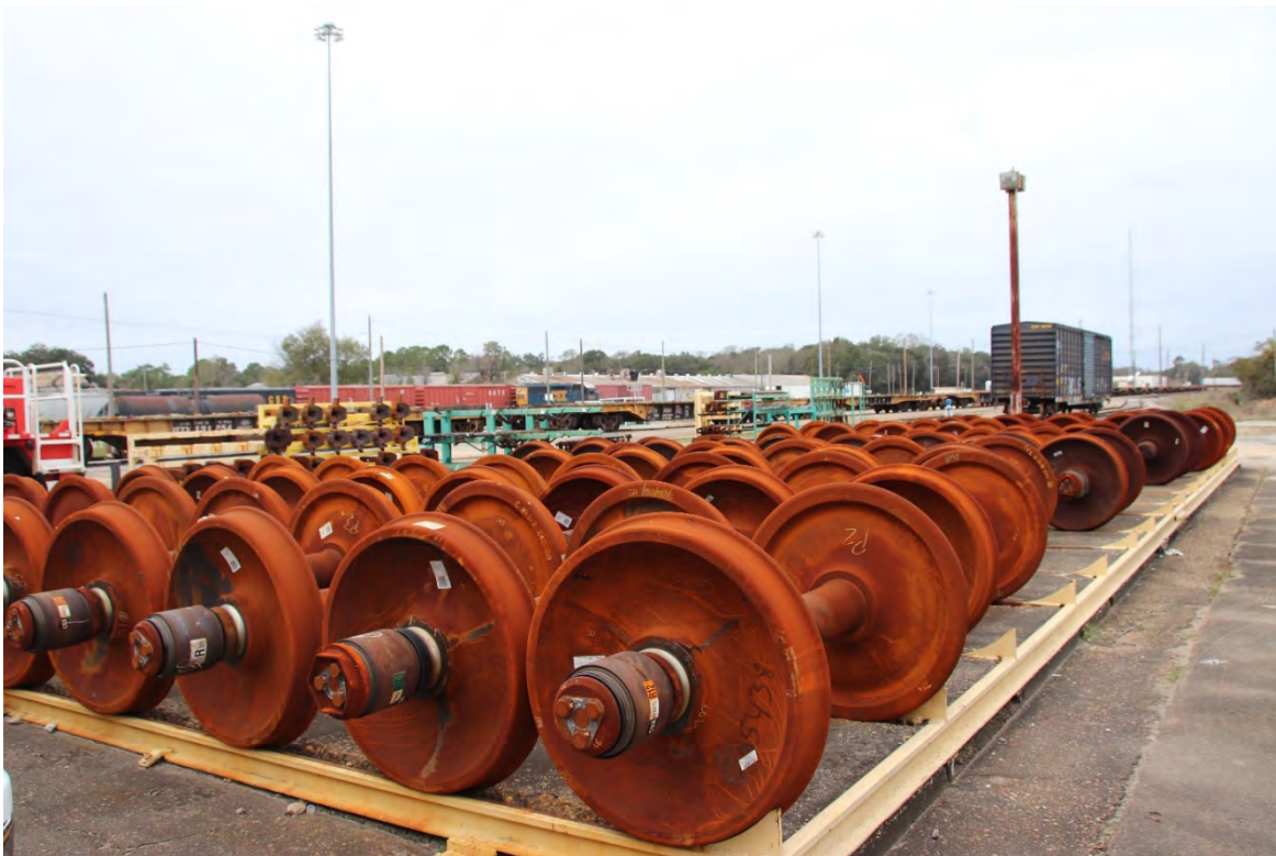
Wheels of every size sit outside of the Pensacola Terminal Mechanical Operations Building waiting to be used to replace a damaged set.
