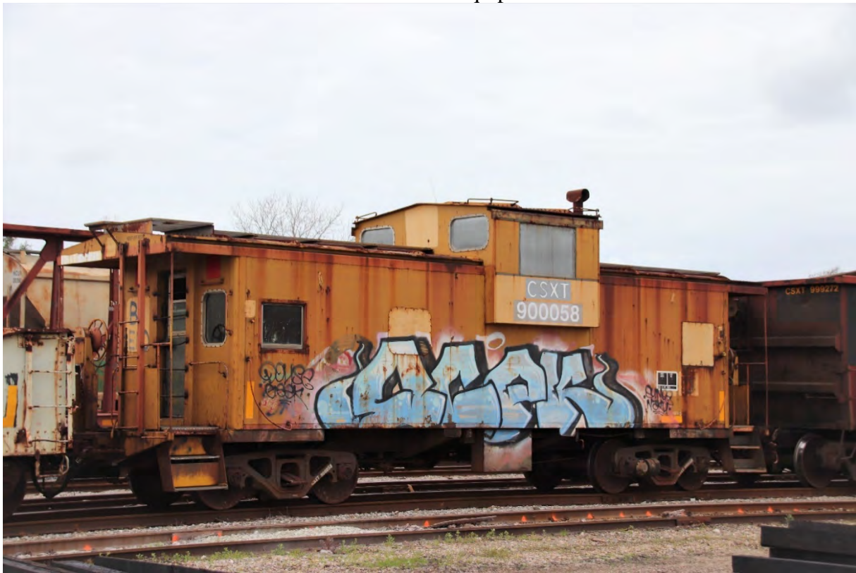
CSXT 900058 may look like a caboose but it is a shoving platform used in local switching service.
