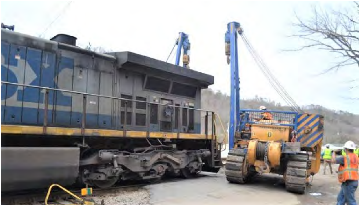
CSXT 449 is once again sitting on the rail and Donahue Brothers have un-hooked from the locomotive and are preparing to reload their equipment for the journey back to Barboursville.
