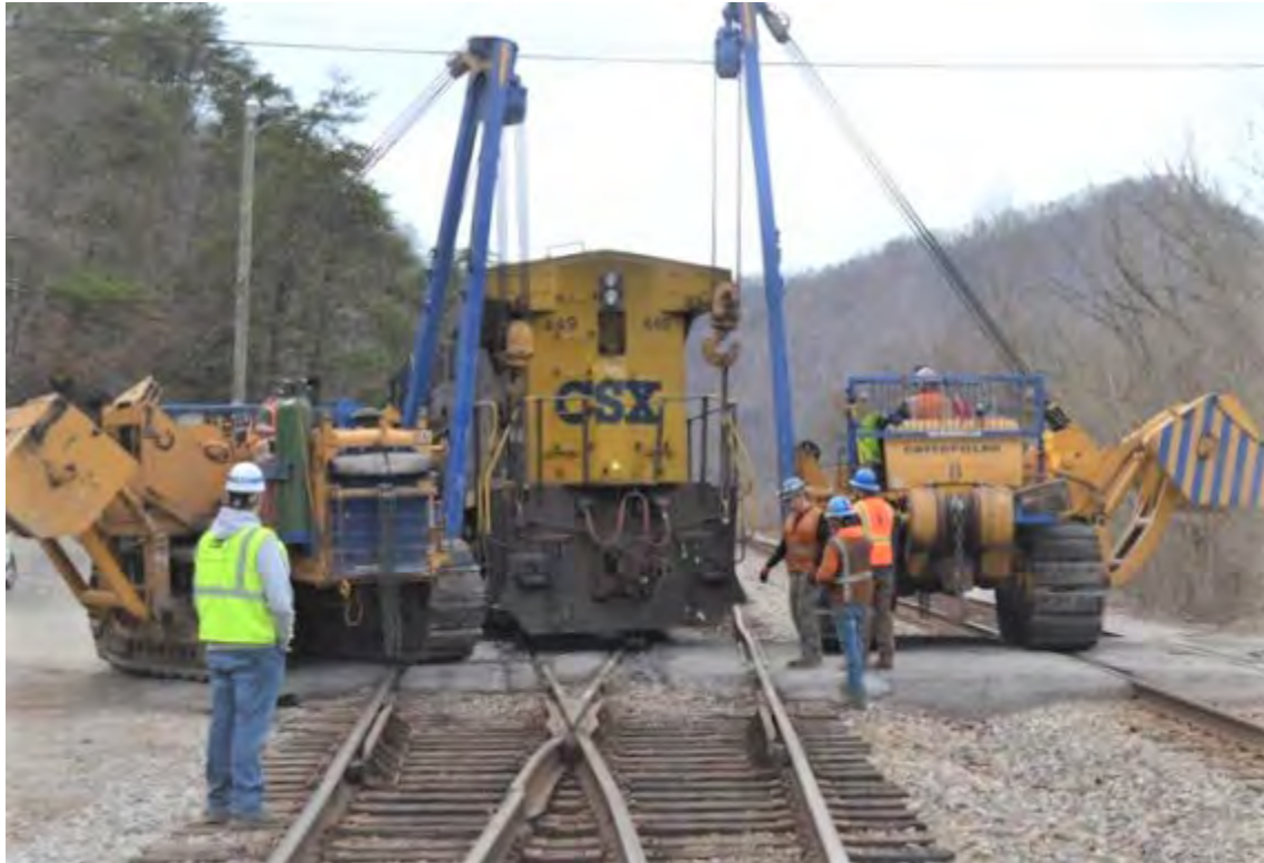
The counter weights are deployed as the lift begins.
