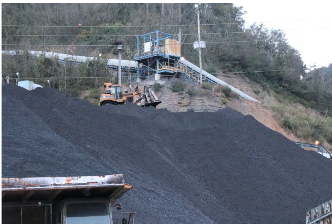
A close-up of the coal stockpile. A dozer is shaping the coal stockpile to ensure even flow of the coal into the tunnel containing the screw that feeds the coal tipples conveyor belt.
