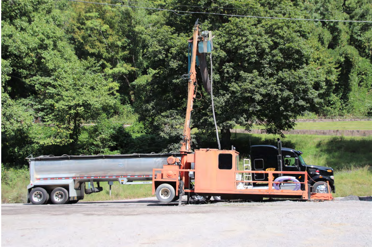
A side view of the coal sampling machine
