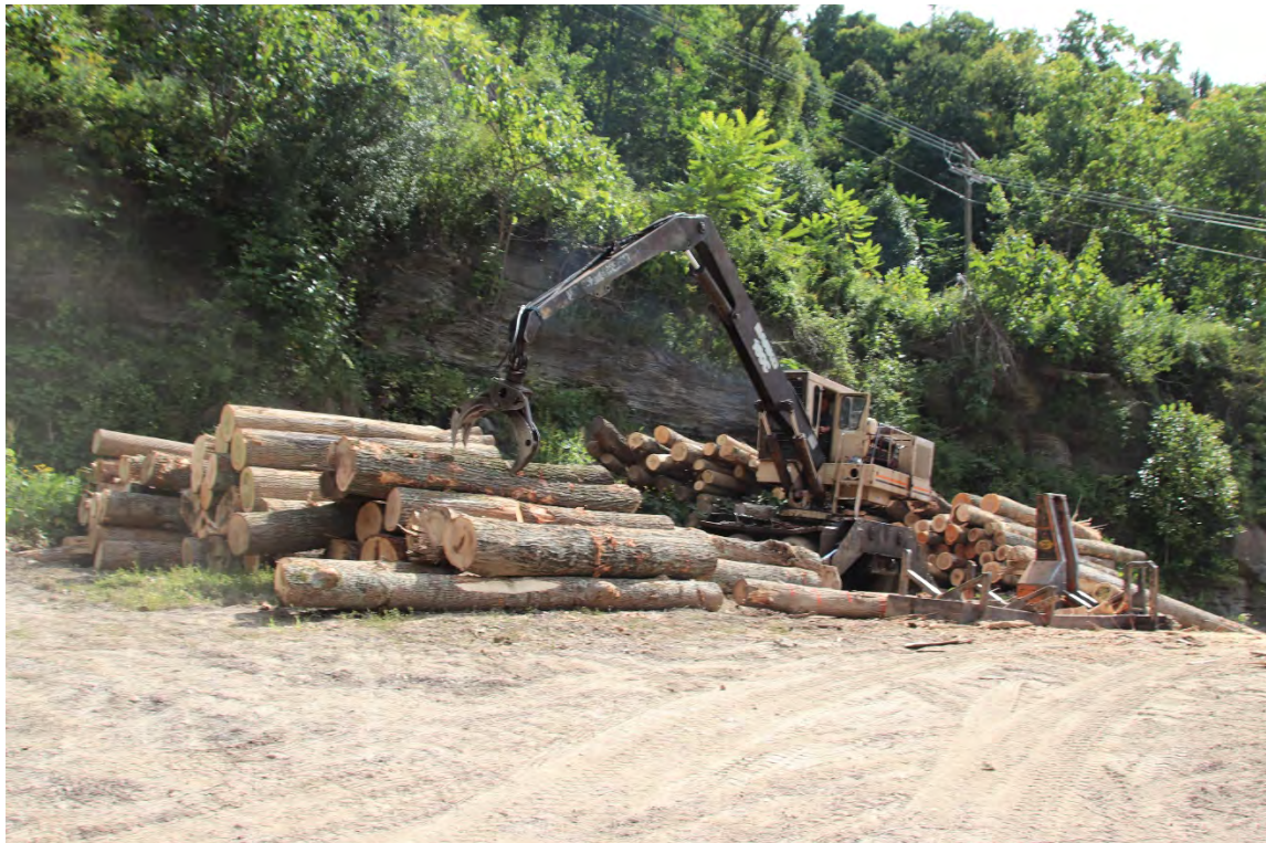
The log picker is arranging the logs in stacks for loading upon a log truck. Depending on the type of tree harvested, the logs will be taken to any one of six lumber yards in a three-county area. Note that none of these logs have their centers hollowed out by rot. All of these logs came from managed second or third generation growth.
