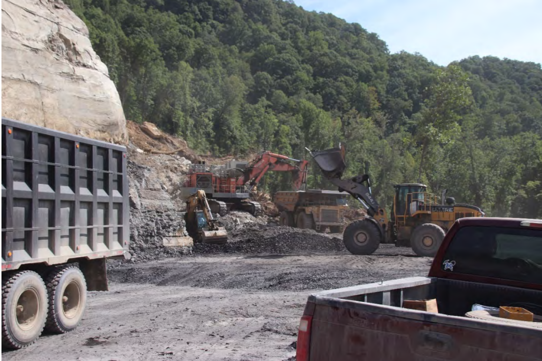
Coal being mined at the highwall. Trucks carry the coal from here to a conveyor belt that then carries the coal to the coal stockpile next to the coal tipple.
