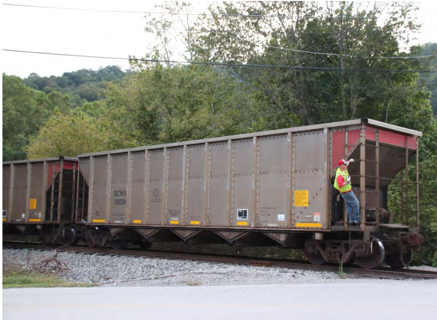
The Conductor, while clinging to his perch on the rear of SCWX 09298, uses his right hand to work his radio. Via the radio, the Conductor provides guidance to the Engineer as the cut of hopper cars enter into the east leg of Lenarue Wye.
