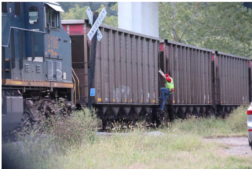
The Conductor is climbing onboard the lead coal hopper to set its hand brake.
