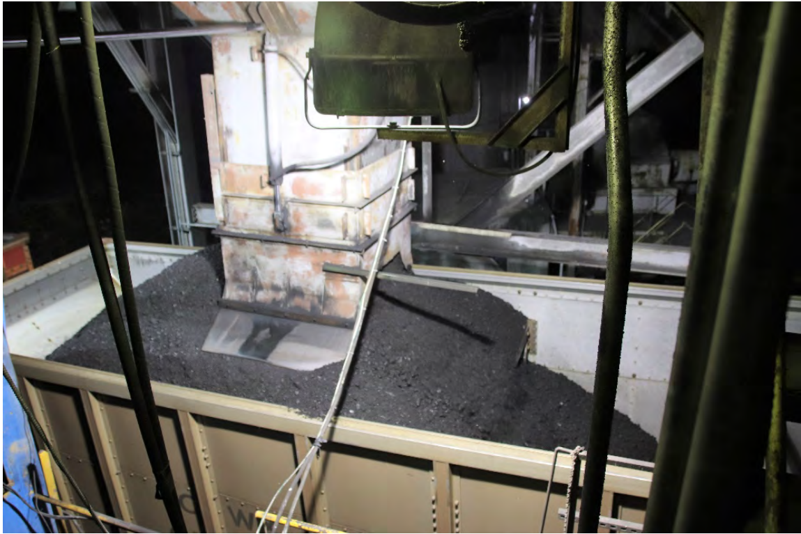
Above and below are views of the discharge chute loading a hopper car with coal. Note how the top of the coal is contoured to hold it within the car.
