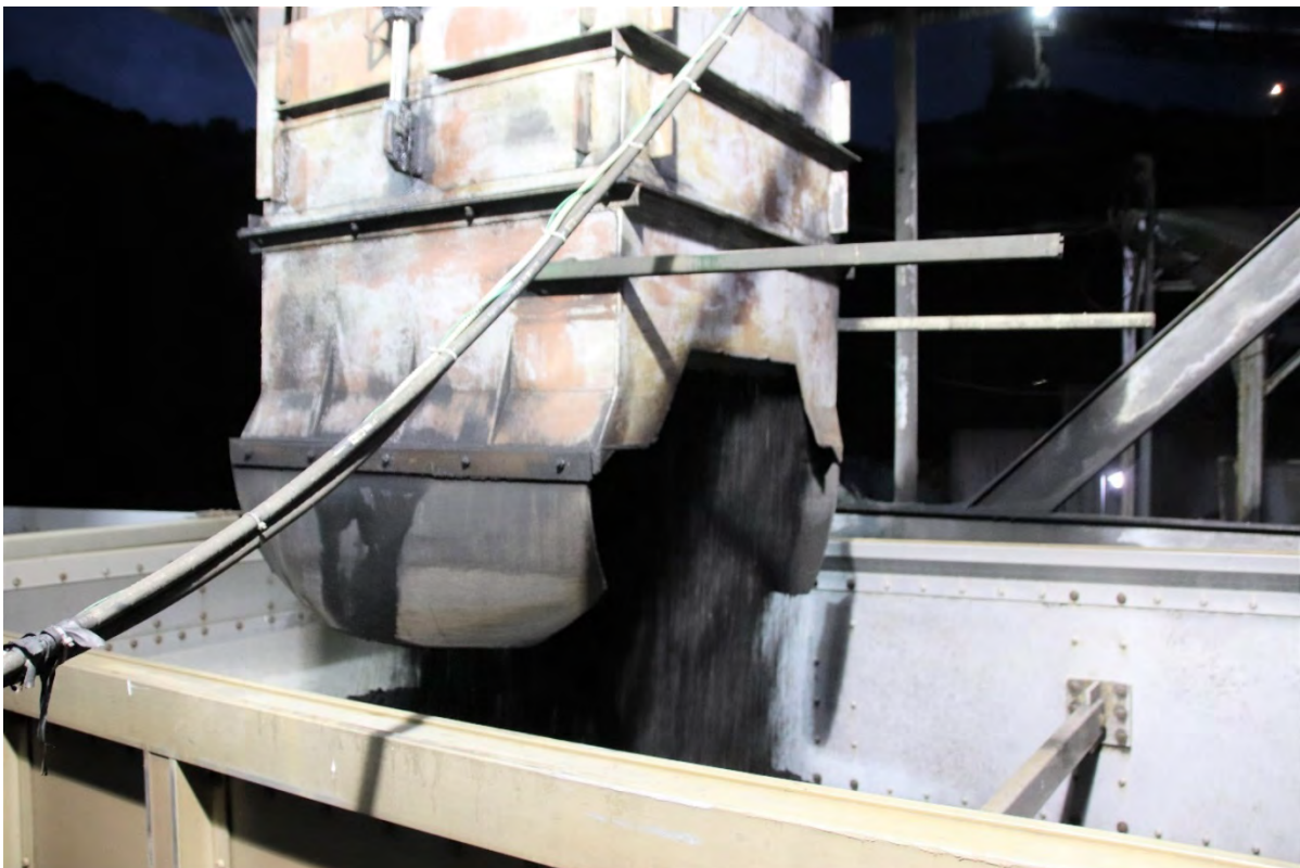
The first discharge of 117 tons of coal is coming out of one of the loading bins into the hopper car.
