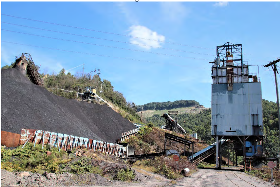
We have turned 180 degrees from the previous photo. The JRL coal stockpile is to the left and the JRL coal loading tippel, which will load CSXT's train C821, is on the right. The coal holding tippel can be seen through the legs of the loading tippel.
