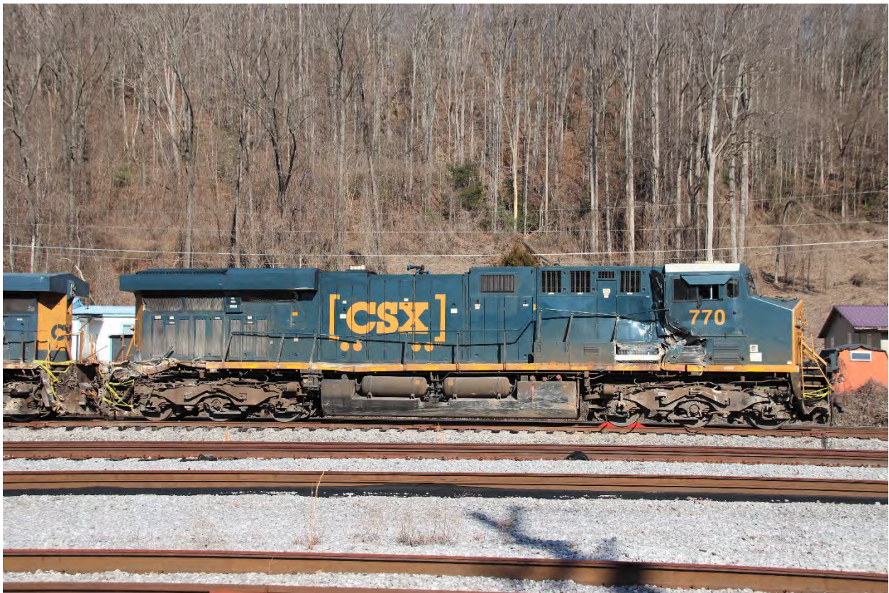
A view of the left side of CSXT 770. This is the side of the locomotive that hit the ground. Note the wheel chock under the third axle.
