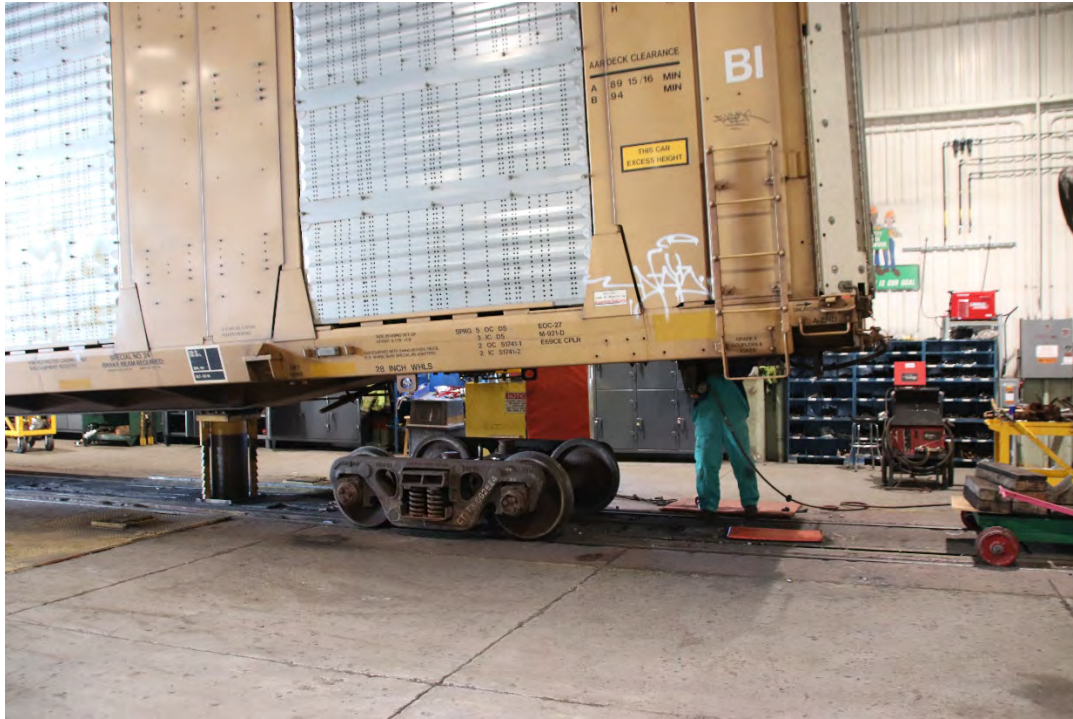
CTTX 692684 is being jacked up so the damaged truck can be pulled free.
