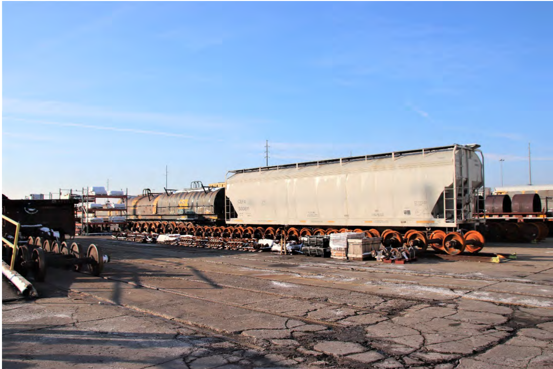
Two cars sit on the RIP track. Notice the various sizes of stored car wheels.
