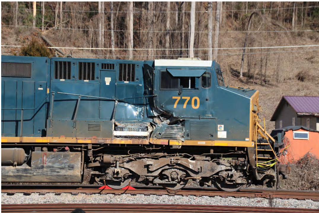
A view of the engineer's side of the cab of CSXT 770 showing the crushing force the locomotive experienced as she hit the ground.
