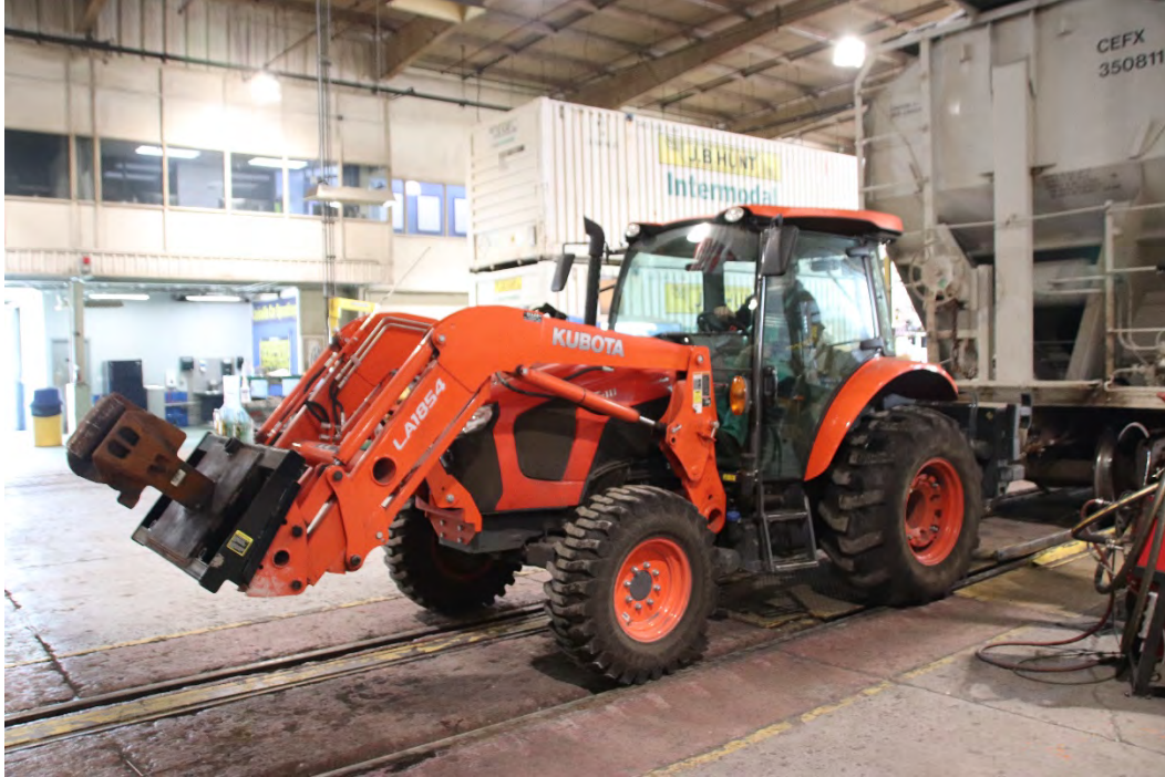
A close-up of the shop's tractor. Note the coupler on its front end; a similar coupler is located on the back of the tractor.
