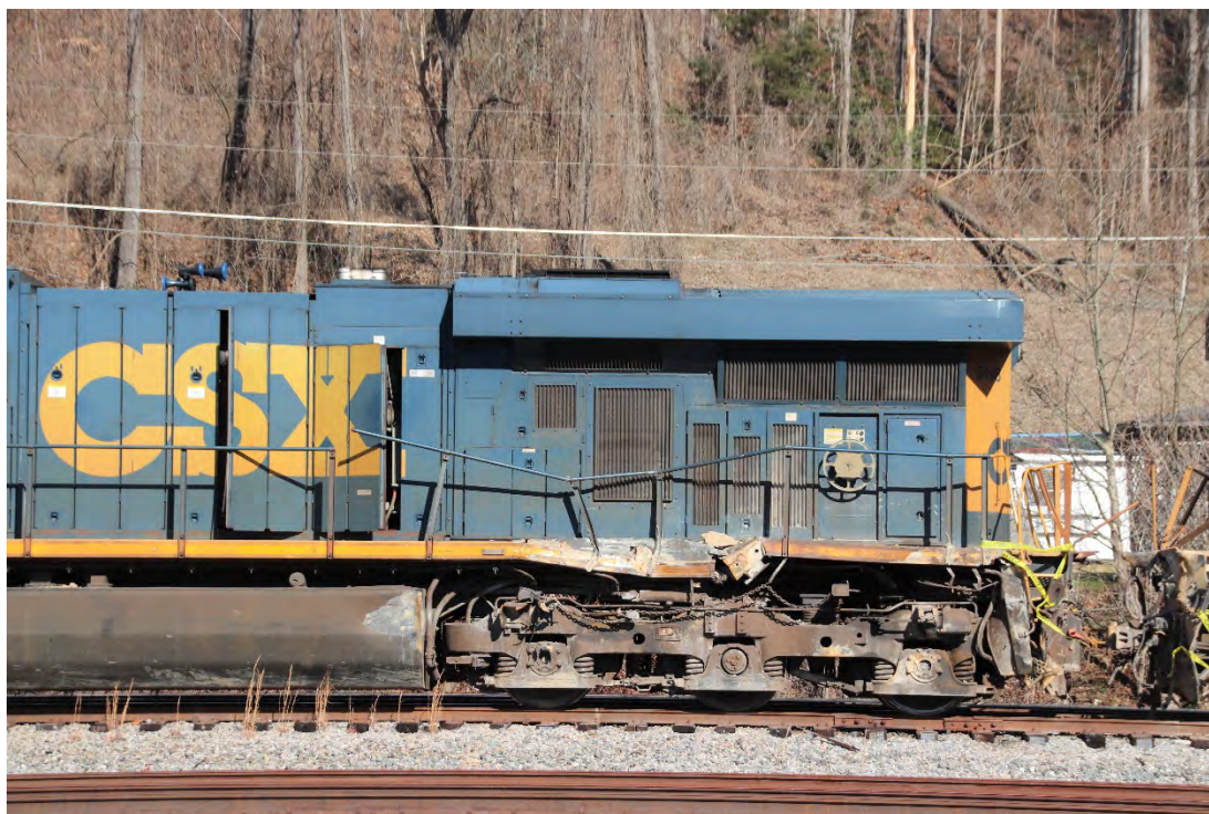
The right rear truck area of CSXT 5498 showing the damage to the locomotive's frame and truck.
