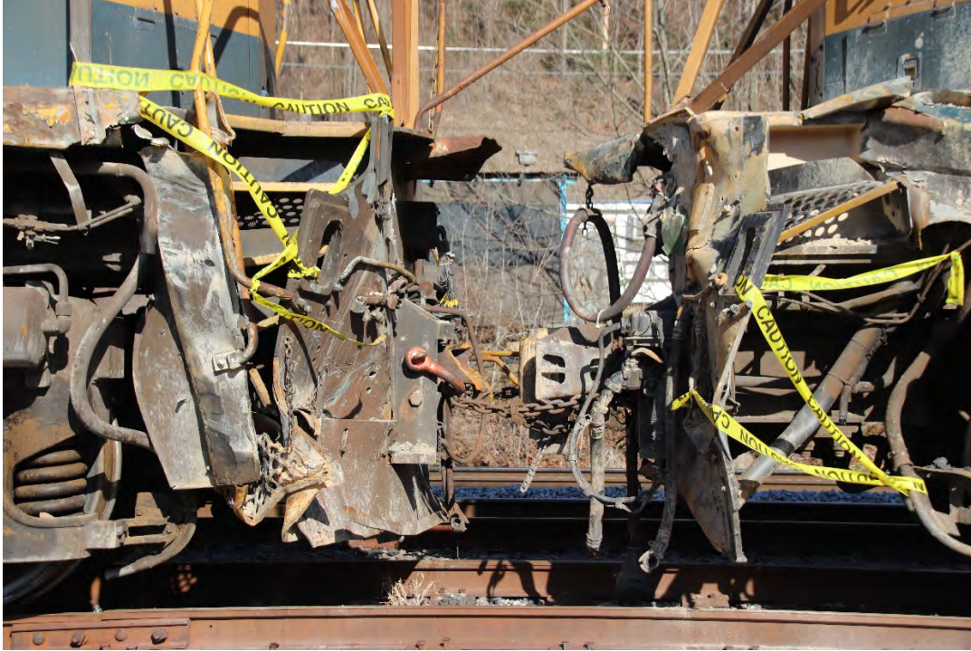
The field expedient chain lash up between CSXT 770 and CSXT 5498 that allowed both locomotives to be moved after re-railing from the accident scene to Loyall Yard.
