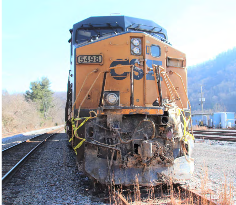
The nose of CSXT 5498 showing the damage it suffered in the derailment.
