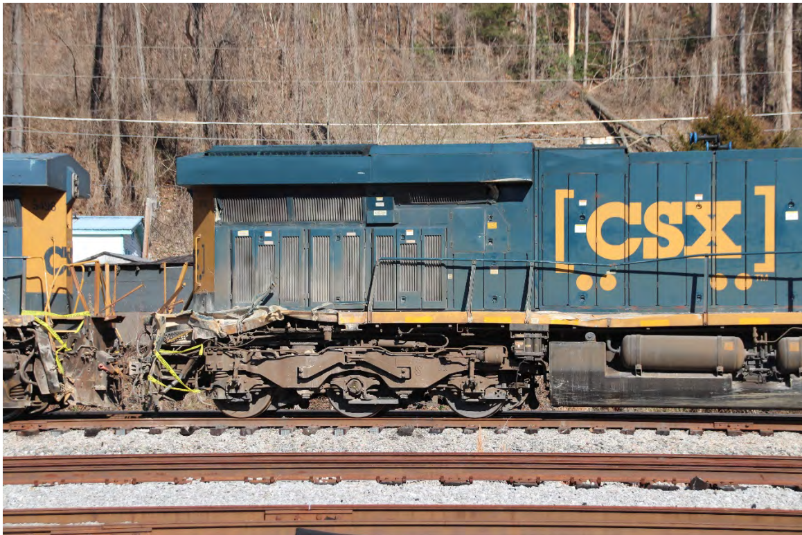
A view of the left rear truck of CSXT 770 showing the collision damage suffered from its coming into contact with CSXT 5498 as they both went on the ground.
