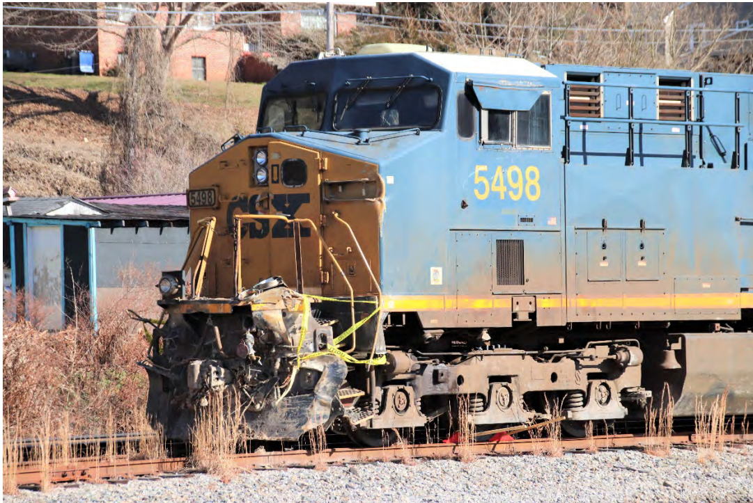
A view of the right side of the cab of CSXT 5498. The cab suffered little damage in the derailment.
