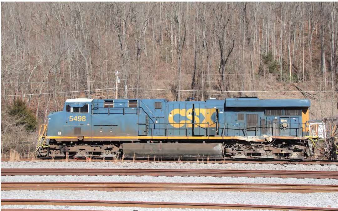
A view of the right side of CSXT 5498, which took the brunt of the force as the locomotive went on the ground.
