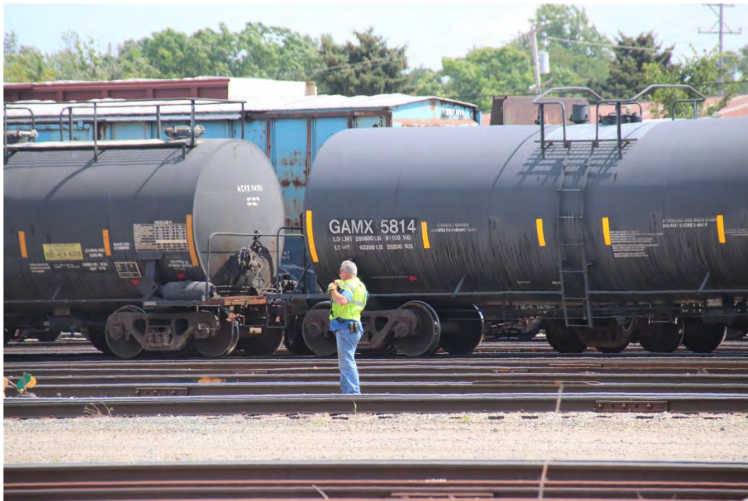
A remote-control locomotive operator, standing on the ground, works his engine as he makes up a train.
