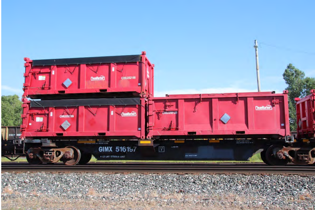
A close-up of three of the “Cleanharbors” hazard materials carrying containers. Note the placard holders have no markings on them.
