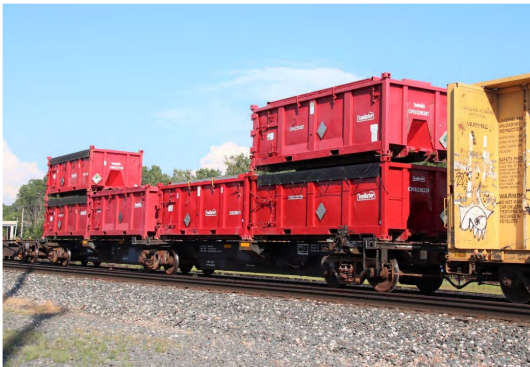
This GIMX 516197 spine car holds six “Cleanharbors” hazard materials carrying containers. These must be new containers as they carry no warning placards.
