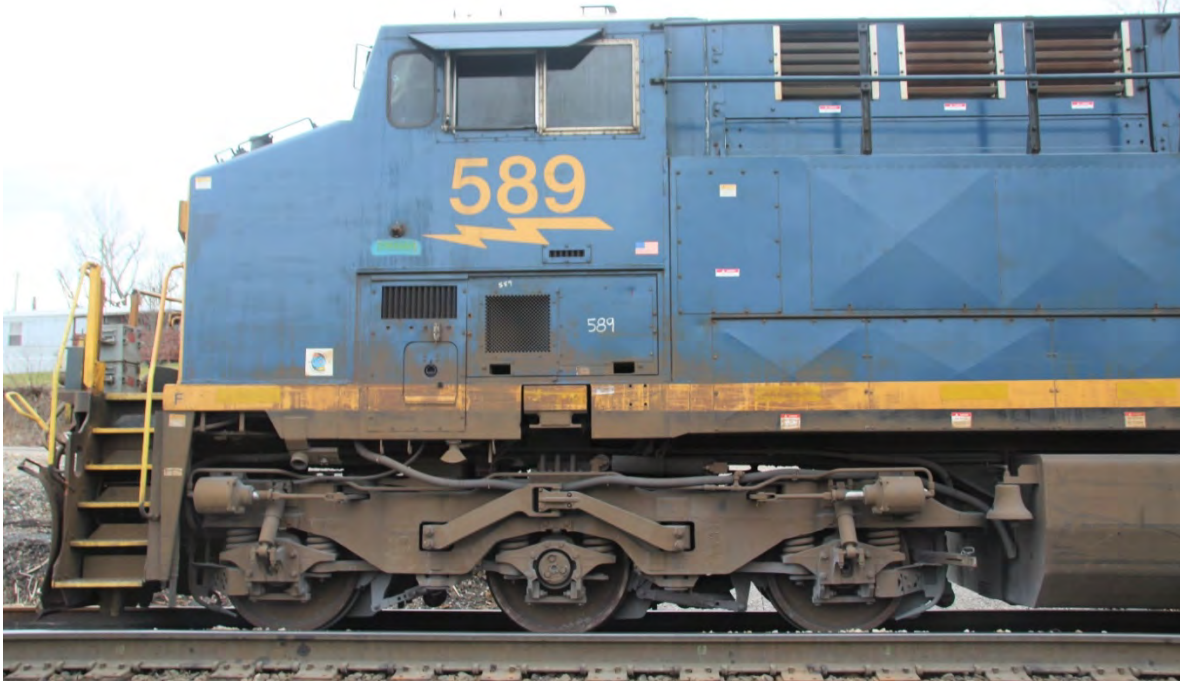
A close-up of the right side of CSXT 589. Note the bell in front of the fuel tank.
