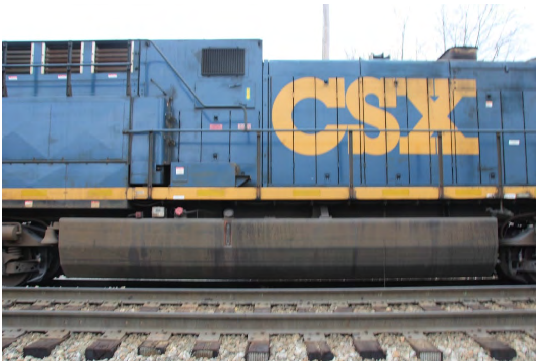
A view of the left center section of CSXT 589 showing the fuel tank and air reservoirs.
