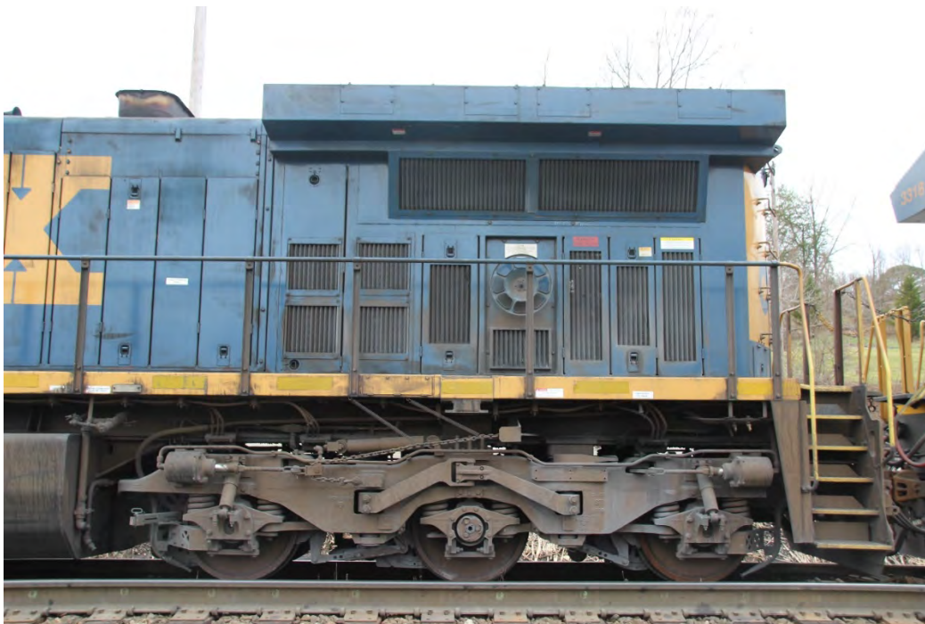
A view of the right rear truck of CSXT 589. Note the hand brake above the center axle.
