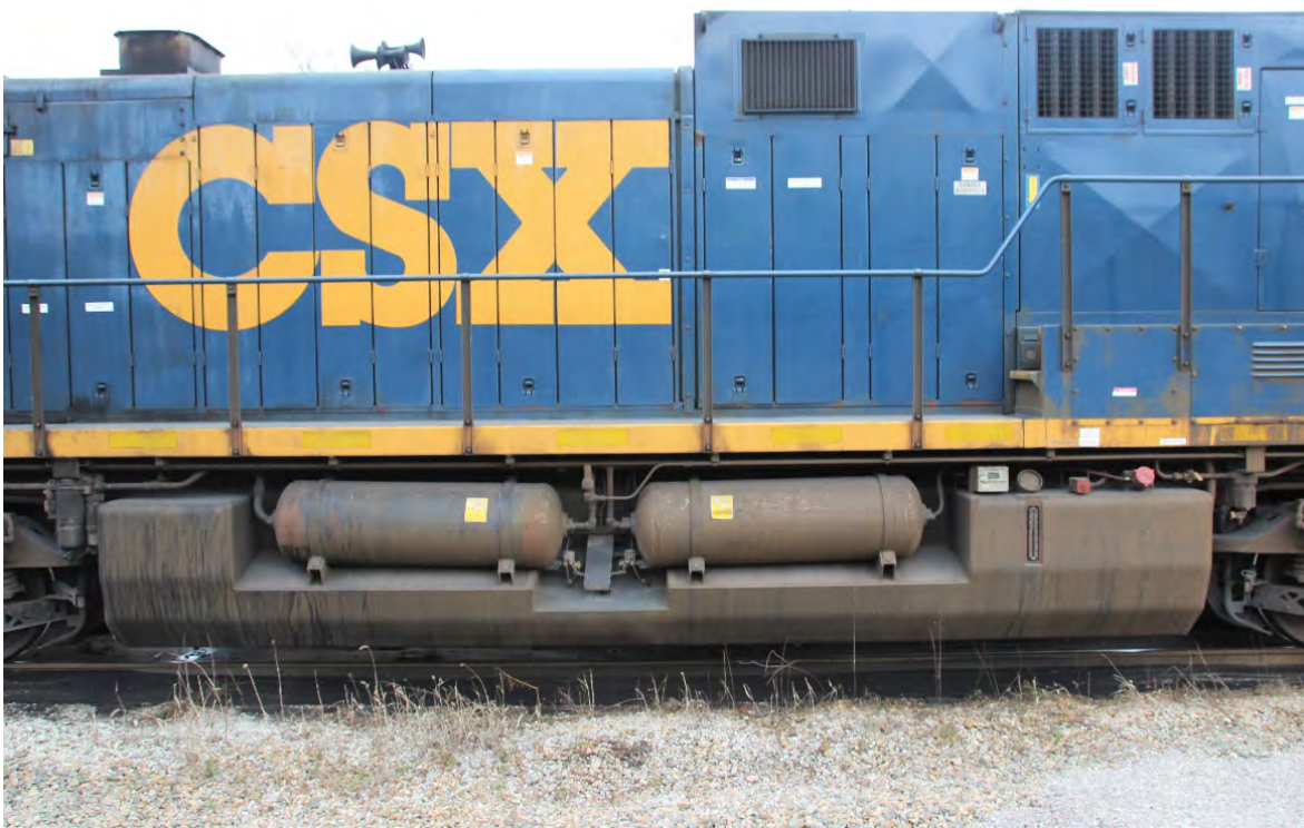
A view of the left mid-section of CSXT 589 showing the fuel tank and air reservoirs
