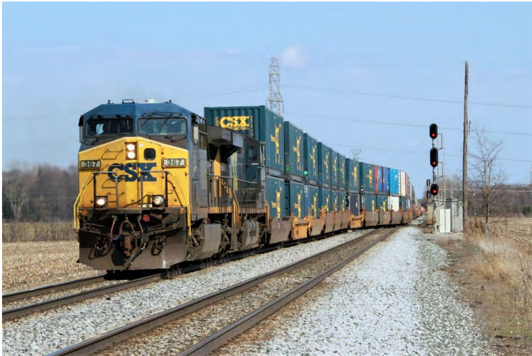
CSXT 367 leads a stack train via a crossover to the double mainline at Goodsend, Ohio. The first eight stacks hold all CSXT containers. Note the protecting signal is displaying red over red over red.
