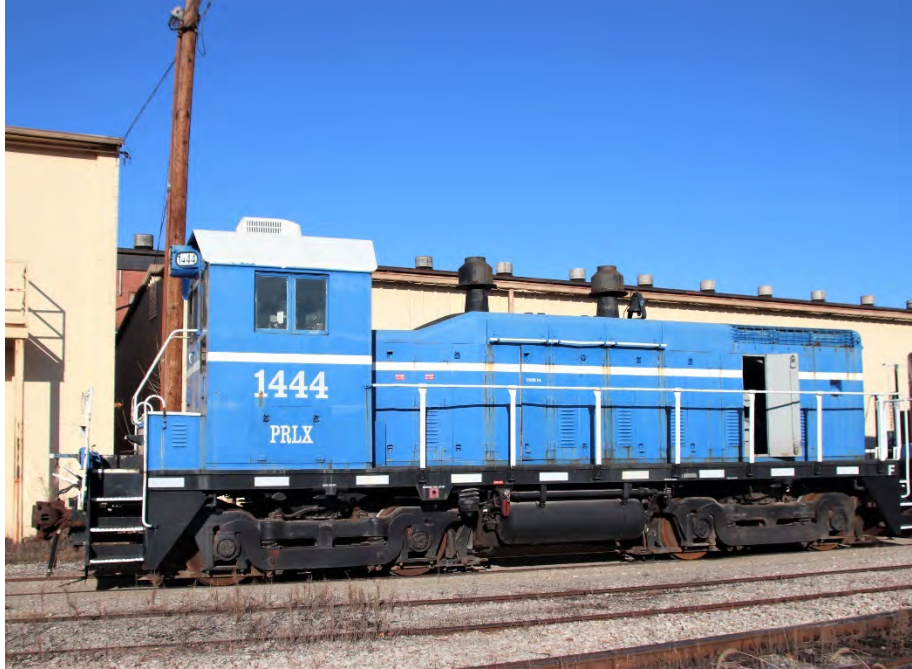
PRLX 1444 is an SW14 with a modified roof
