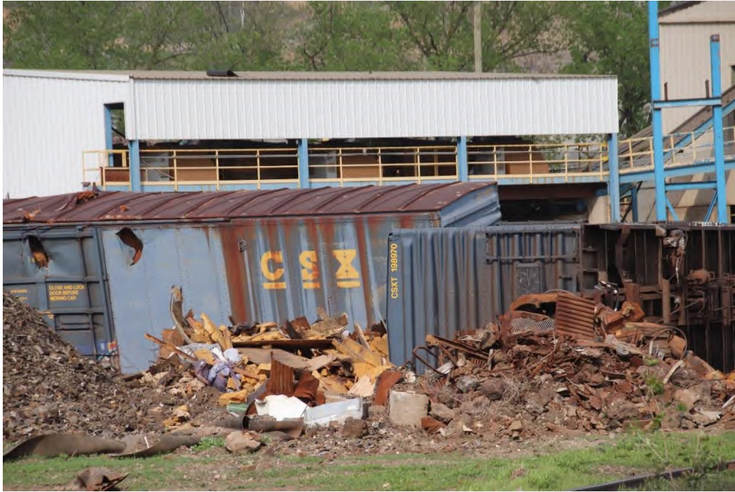
Two CSXT boxcars are in the process of being cut up.
