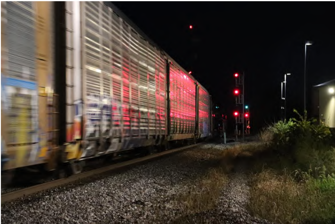
The near signal light is knocked down, RED over Red over Red. The distant light still shows Green over Red.
