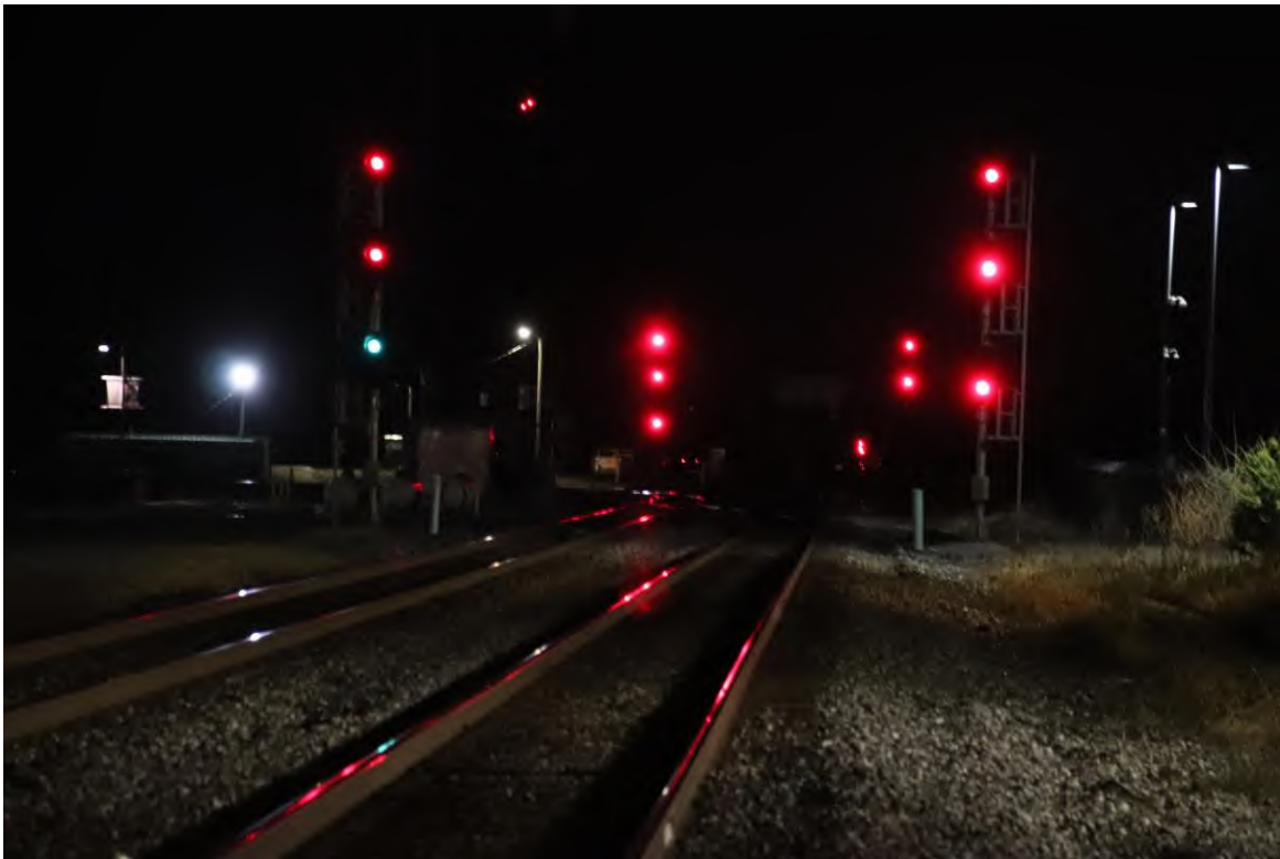
The signal lights for Track #1 now all show a Red aspect, however, the left signal, Track #2, still displays Red over Red over Green.
