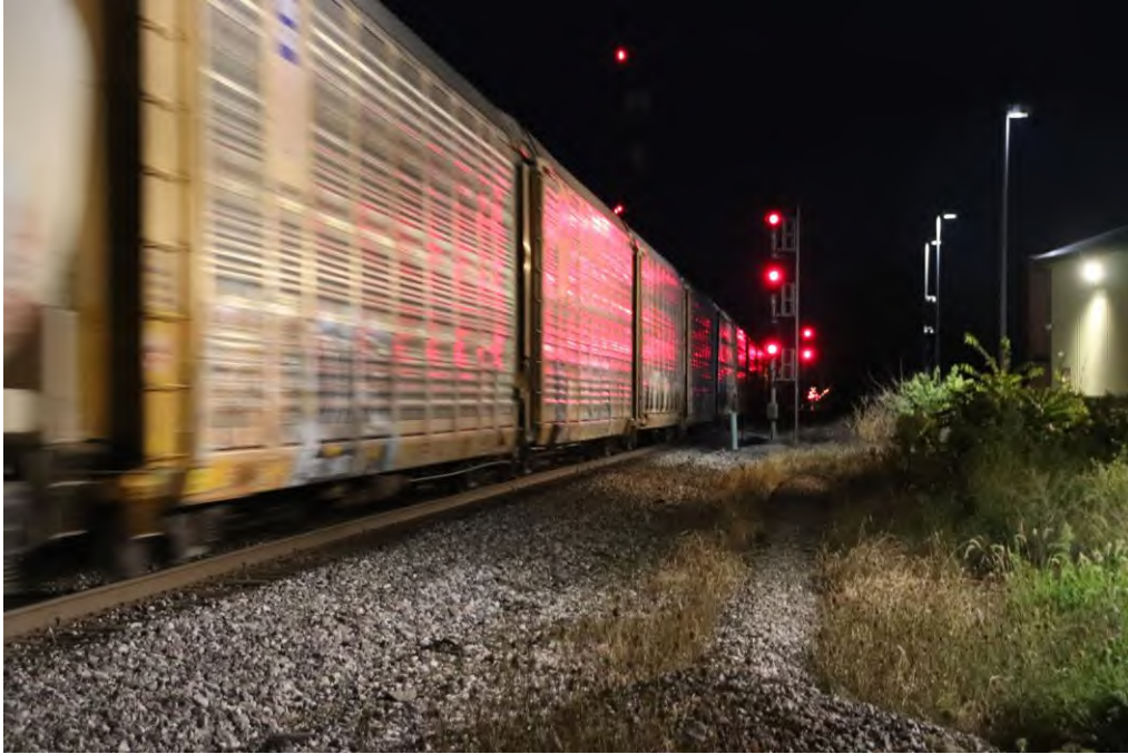
The distant signal light is knocked down and now reads Red over Red.
