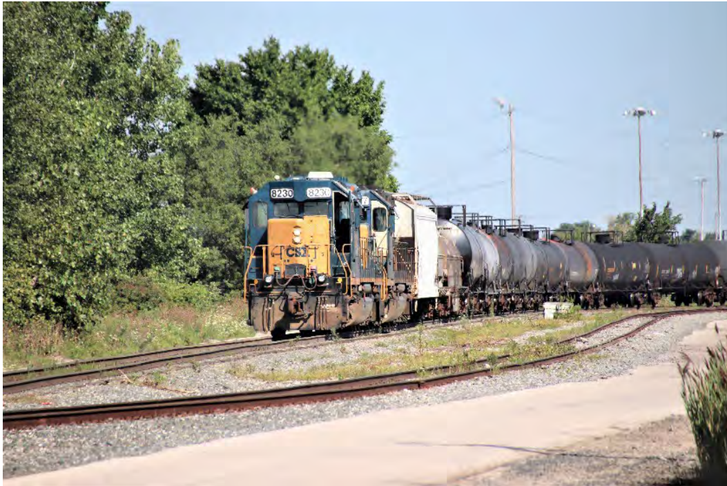
The train is moved from the bowl to the departure track where mainline power will be coupled to the train to take the cars to their next destination.
