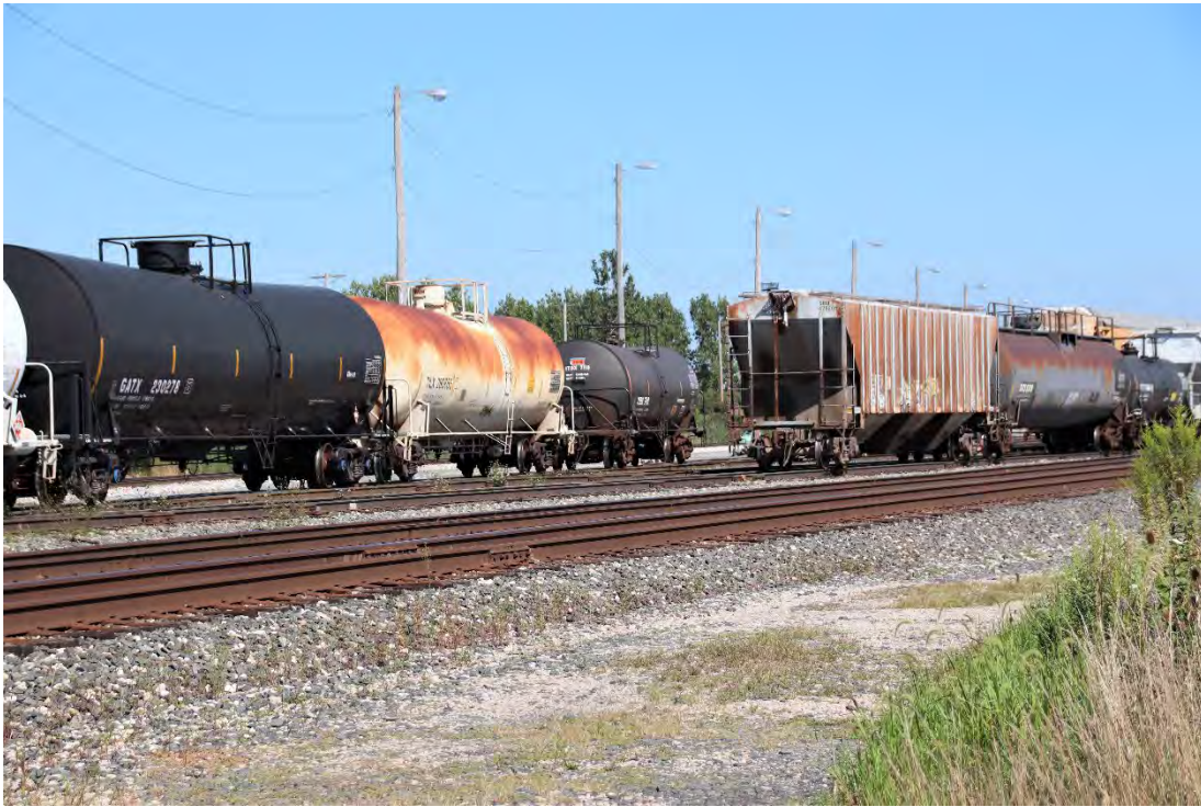
Above and below: The switching locomotives are brought to a quick stop and a tank car rolls free into the correct receiving track.
