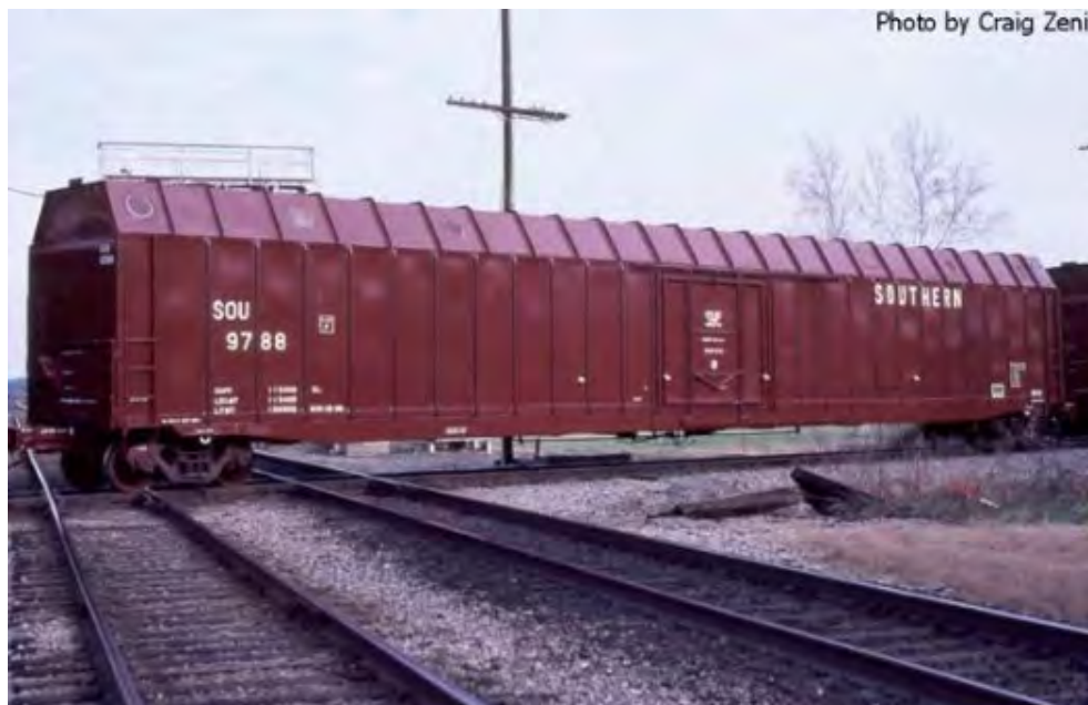
These oversize Southern Railway boxcars were used to move bailed tobacco from warehouses in Kentucky to the factory where cigarettes or cigars were produced. Note the rooftop round sky lights. These boxcars were at times in pool service and moved via CSXT in the 1980s and 1990s. (Craig Zeni)
