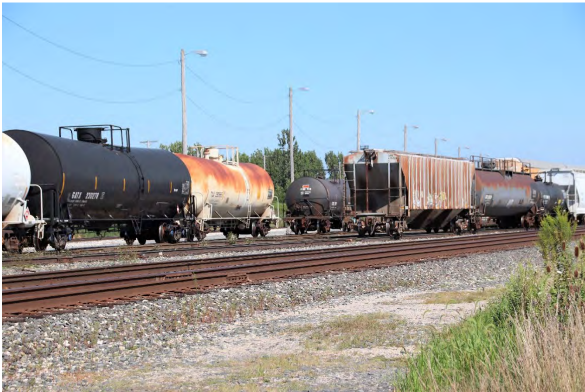
Above and below: The switching locomotives are brought to a quick stop and a tank car rolls free into the correct receiving track.
