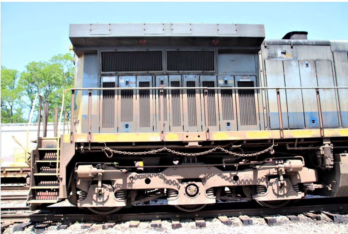
A view of CSXT 30's left side rear truck and its hood ventilation slots
