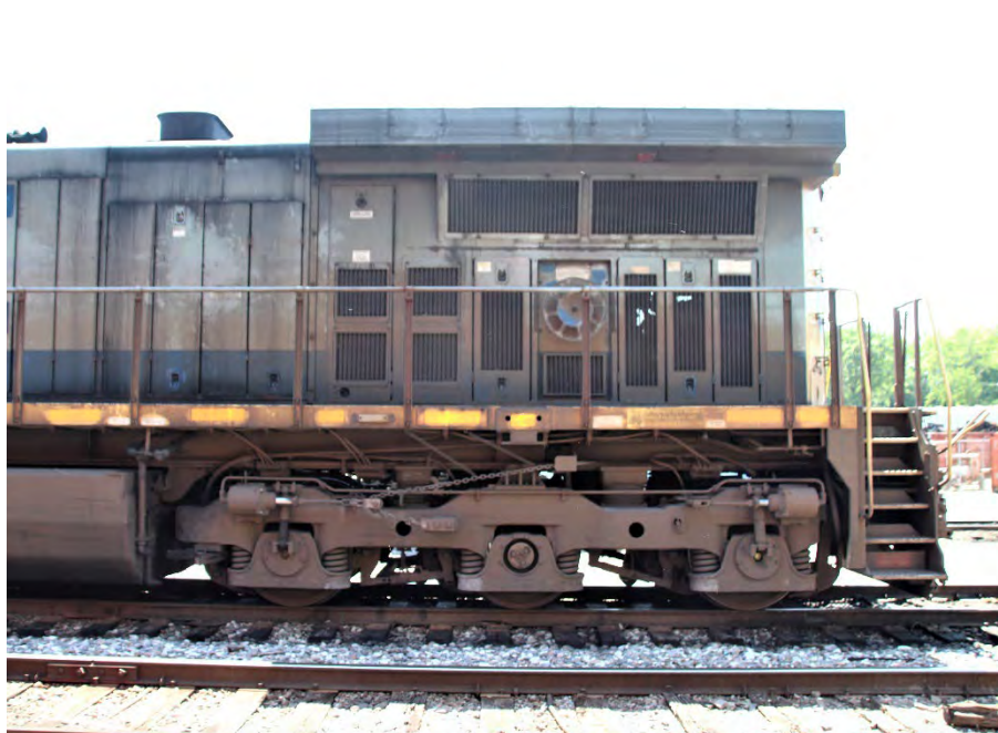
The right side of CSXT 30 shows axles 4, 5, and 6 and the overhanging radiator.
