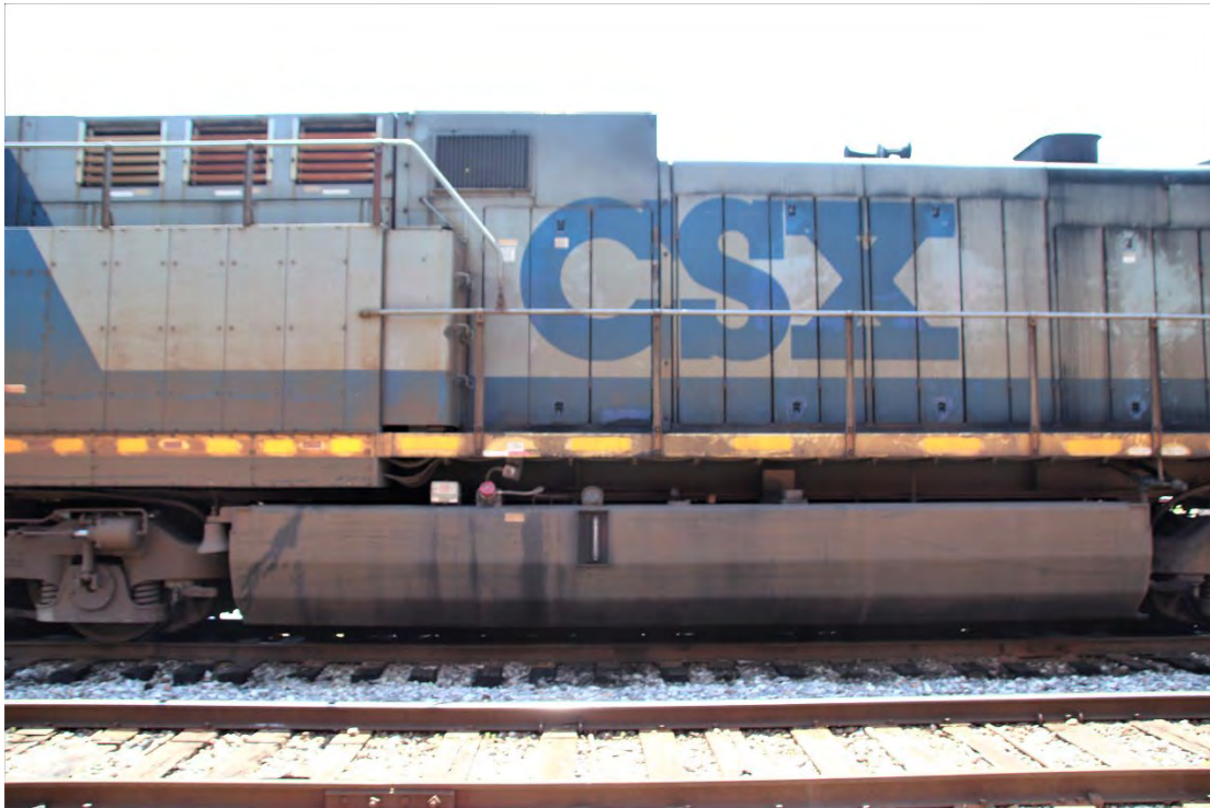
A view of the right side of CSXT 30 showing the fuel tank
