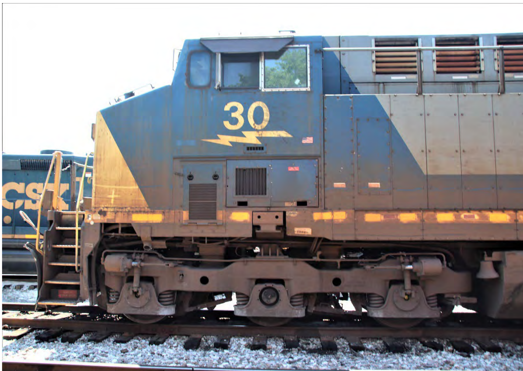
The right side of CSXT 30 shows Axles 1, 2, and 3, conductor cab window, and ventilation grills.
