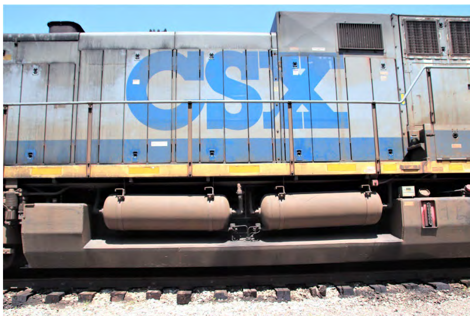
Left side mid body of CSXT 30 showing the air reservoirs tucked into the shell of the main fuel tank.
