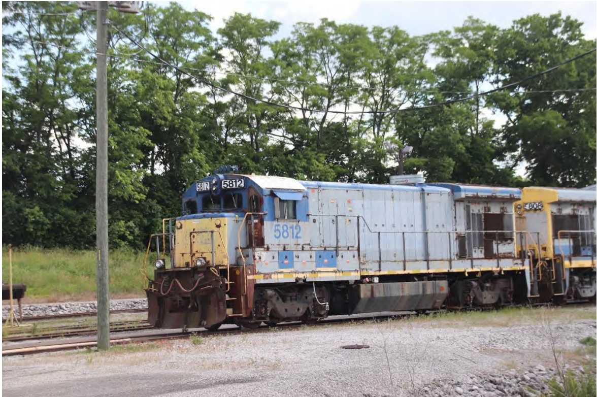
Above and below: TTI 5812 and TTI 5808, both GE B36-7 locomotives, were purchased from CSXT for use as a spare part source. Both are ex SBD.
