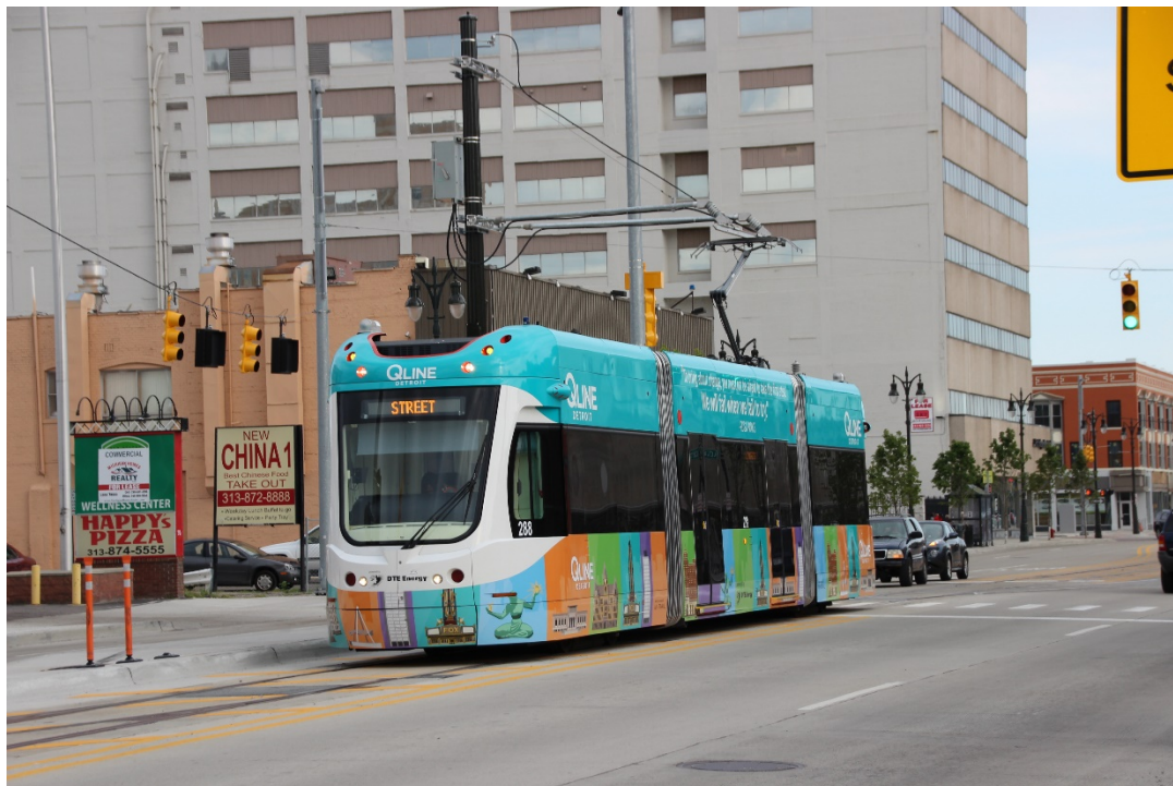
At the end of the line at Grand Avenue. The streetcar has its pantograph raised to pull electricity from the overhead plate to recharge its lithium-ion batteries.
