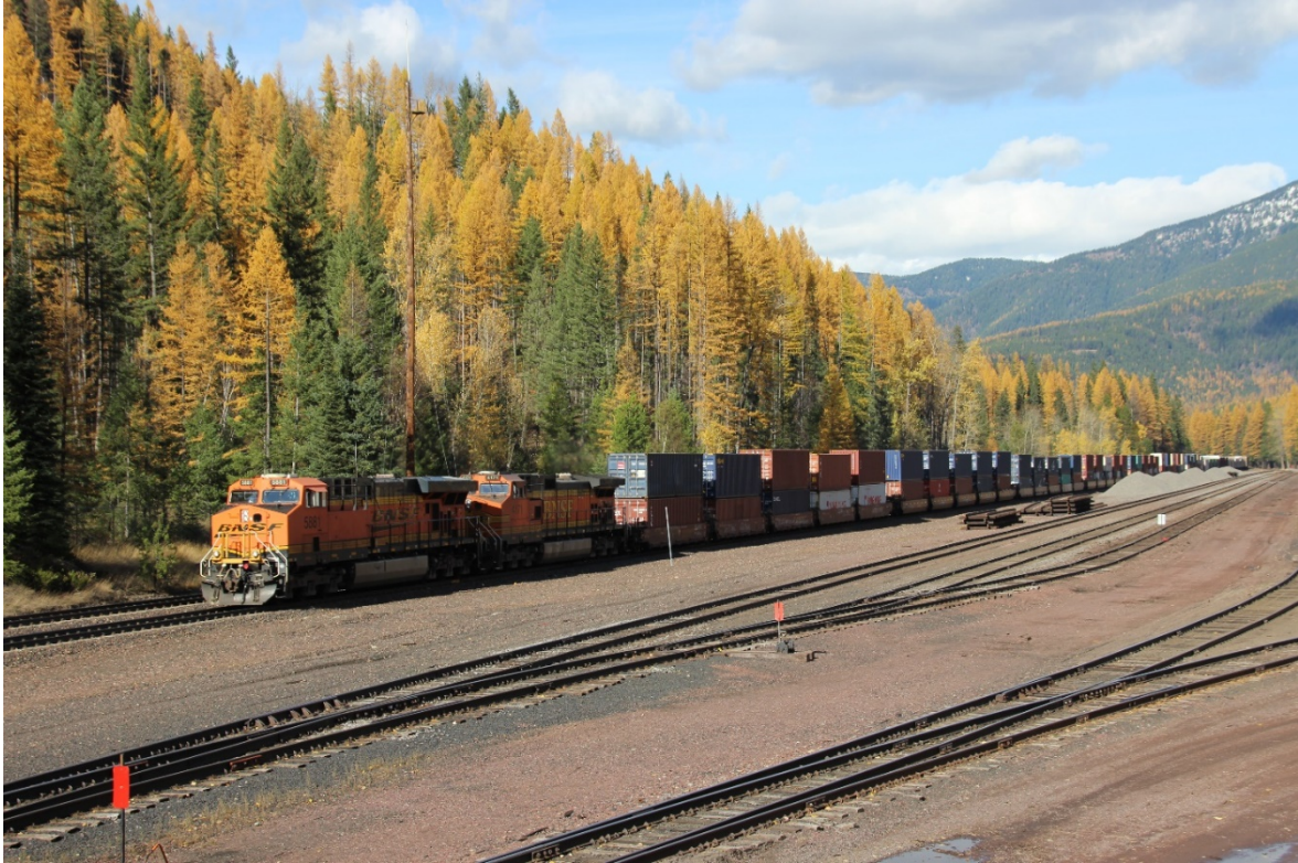
A stack train headed by BNSF 5881, a GE ES44AC, and BNSF 4171, a GE C44-9W, as seen in Essex Yard from the pedestrian bridge that connects Caboose Row with the Izaak Walton Inn.
