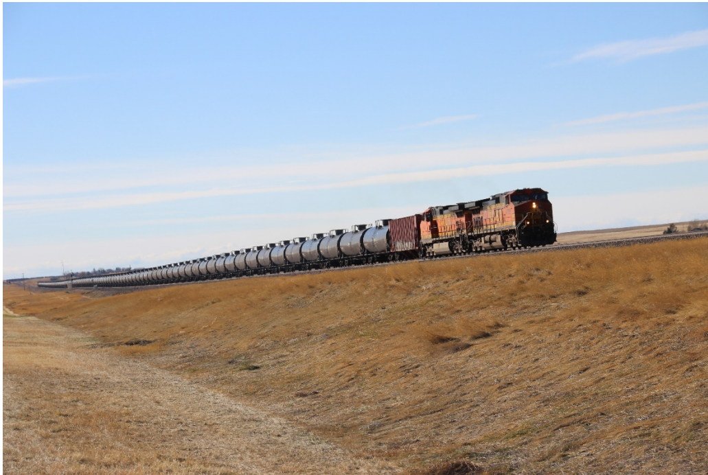
BNSF 4758 and BNSF 4056, both GE C44-9W, lead an oil train east from Culbertson, Montana. Note the spaced car between the locomotives and the tank cars. A spacer car was also located at the end of the train to separate the pusher locomotive from the tank cars. All spaced cars carried lettering showing they were in spacer car service and were not to be removed from the train without authorization.
