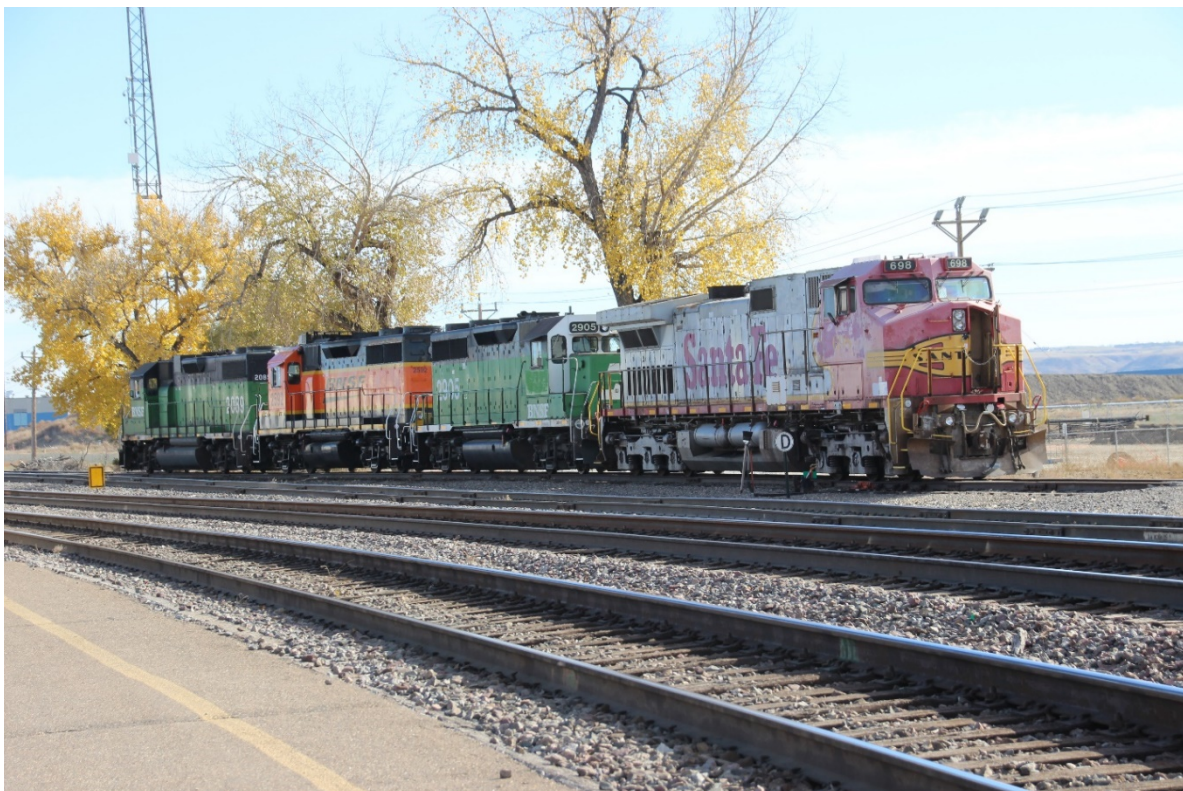
Above and below: Working the east end of the Williston Yard was BNSF 2725, a GM GP39-2, while parked in a pocket track were BNSF 698, a GE C44-9W; BNSF 2905, a GM GP39-2R; BNSF 2952, a GM GP39-2; and BNSF 2089, a GM GP38-2.
