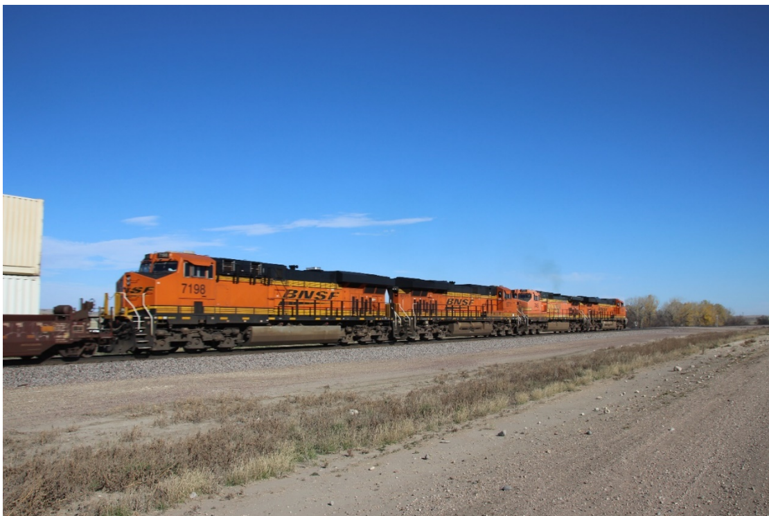
BNSF 7926, a GE ES44DC; BNSF 745, GE C44-9W; BNSF 6771, a GE ES44C4; and BNSF 7198, a GE ES44C4, head west from Williston with a stack train. Note the road in this photo and below that we were using to follow the railroad tracks.
